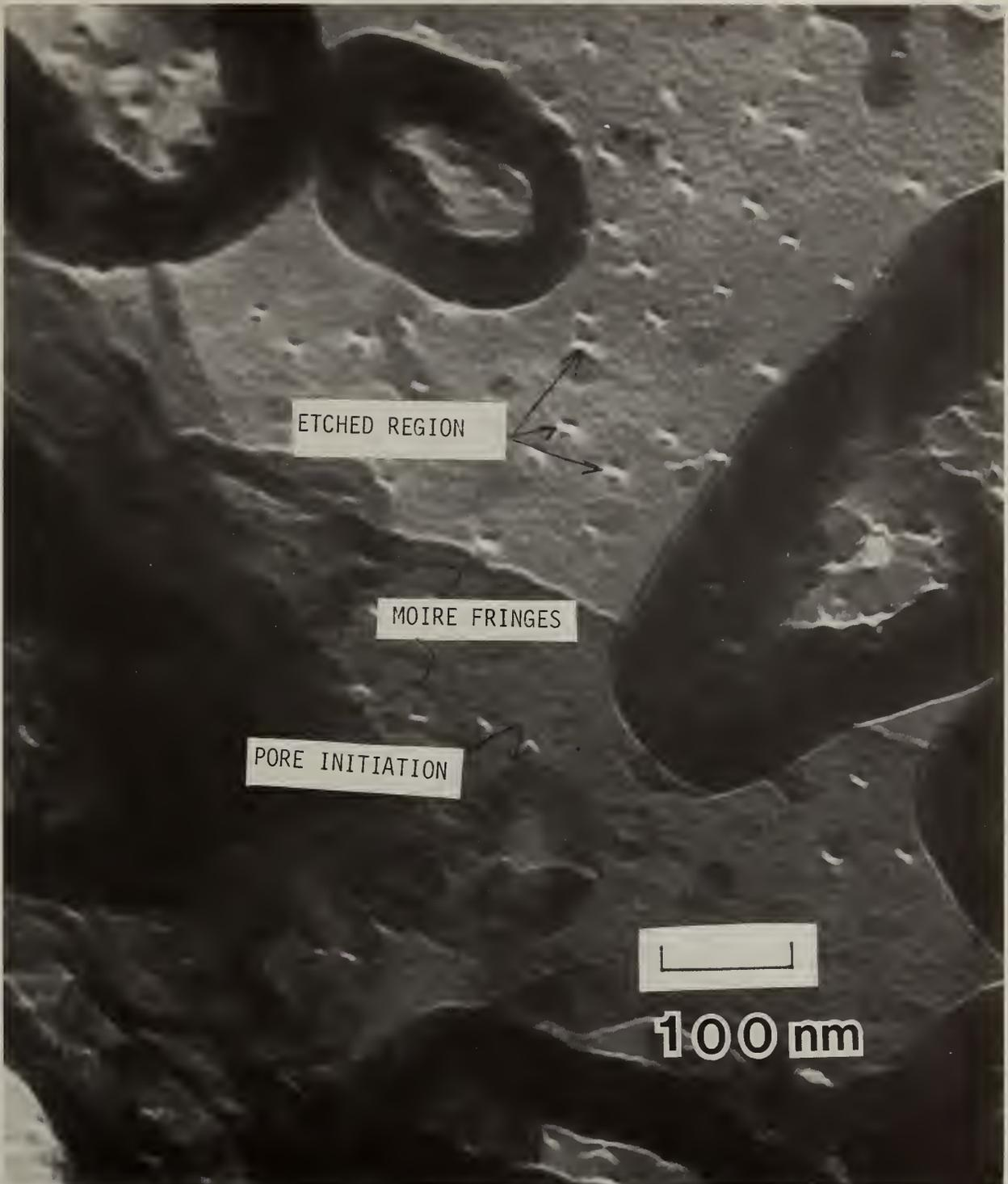
Figure 7. A TEM micrograph of the initial stages of anodic film formation on 7146 T6. The electron beam is now perpendicular to the interface. Note that the surface is covered with Moire fringes which may indicate an epitaxial oxide forms during the initial stages of anodization.
