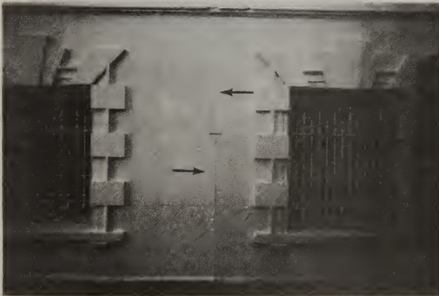
FIGURE 45. AREA D AFTER REPAINTING; ARROWS INDICATE VERTICAL LINE DIVIDING TEST SECTIONS D4 AND D1 (TO LEFT) FROM SECTIONS D2 AND D3 (TO RIGHT)
