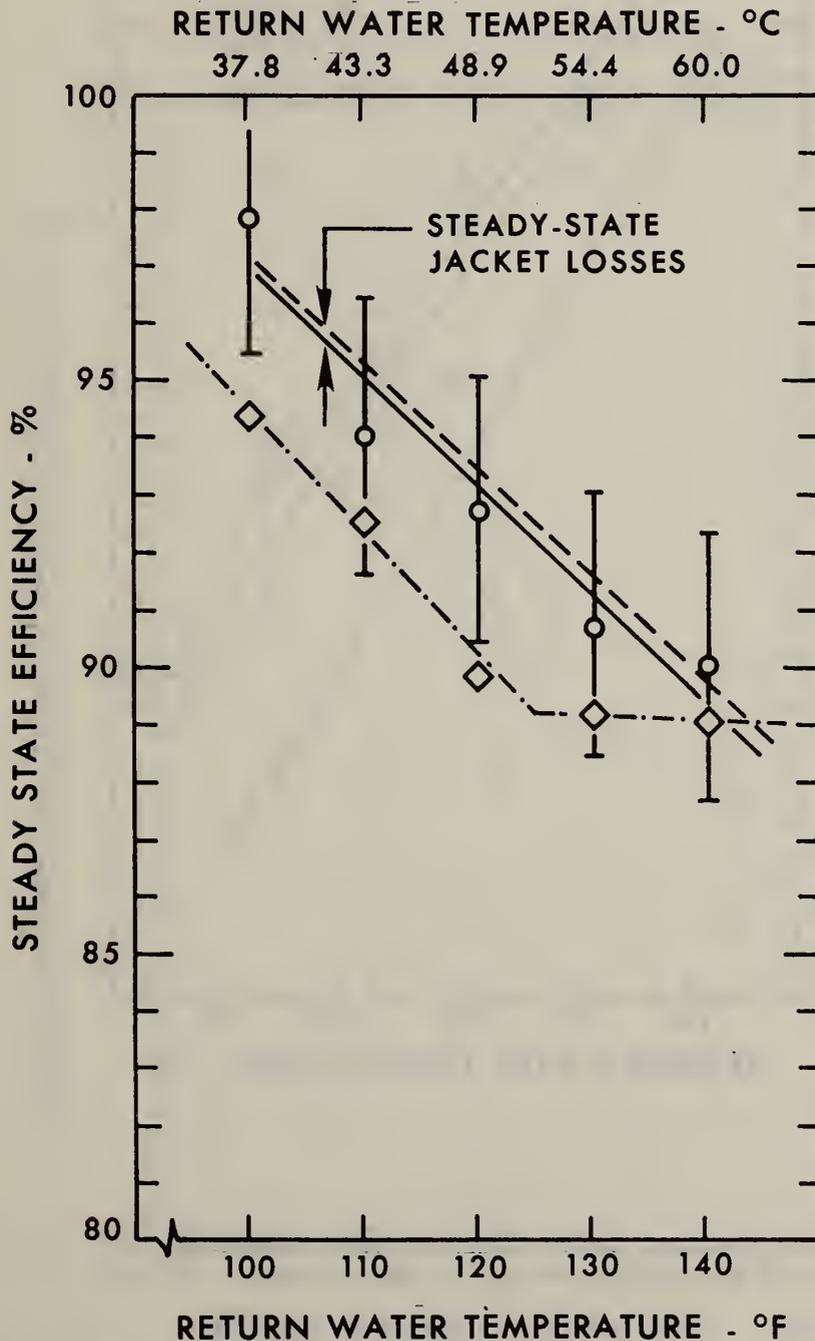
Figure 7. Steady-state efficiency vs. return water temperature.
