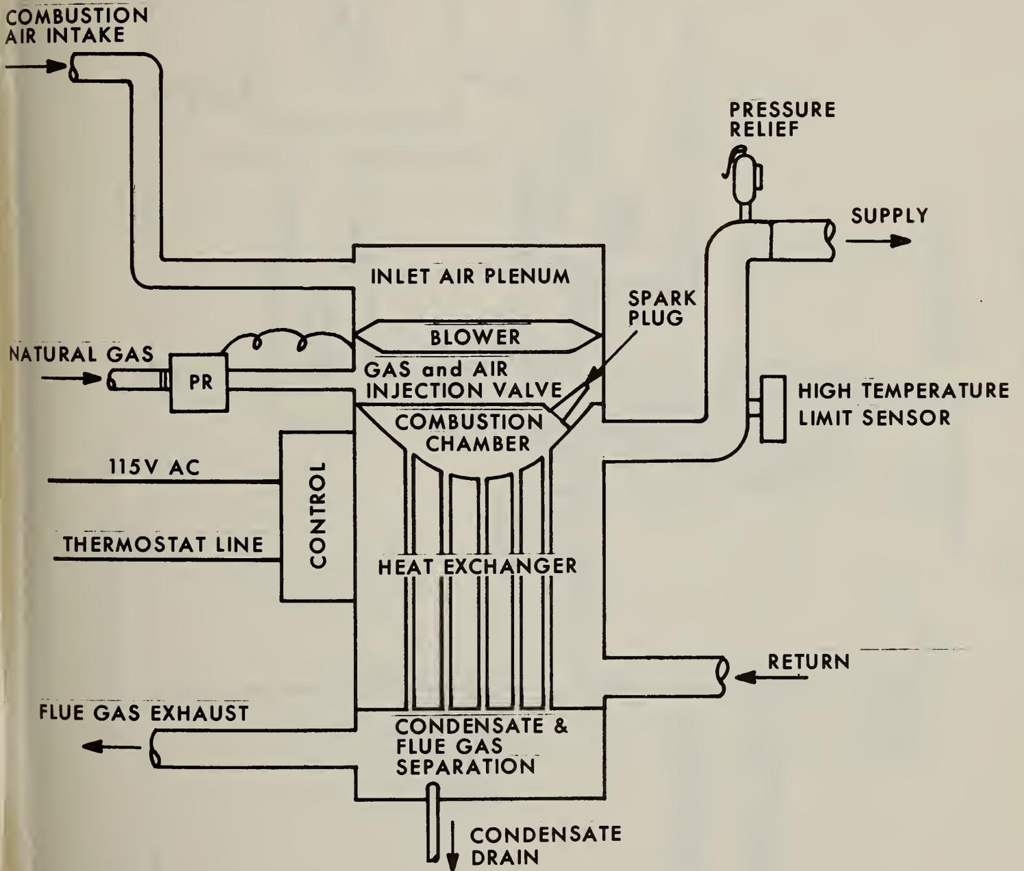
Figure 2. Pulse-combustion condensing boiler schematic.
