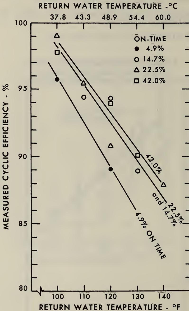
Figure 8. Cyclic efficiency at percent on-times of 4.9, 14.7, 22.5, and 42.0% as determined using input/output method.
