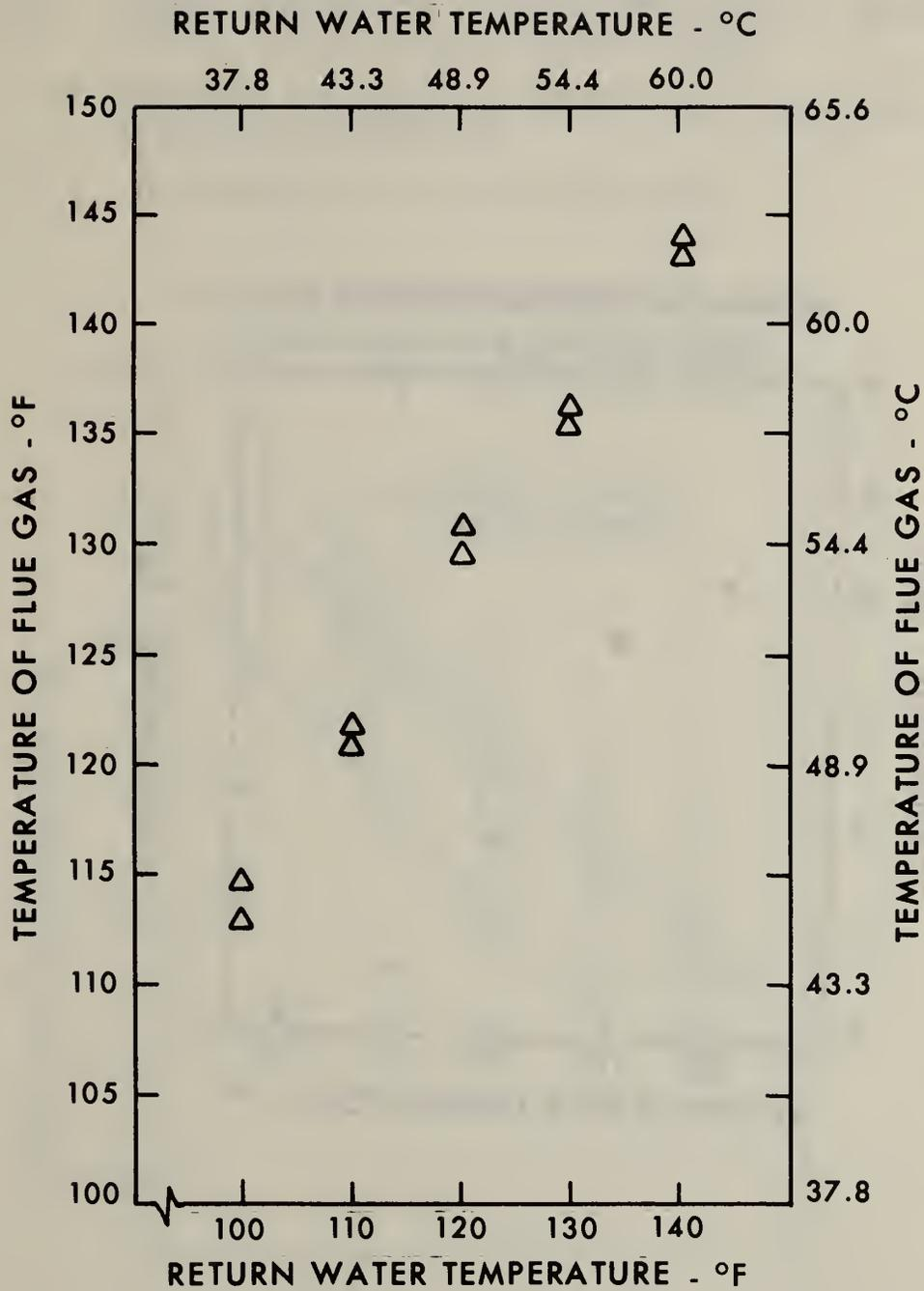
Figure 5. Flue gas temperature dependence on return water temperature from steady-state tests.
