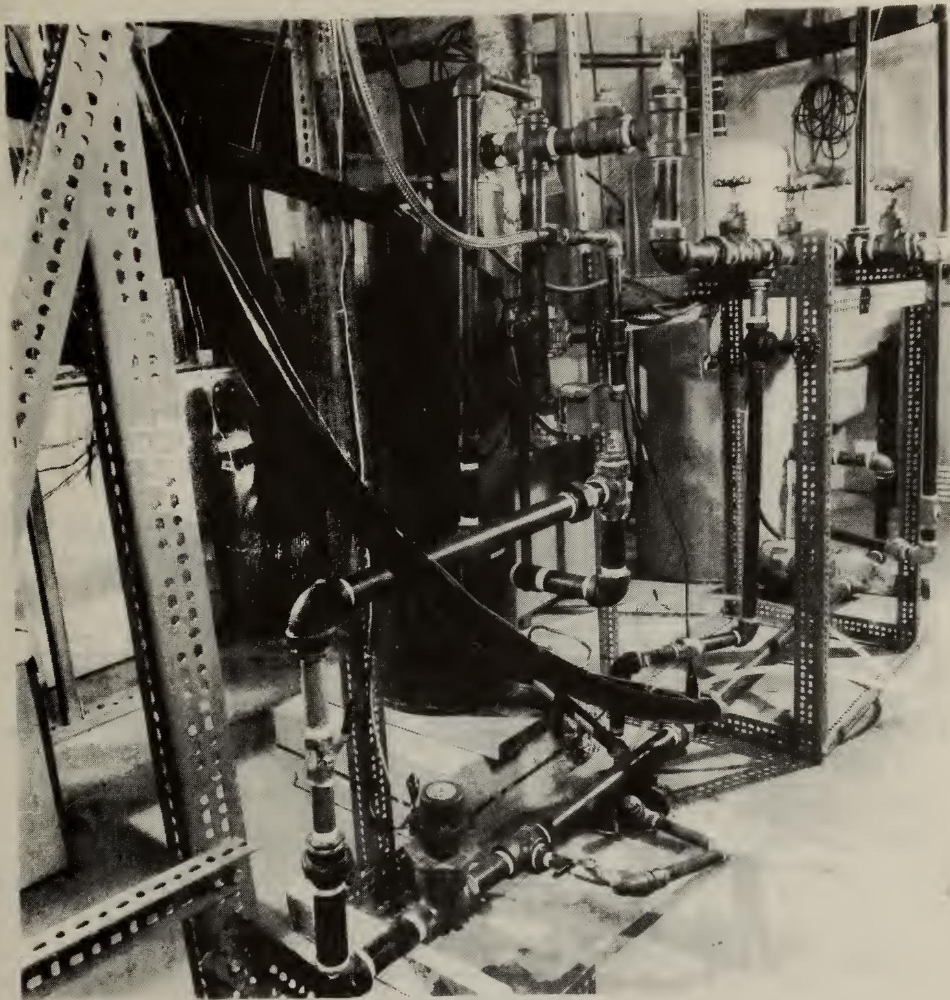
Figure 1. Condensing boiler test arrangement.
