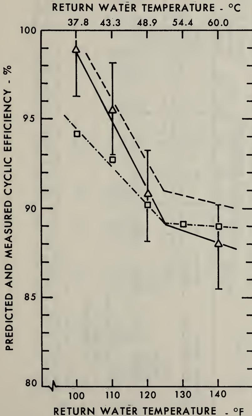
Figure 9. Cyclic efficiency at 22.5% on-time vs. return water temperature.
