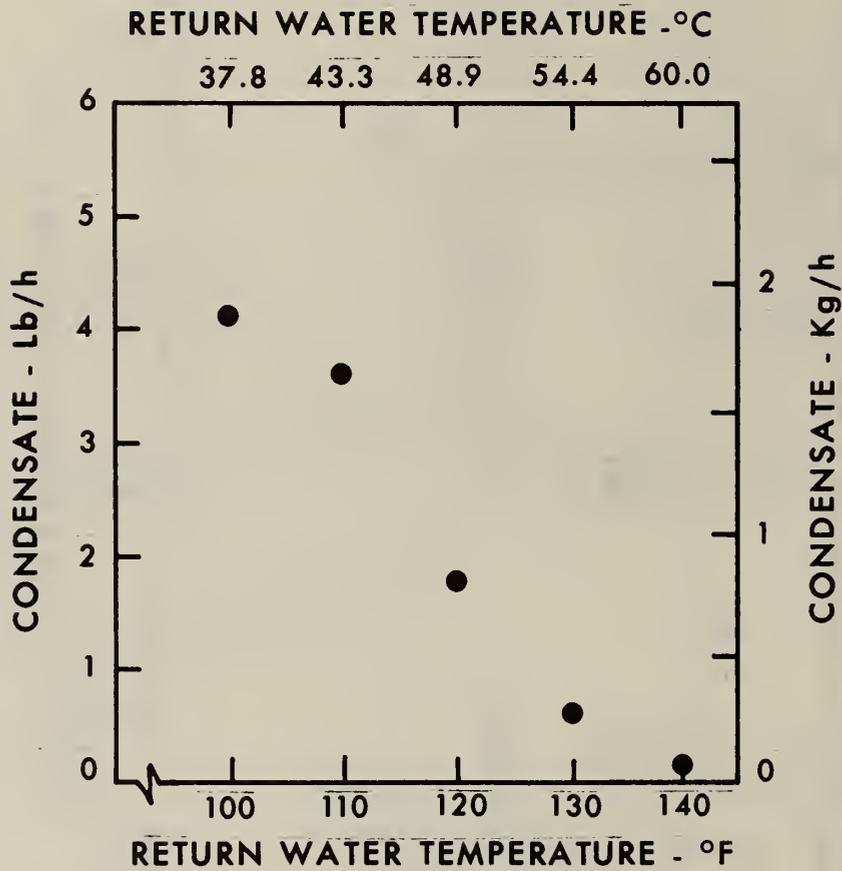
Figure 6. Condensate vs. return water temperature during steady-state tests
