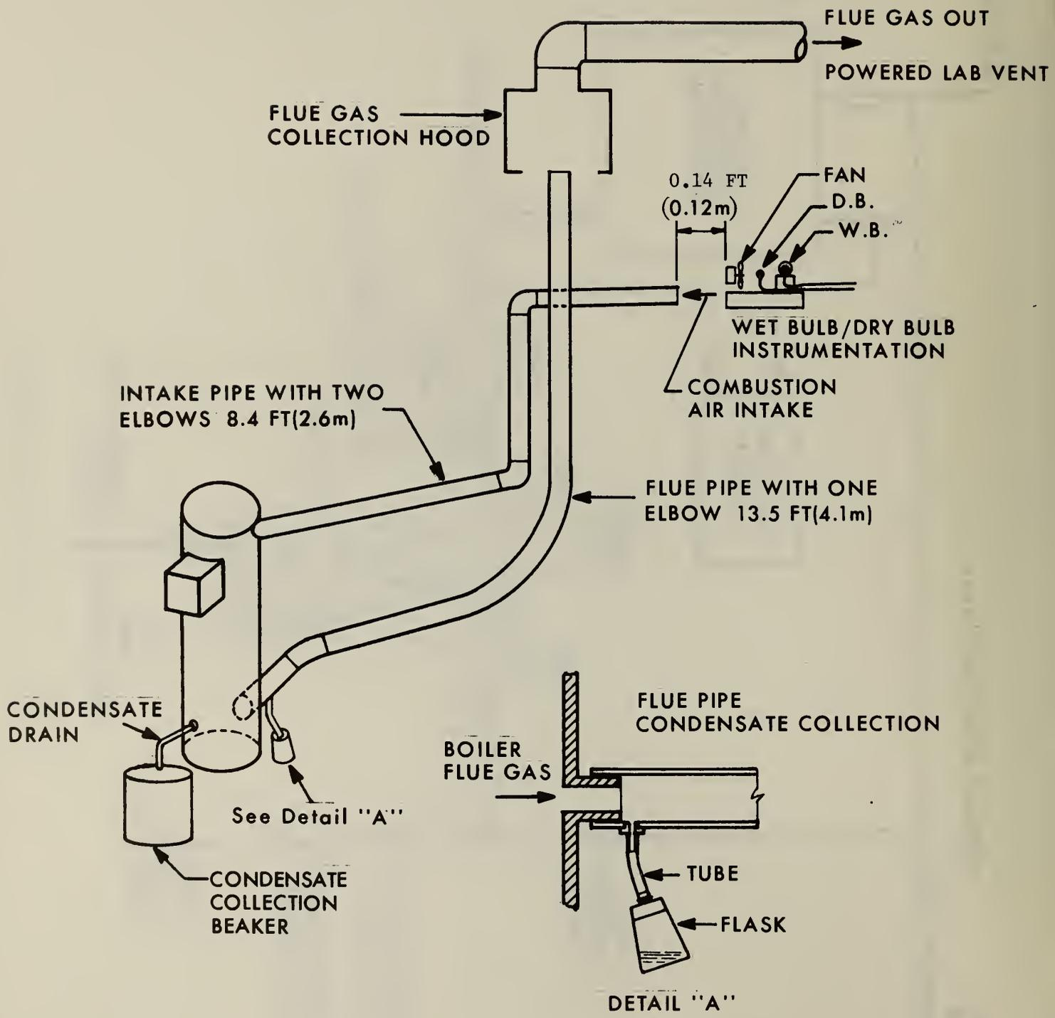
Figure 4. Exhaust/air intake installation.
