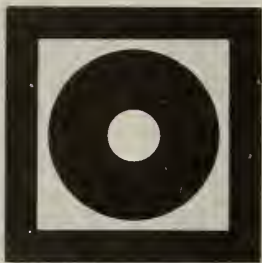
Fire Alarm Call Point (White on Red)
