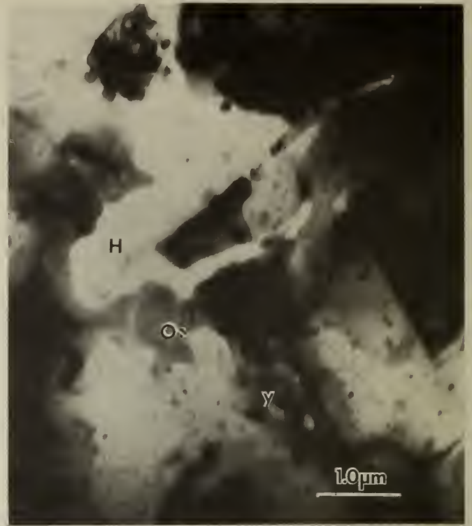
Fig. 5. Specimen at 750°C in 5300 Pa \text{O}_2 . The hole (H) and the film around it (Ox) were produced in \sim 30 min (Material-B-).
