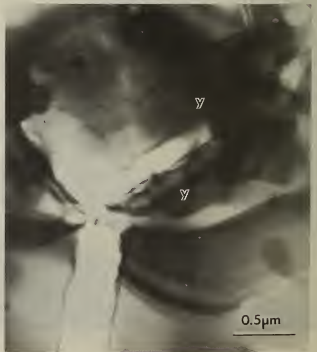
Fig. 7. Portion of in situ specimen which was under the grid, yttria phase (Y) is \text{Y}_4\text{Si}_2\text{O}_7\text{N}_2 .
