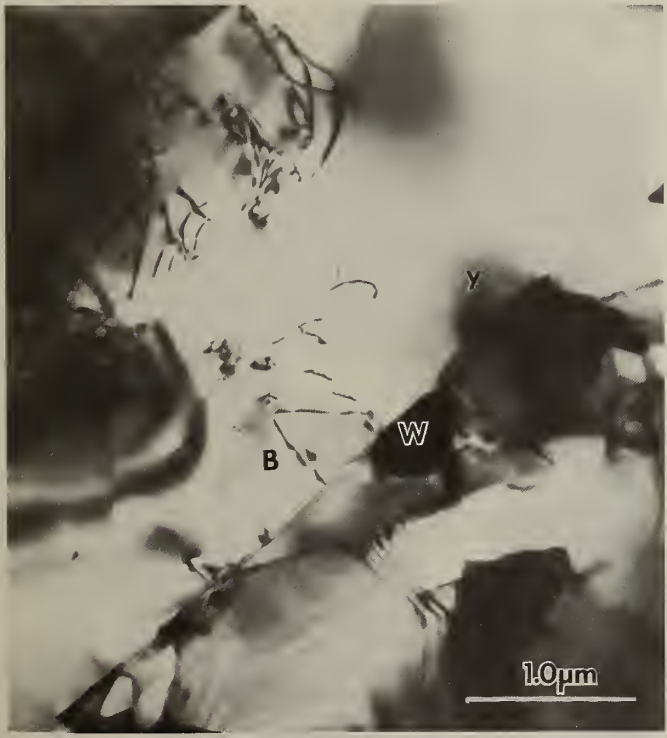
Fig. 2. Microstructure of hot-pressed \text{Si}_3\text{N}_4 + 8\% \text{Y}_2\text{O}_3 showing \beta\text{Si}_3\text{N}_4 ( \beta ), grains \text{YSiO}_2\text{N} phase (Y) WSi particles (W).
