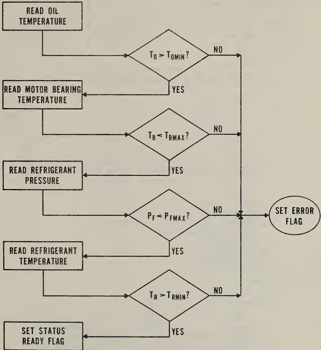
Figure 10 Generalized Chiller Control Logic with Microprocessor-STATUS
