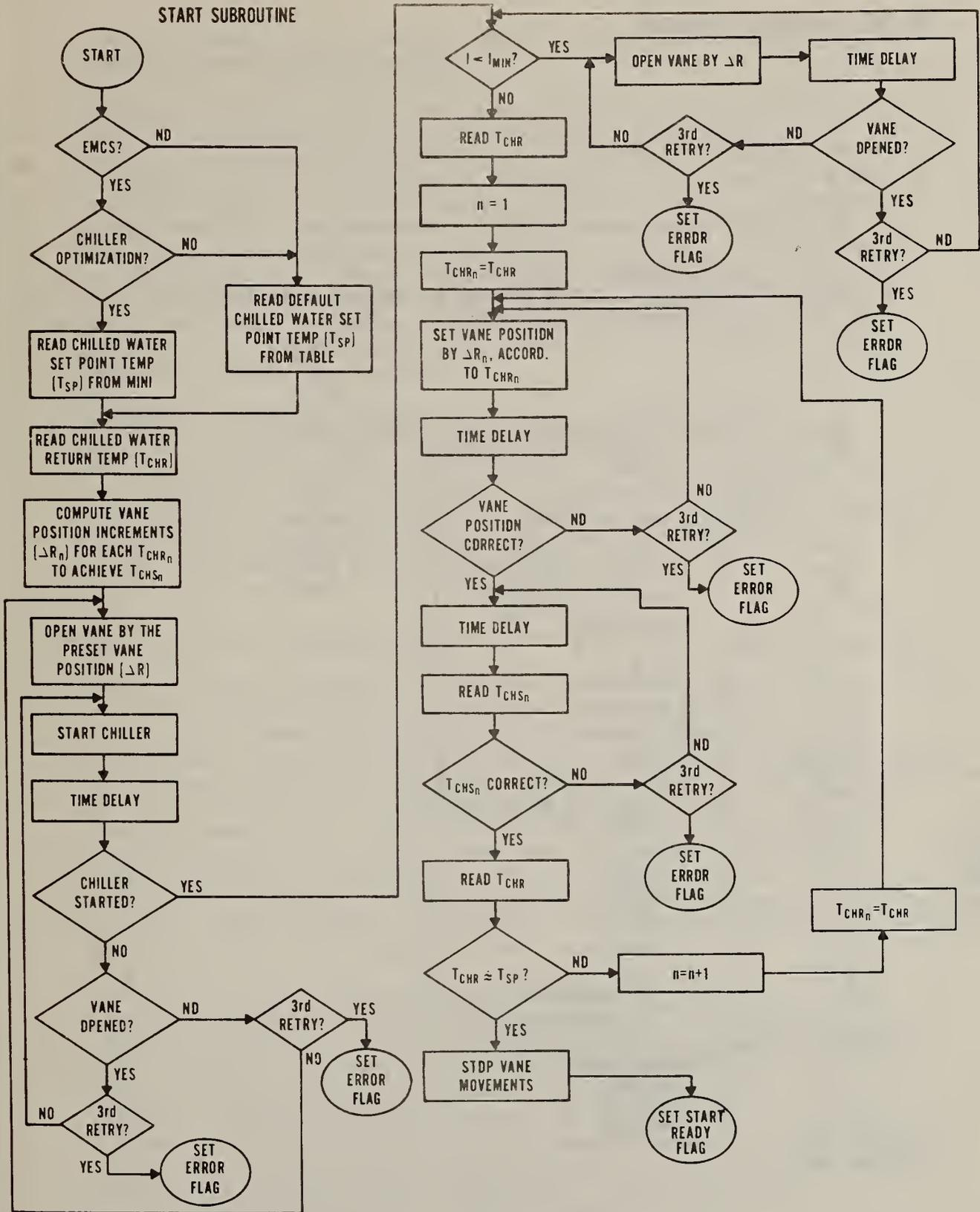
Figure 12 Generalized Chiller Control Logic with Microprocessor-START
