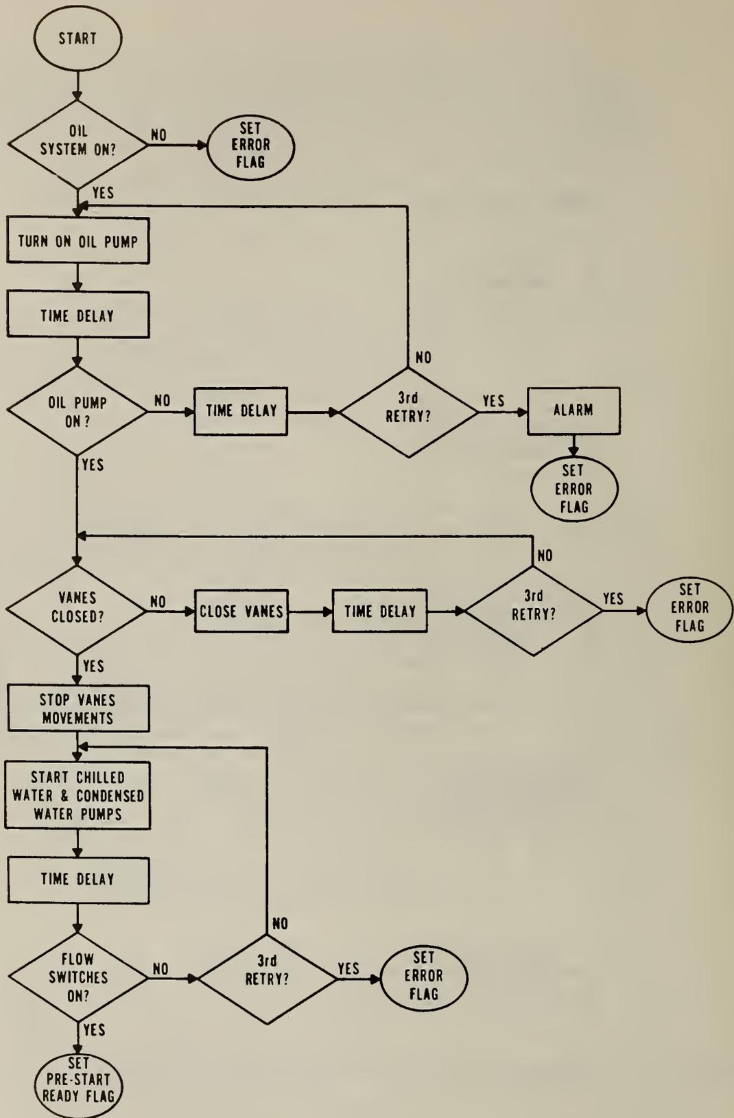
Figure 11 Generalized Chiller Control Logic with Microprocessor- PRE-START
