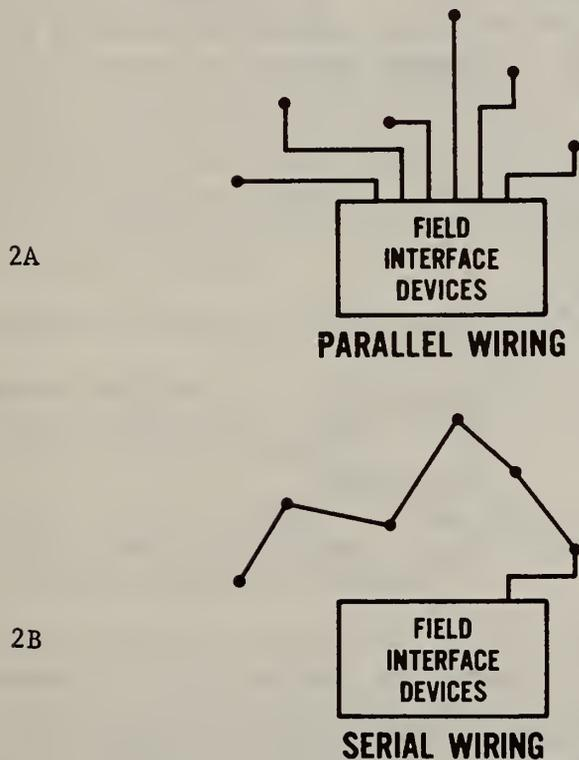
Figure 2 Connections of Sensors and Field Interface Devices
