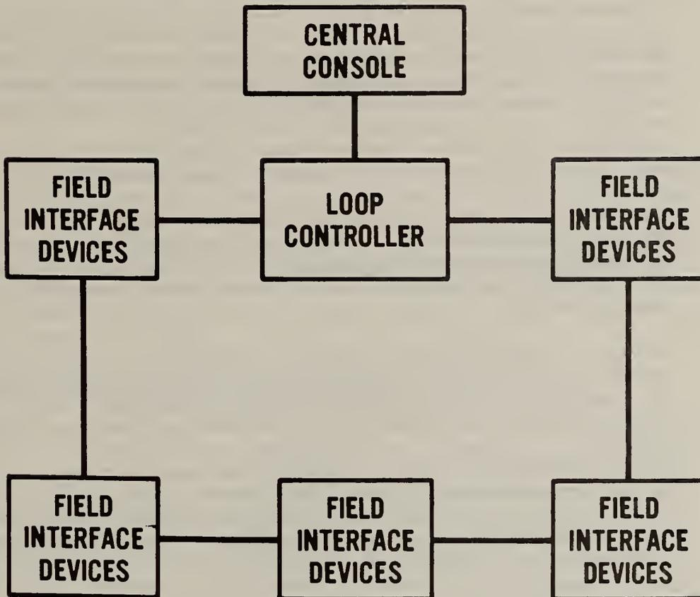
Figure 5 Interconnections of the "loop" System
