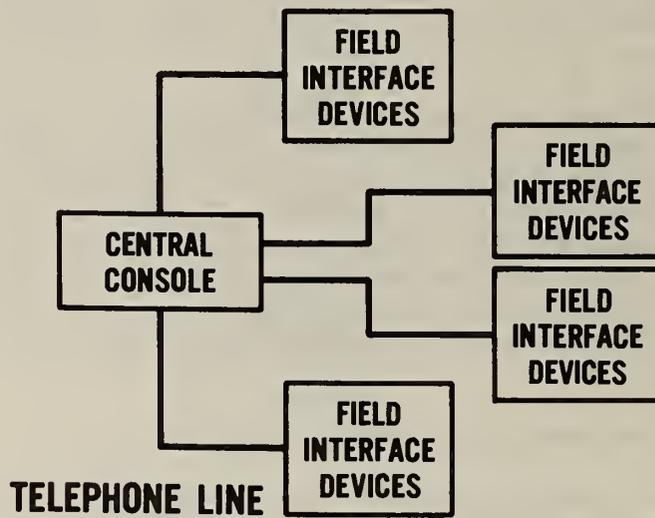
Figure 4 Typical Connections of Field Interface Devices and Central Console
