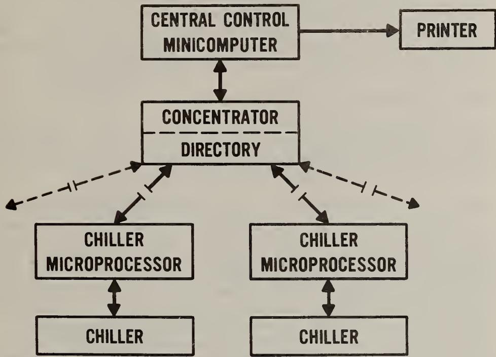
Figure 9 General Layout of Chiller Control Microprocessor with Minicomputer
