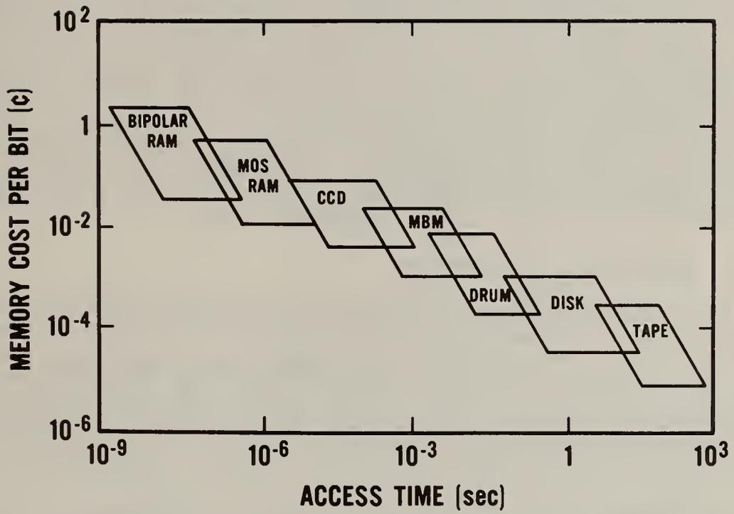
Figure 8 Comparison of Cost and Speed of Memory Systems
