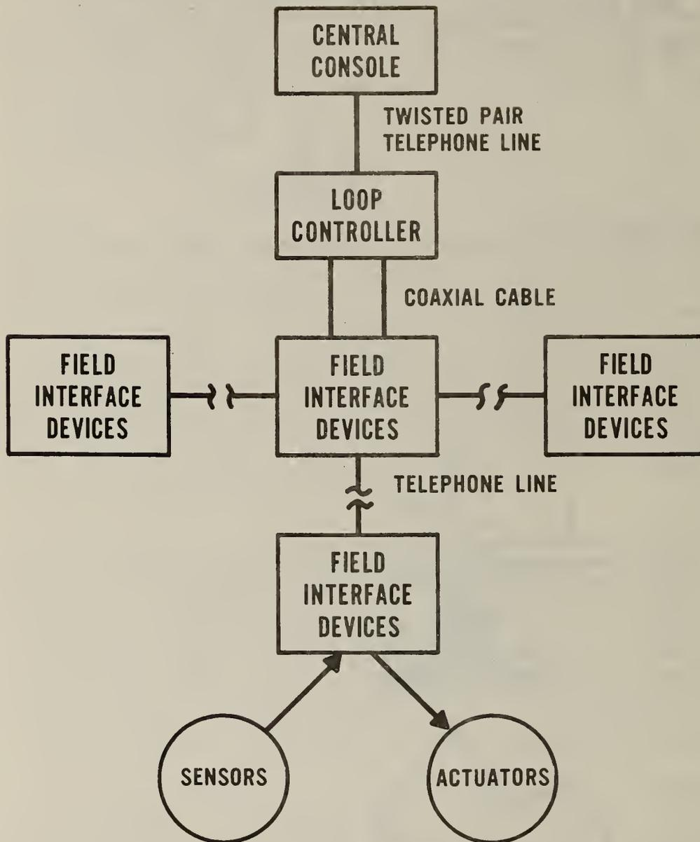
Figure 3 Hierarchy Configuration of the Centralized Control Systems
