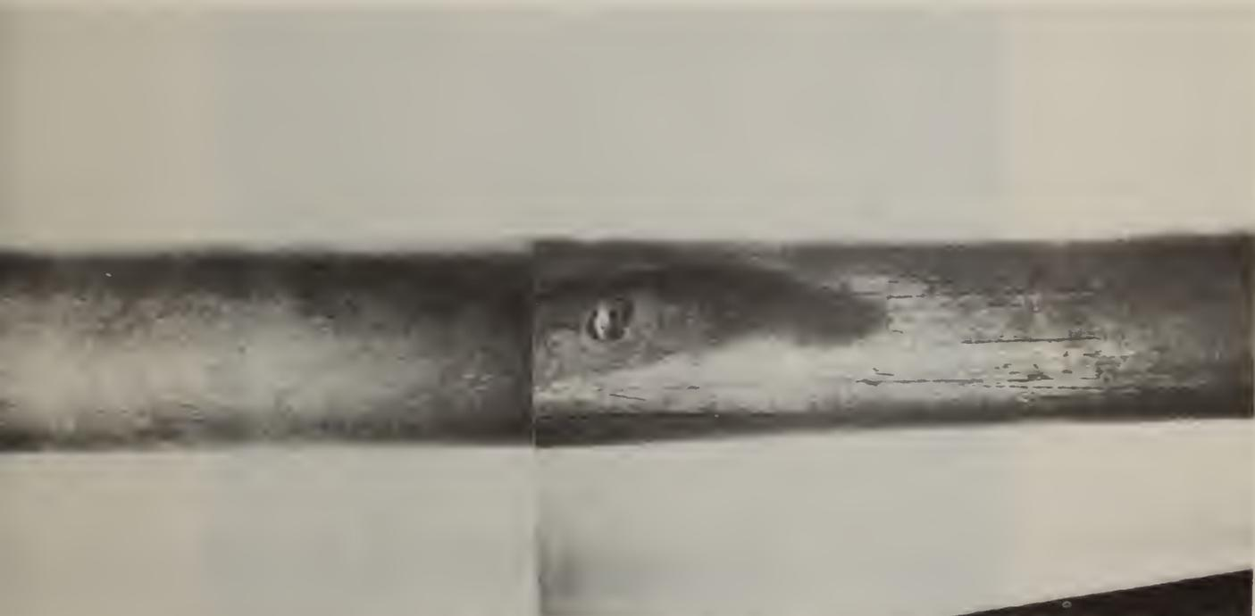
Fig. 14. Type 304 stainless steel after exposure for 4 hours at 400 °C to  $K_2SO_4$  seeded, oxygen rich hot gas stream and subsequent cleaning. Approximately 2 X.
