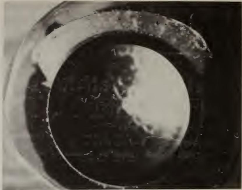
Fig. 3. Section of Type 316 stainless steel tubing after exposure to K<sub>2</sub>SO<sub>4</sub> seeded oxygen rich hot gas stream. Note formation of coating on the upper surface. Tube temperature 400 °C.
