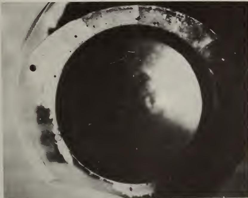
Fig. 2. Section of Type 316 stainless steel tubing after exposure to  $K_2SO_4$  seeded oxygen rich hot gas stream. Note formation of deposit on the upper surface. Tube temperature 500 °C.
