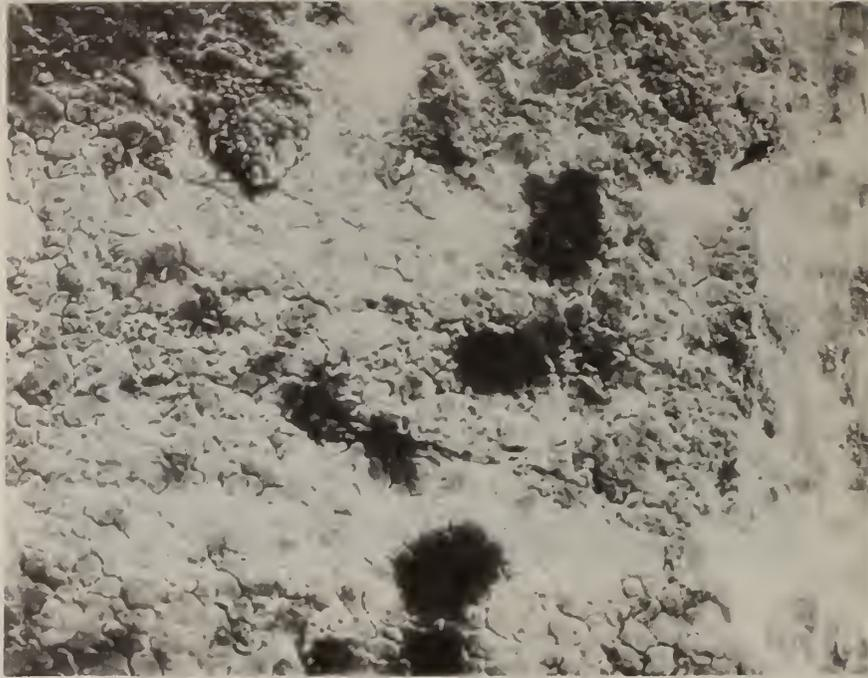
Fig. 22. SEM micrograph, 375 X, of another region specimen 14-4 showing what appears to be the onset of corrosion.
