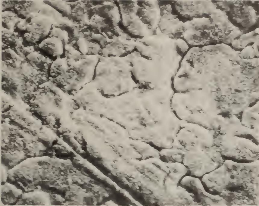
Fig. 26. SEM micrograph, 1400 X, of Type 304 stainless steel after exposure for 4 hours at 400 °C to a  $K_2SO_4$  seeded hot gas stream and subsequent cleaning. Note grain boundaries and grain surface.
