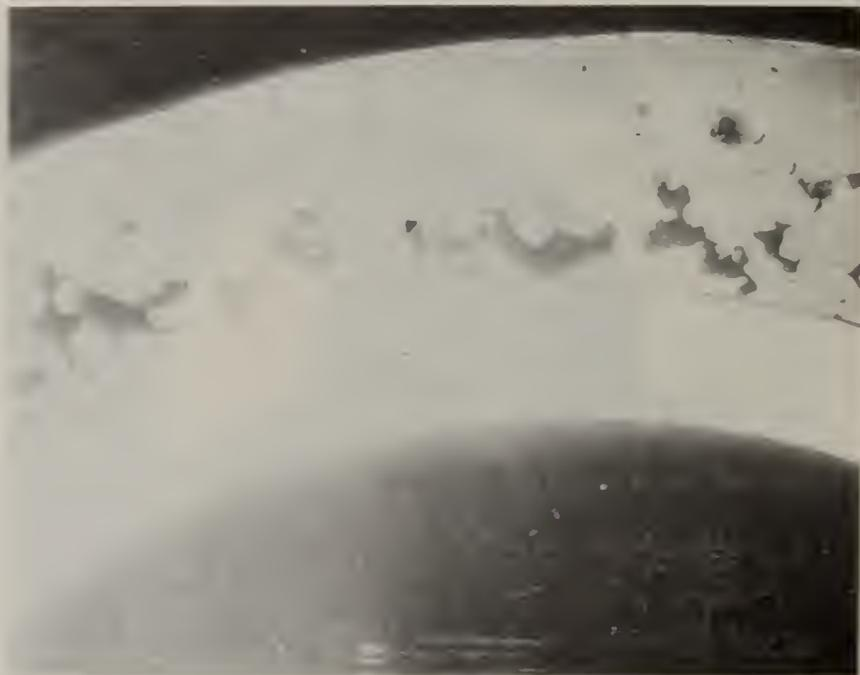
Fig. 4. SEM micrograph, 20 X, of K<sub>2</sub>SO<sub>4</sub> deposit on leading surface of Type 316 stainless steel. Specimen temperature 590 °C gas stream oxygen rich.
