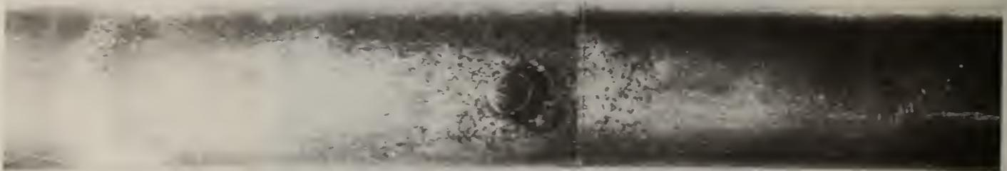
Fig. 12. Type 316 stainless steel after exposure for 4 hours at 590 °C to K<sub>2</sub>SO<sub>4</sub> seeded, oxygen rich hot gas stream and subsequent cleaning. Approximately 2 X.
