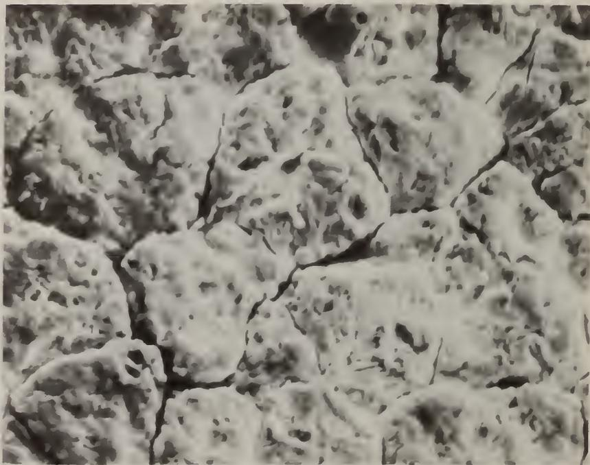
Fig. 25. SEM micrograph, 1900 X, of Type 304 stainless steel after exposure for 4 hours at 590 °C to a K<sub>2</sub>SO<sub>4</sub> seeded hot gas stream and subsequent cleaning. Note grain boundaries and grain surface.
