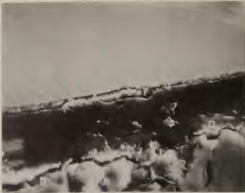
Fig. 7. SEM micrograph, 2000 X, of center region of Fig. 6 showing reaction area at interface. Lettered regions correspond to labeled EDX spectra, Figs. 7a-7h. Specimen temperature 590 °C, gas stream oxygen rich.
