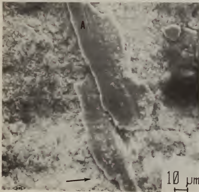
Fig. 21. (a) Entry region of wear scar on a DP80 specimen with sliding direction indicated by arrow. (b) Note crack in particle at (A) in one area of loose debris deposit.
