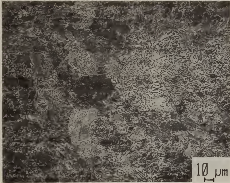
Fig. 4. 0-2 tool steel microstructure, etched in nital.
