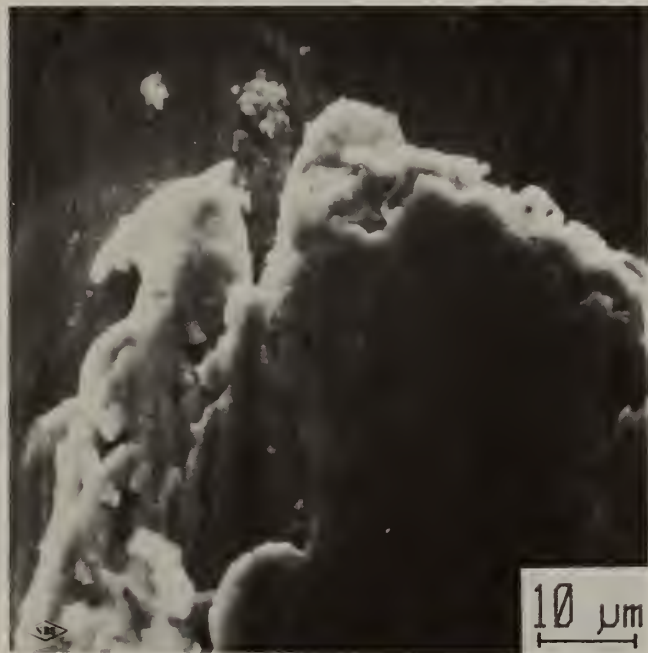
Fig. 17. Scanning electron micrograph of exit edge of wear scar on 1015 steel specimen surface. (a) arrow shows sliding direction. (b) evidence of deformation and fracture at edges of displaced material.
