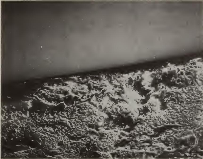
Fig. 5. SEM micrograph, 200 X, of small, high potassium concentration nodes in the salt deposit. Specimen temperature 500°C; gas stream oxygen rich.
