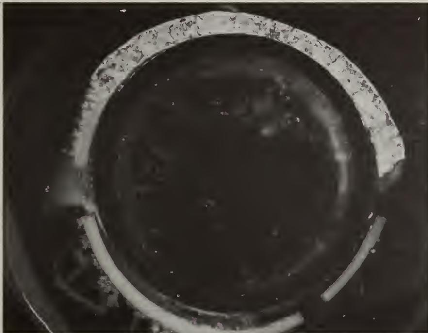
Fig. 11. Section of Type 304 stainless steel tubing after exposure to  $K_2CO_3/K_2SO_4$  seeded fuel rich hot gas stream. Note formation of 0.8 mm deposit on upper surface. Tube temperature  $400^\circ C$ . 6 X.
