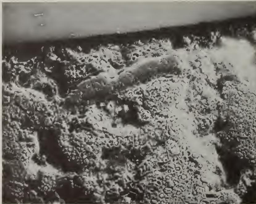
Fig. 4. SEM micrograph, 200 X, of small, high potassium concentration nodes in the salt deposit. Specimen temperature  $400^\circ C$ ; gas stream oxygen rich.
