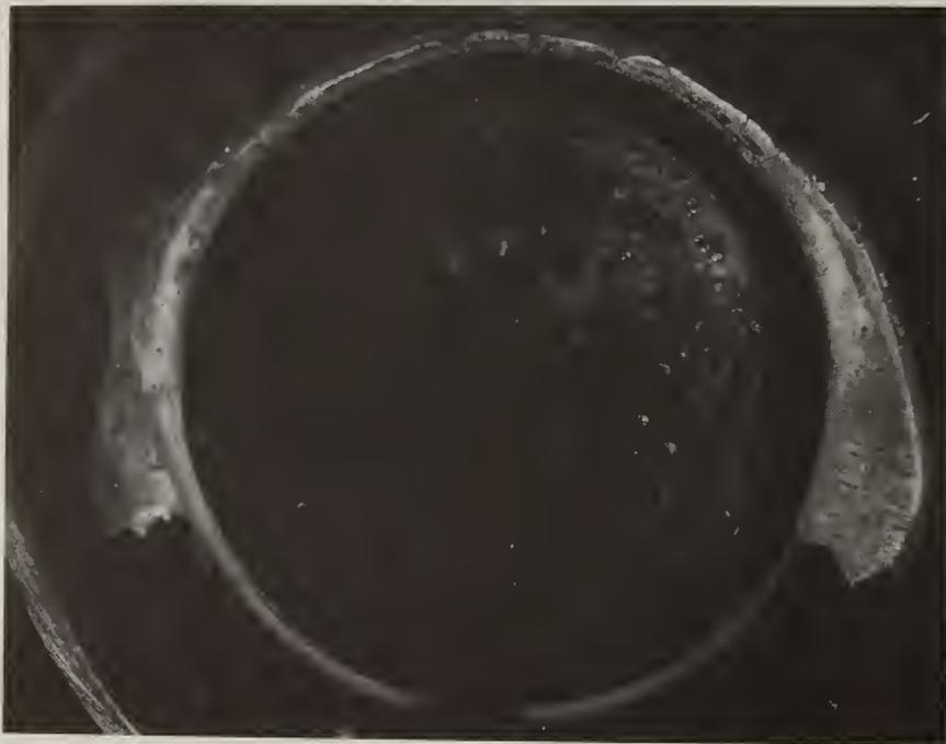
Fig. 13. Section of Type 304 stainless steel tubing after exposure to  $K_2CO_3/K_2SO_4$  seeded fuel rich hot gas stream. Note formation of thin deposit on upper surface. Tube temperature  $590^\circ C$ . 6 X.
