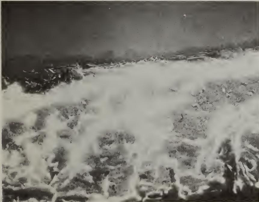
Fig. 6. SEM micrograph, 200 X, of salt deposit showing absence of high potassium concentration nodules. Specimen temperature 590°C; gas stream oxygen rich.
