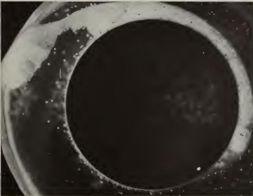
Fig. 2. Section of Type 304 stainless steel tubing after exposure to  $K_2CO_3/K_2SO_4$  seeded oxygen rich hot gas stream. Note formation of thick deposit, 1 mm on upper surface. Tube temperature 500°C. 6 X.
