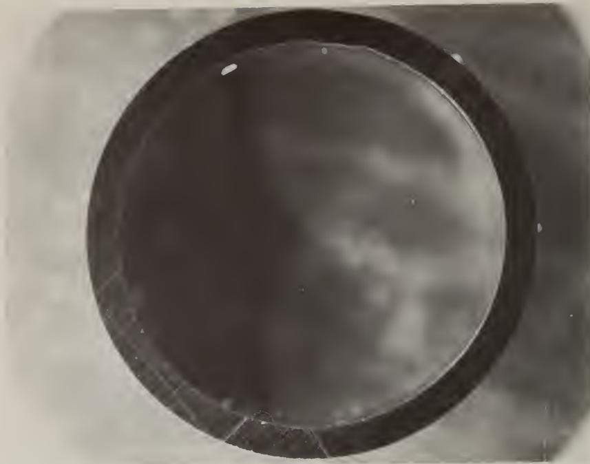
Fig. 16. Section of Type 304 stainless steel prior to exposure to the seeded hot gas stream. 6 X.
