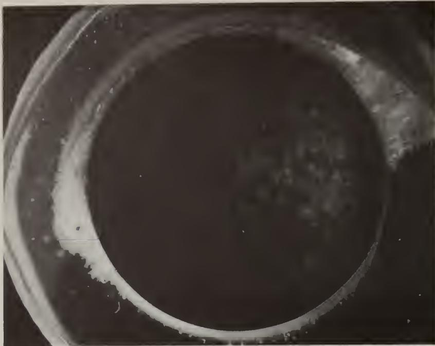
Fig. 3. Section of Type 304 stainless steel tubing after exposure to  $K_2CO_3/K_2SO_4$  seeded oxygen rich hot gas stream. Note formation of thinner deposit on upper surface. Tube temperature  $590^\circ C$ . 6 X.
