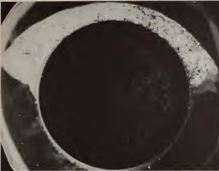
Fig. 1. Section of Type 304 stainless steel tubing after exposure to  $K_2CO_3/K_2SO_4$  seeded oxygen rich hot gas stream. Note formation of thick deposit, 1.7 mm, on upper surface and thin powdery deposit on lower surface. Tube temperature 400°C. 6 X.
