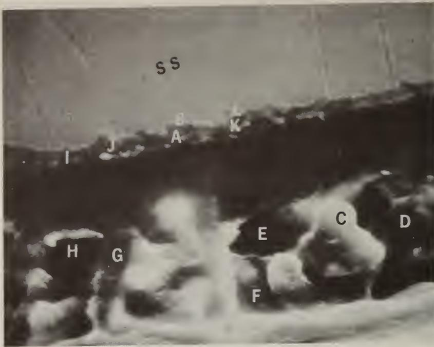
Fig. 7. SEM micrograph, 2000 X, of stainless steel-salt deposit reaction zone. Lettered regions correspond to labeled EDX spectra, figures 7a through 7f. Specimen temperature 500°C; gas stream oxygen rich.
