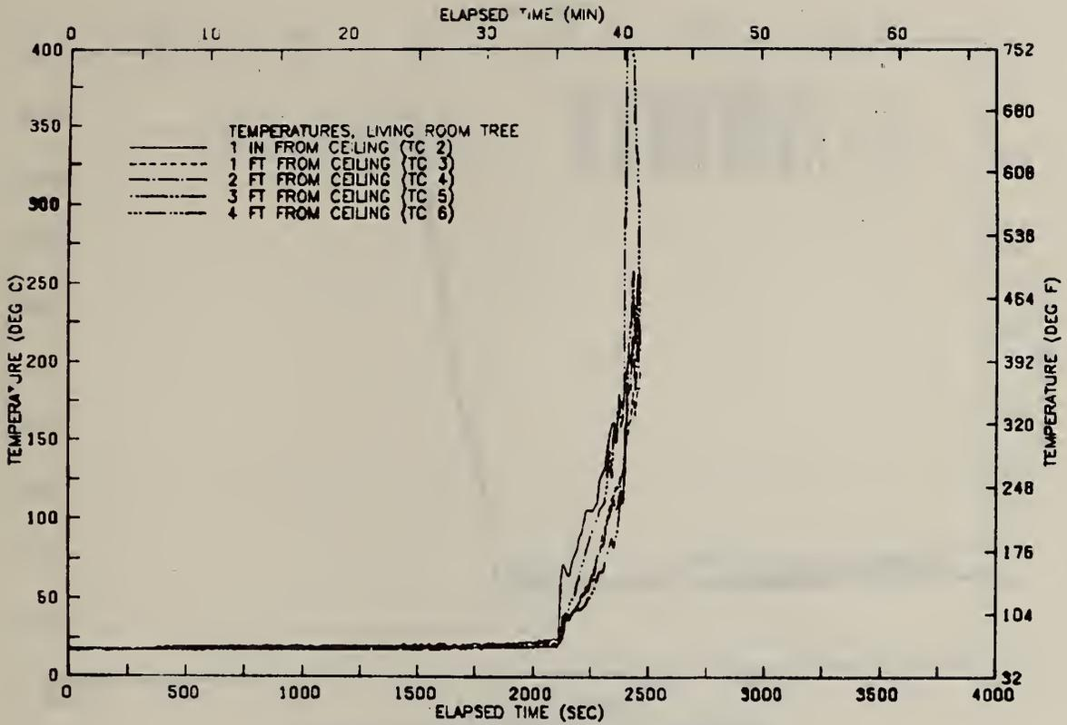
FIGURE B1 VERTICAL TEMP. PROFILE ABOVE CHAIR-TEST 14
