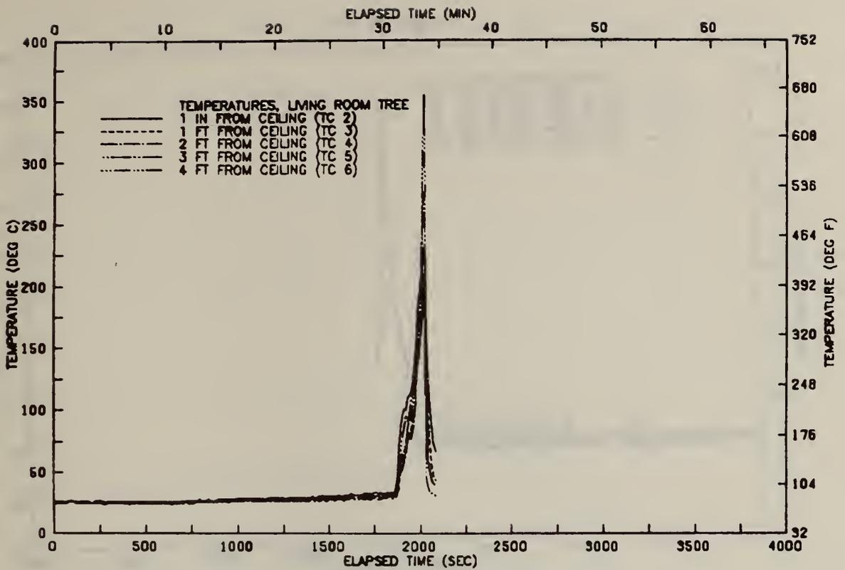
FIGURE A1 VERTICAL TEMP. PROFILE ABOVE CHAIR-TEST 01
