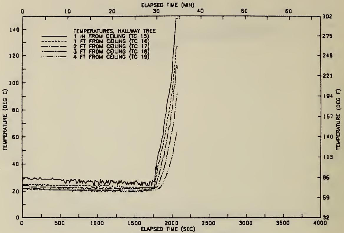
FIGURE B35 VERTICAL TEMP. PROFILE IN HALLWAY-TEST 17
