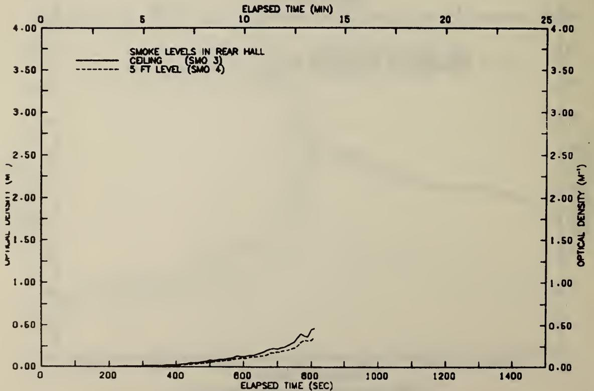
FIGURE A78 SMOKE LEVELS IN REAR HALLWAY-TEST 08
