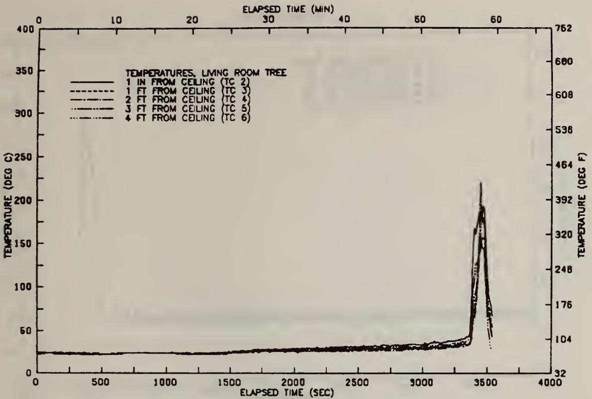
FIGURE A31 VERTICAL TEMP. PROFILE ABOVE CHAIR-TEST 04
