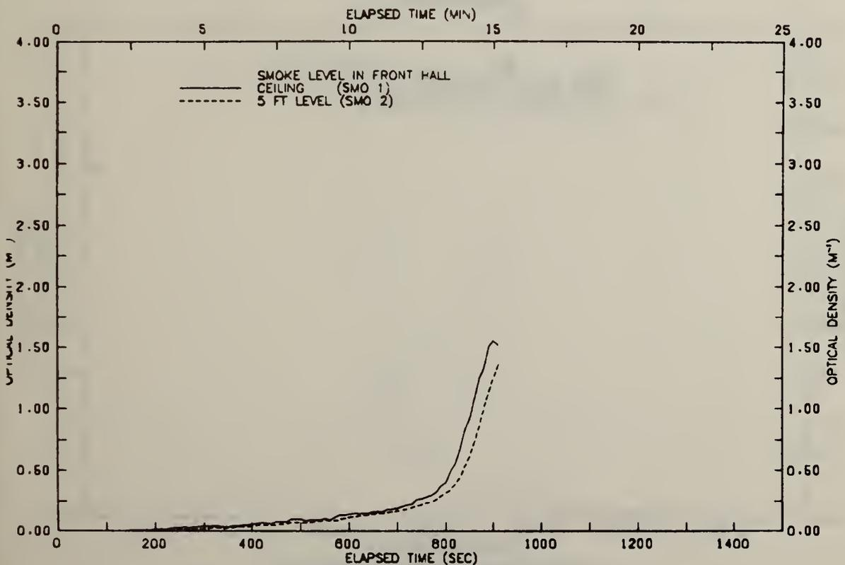
FIGURE B62 SMOKE LEVELS IN FRONT HALLWAY—TEST 19
