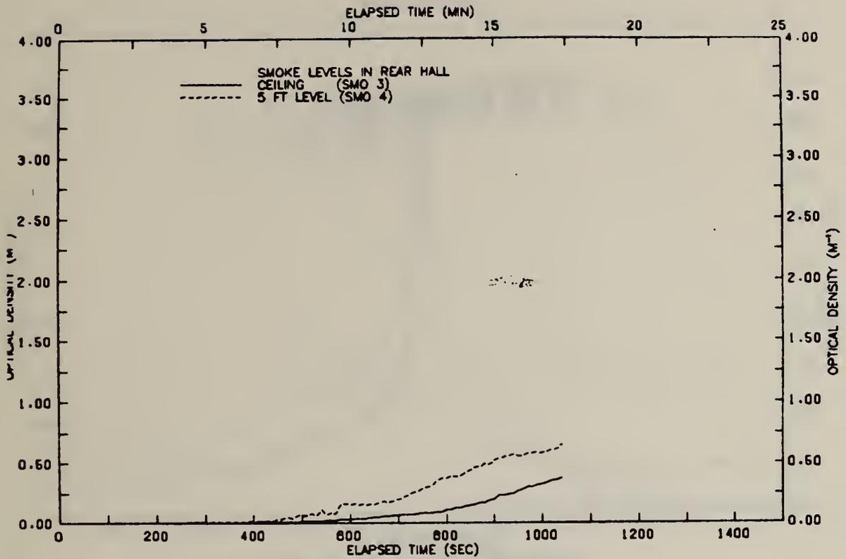
FIGURE B85 SMOKE LEVELS IN REAR HALLWAY—TEST 21
