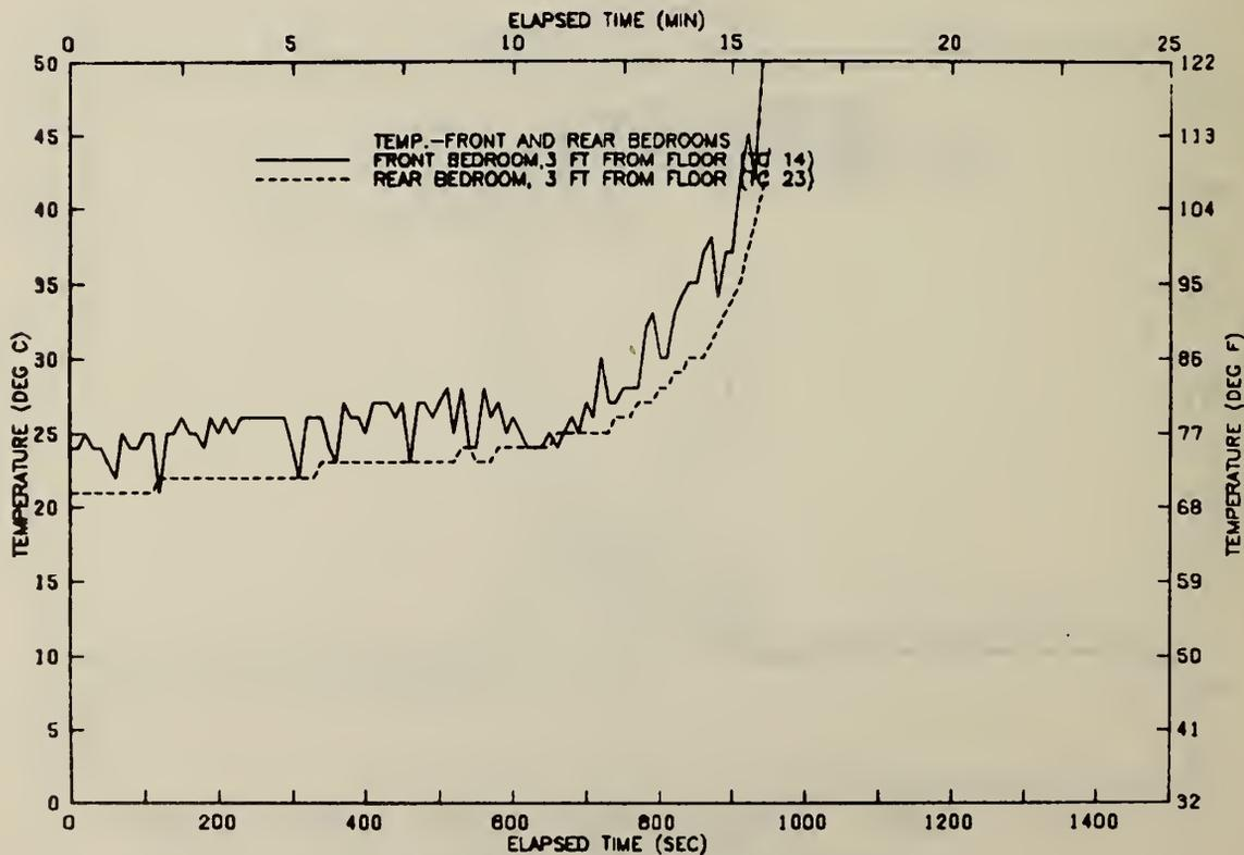
FIGURE B72 TEMP. IN FRONT AND REAR BEDROOMS—TEST 20
