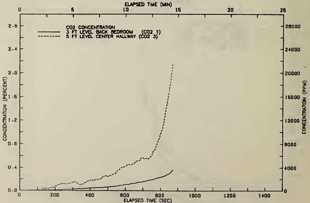
FIGURE A110B CARBON DIOXIDE CONCENTRATION-TEST 1
