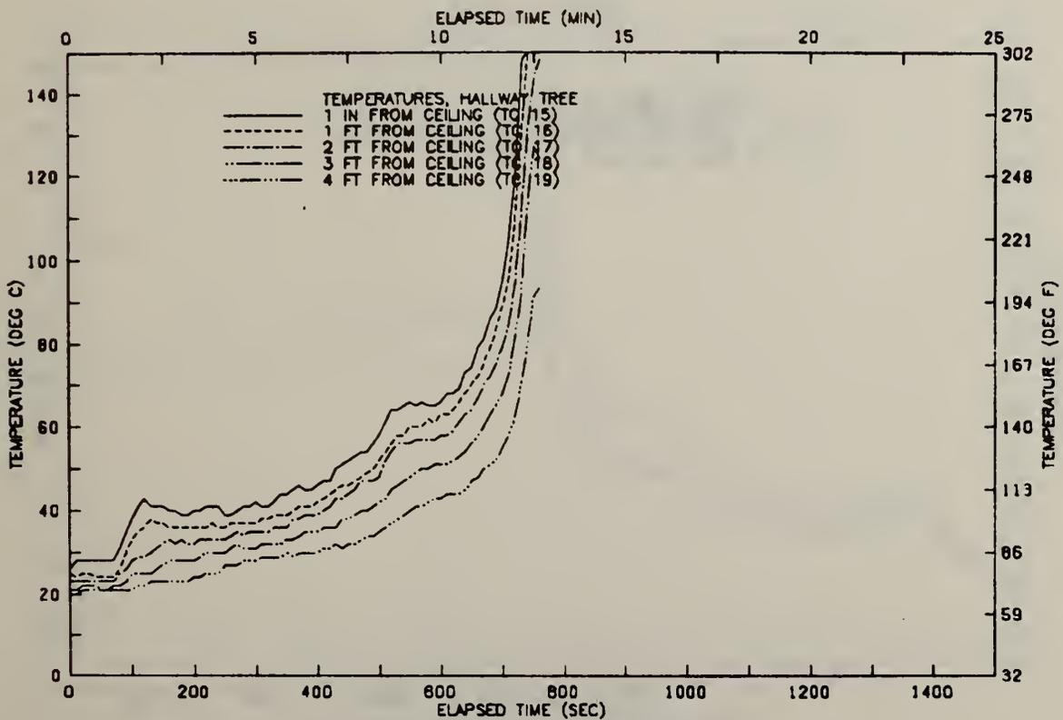
FIGURE B90 VERTICAL TEMP. PROFILE IN HALLWAY—TEST 22
