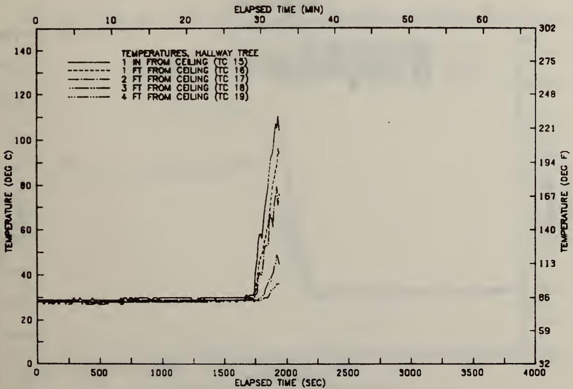
FIGURE A62 VERTICAL TEMP. PROFILE IN HALLWAY-TEST 07
