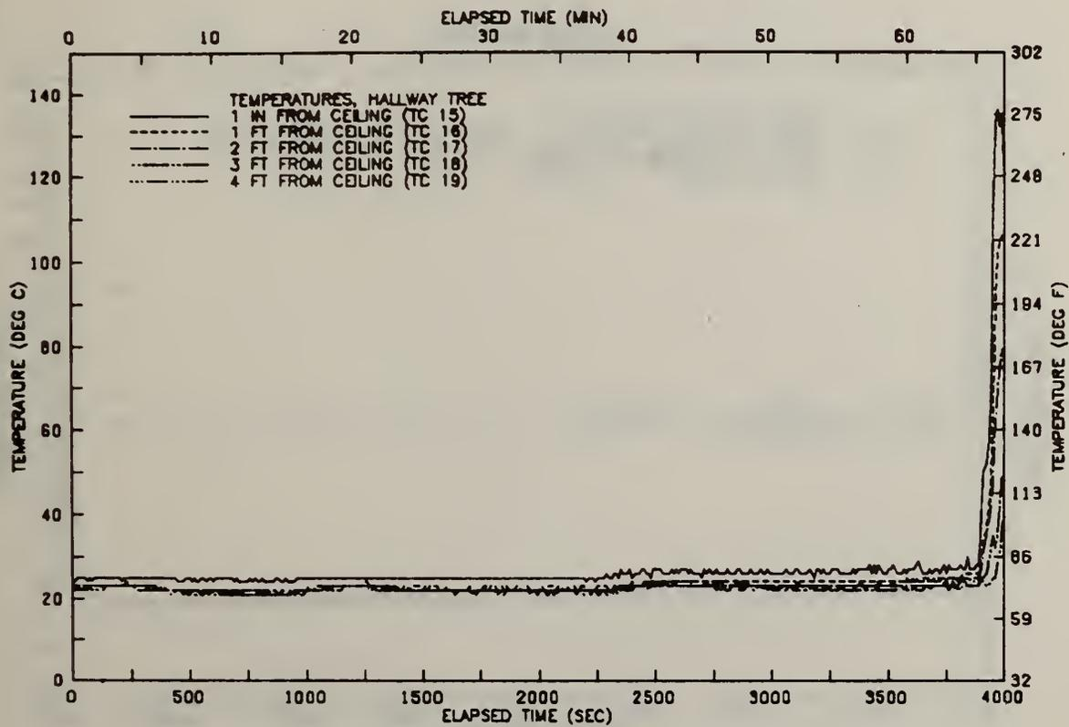
FIGURE A52 VERTICAL TEMP. PROFILE IN HALLWAY-TEST 06
