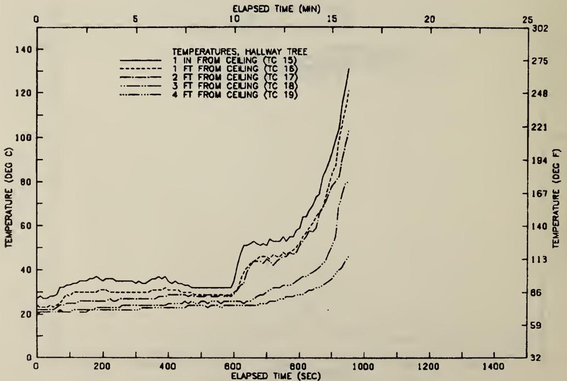
FIGURE B68 VERTICAL TEMP. PROFILE IN HALLWAY—TEST 20
