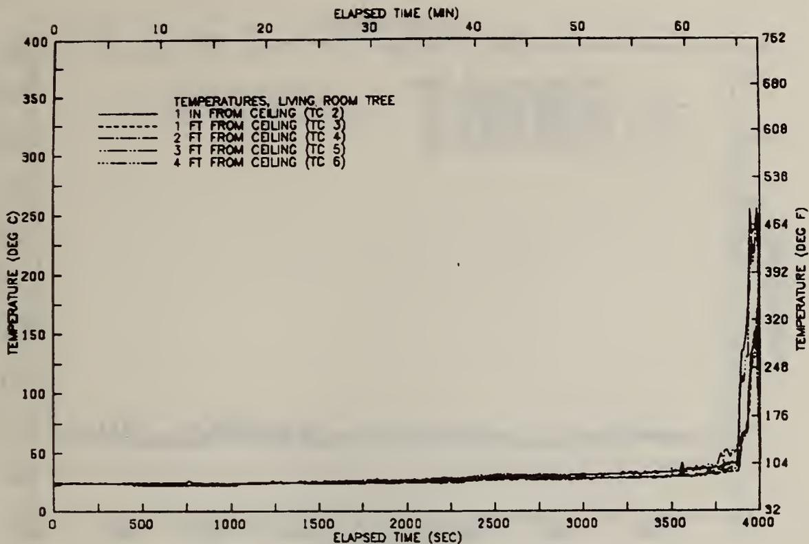
FIGURE A51 VERTICAL TEMP. PROFILE ABOVE CHAIR-TEST 06
