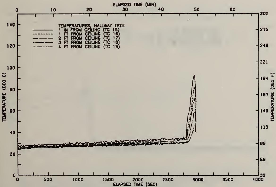
FIGURE A42 VERTICAL TEMP. PROFILE IN HALLWAY-TEST 05
