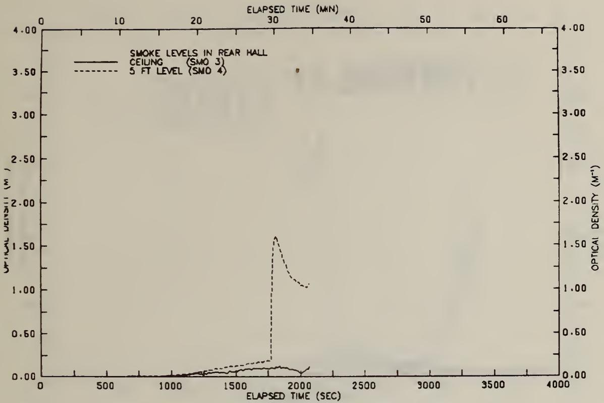
FIGURE B41 SMOKE LEVELS IN REAR HALLWAY-TEST 17
