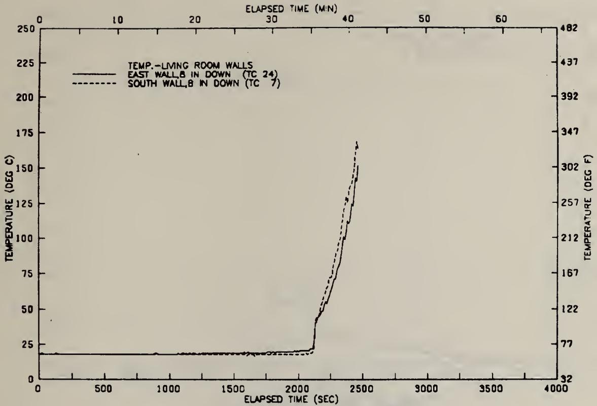
FIGURE B5 TEMPERATURE AT LIVING ROOM WALLS—TEST 14
