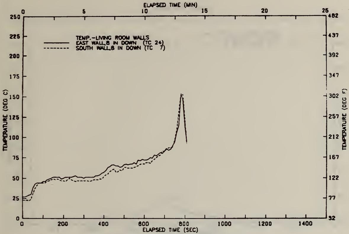
FIGURE A75 TEMPERATURE AT LIVING ROOM WALLS—TEST 08
