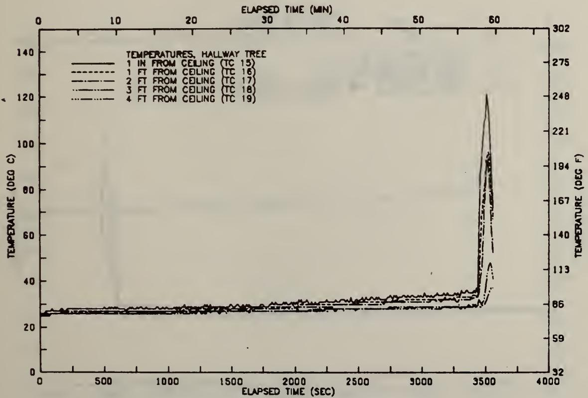
FIGURE A22 VERTICAL TEMP. PROFILE IN HALLWAY-TEST 03
