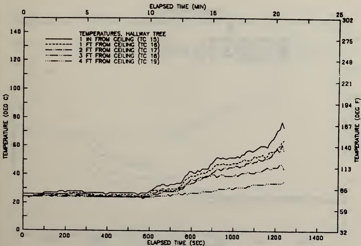
FIGURE A92 VERTICAL TEMP. PROFILE IN HALLWAY-TEST 10
