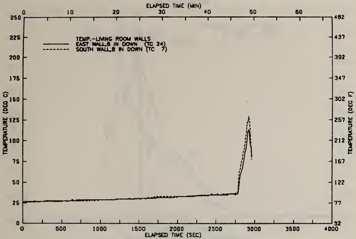
FIGURE A45 TEMPERATURE AT LIVING ROOM WALLS—TEST 05
