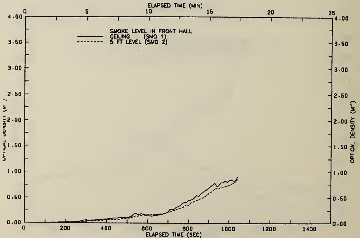
FIGURE B84 SMOKE LEVELS IN FRONT HALLWAY—TEST 21
