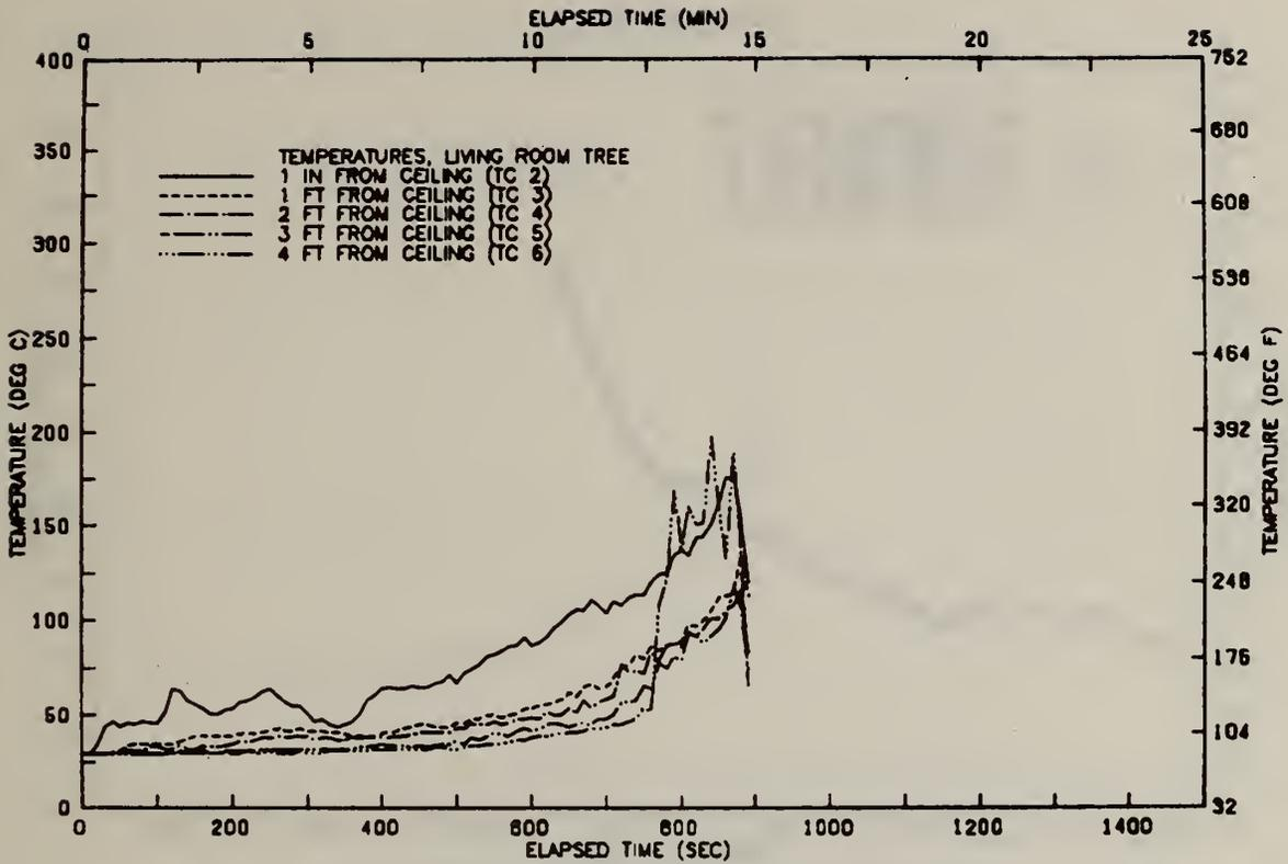
FIGURE A111 VERTICAL TEMP. PROFILE ABOVE CHAIR-TEST 12
