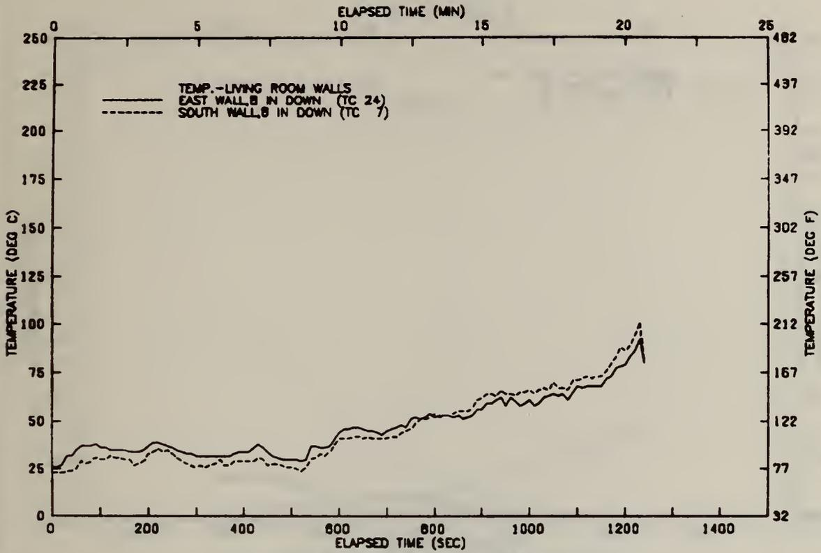
FIGURE A95 TEMPERATURE AT LIVING ROOM WALLS-TEST 10
