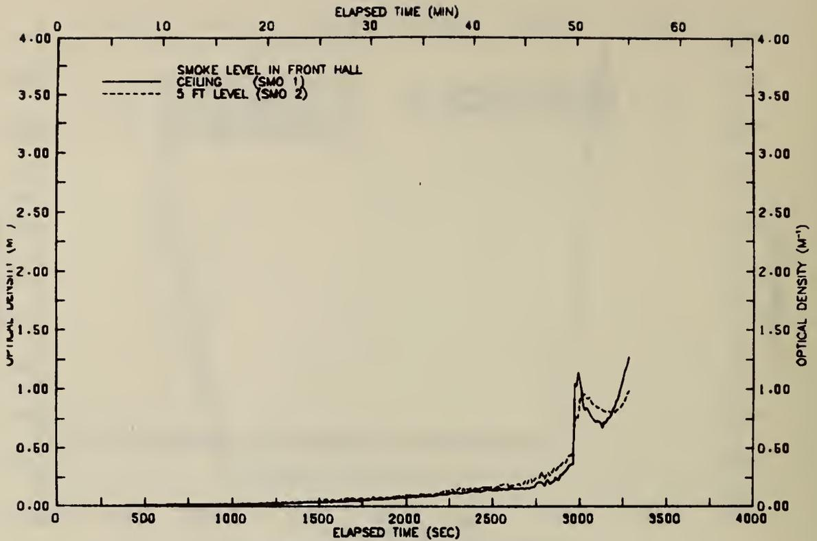
FIGURE B51 SMOKE LEVELS IN FRONT HALLWAY-TEST 18
