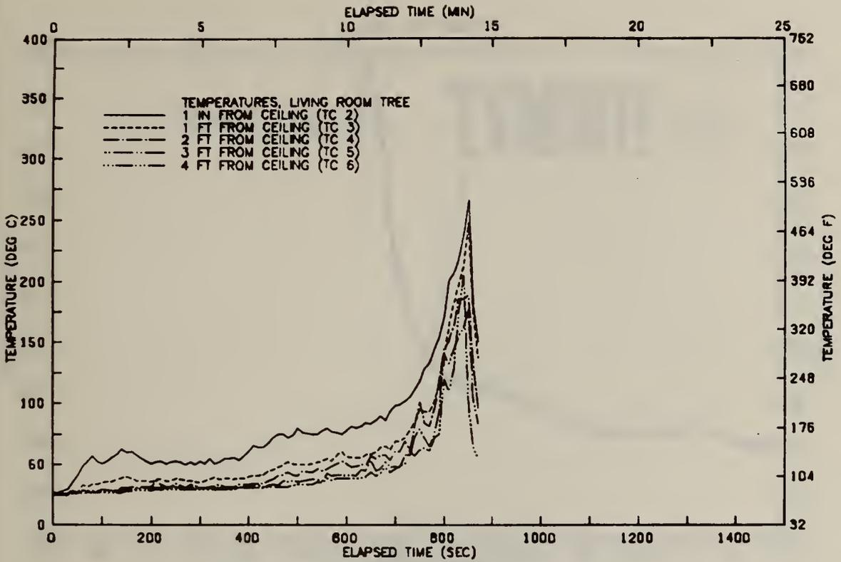
FIGURE A101 VERTICAL TEMP. PROFILE ABOVE CHAIR—TEST 11
