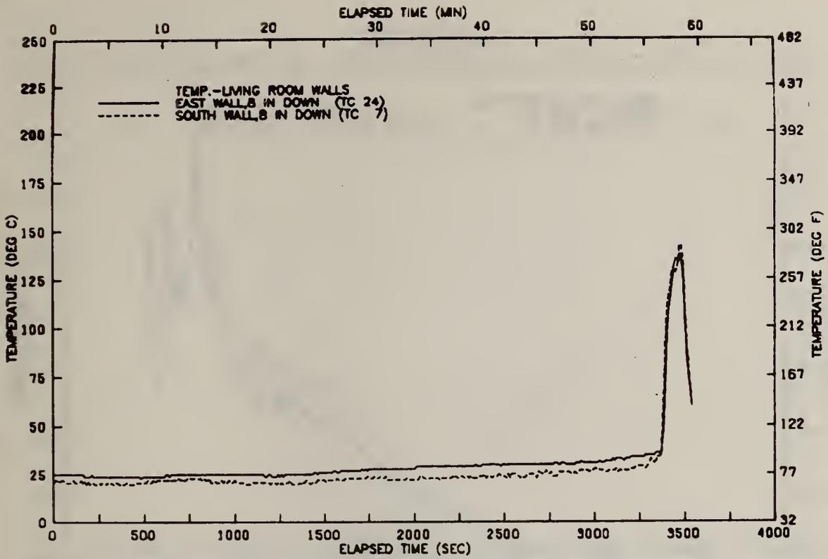
FIGURE A35 TEMPERATURE AT LIVING ROOM WALLS-TEST 04
