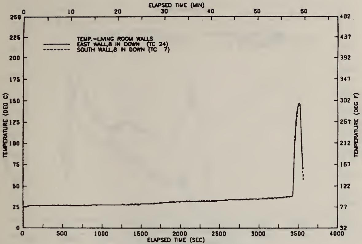
FIGURE A25 TEMPERATURE AT LIVING ROOM WALLS—TEST 03
