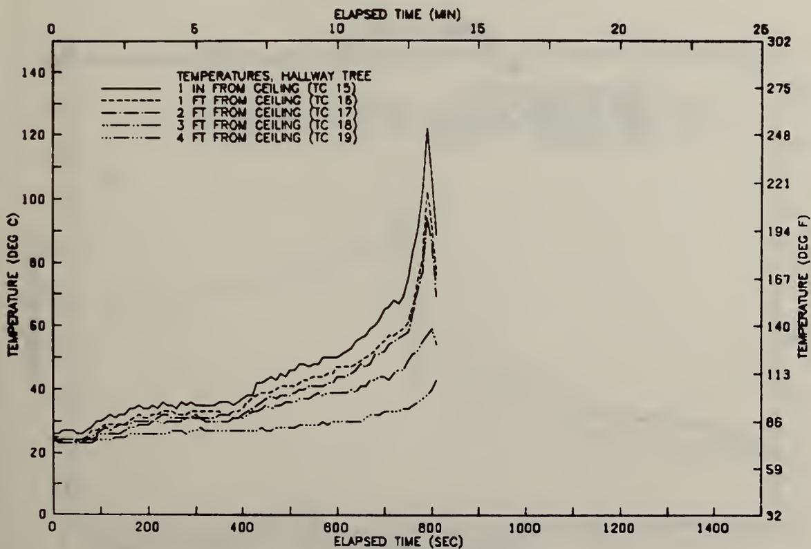
FIGURE A72 VERTICAL TEMP. PROFILE IN HALLWAY—TEST 08
