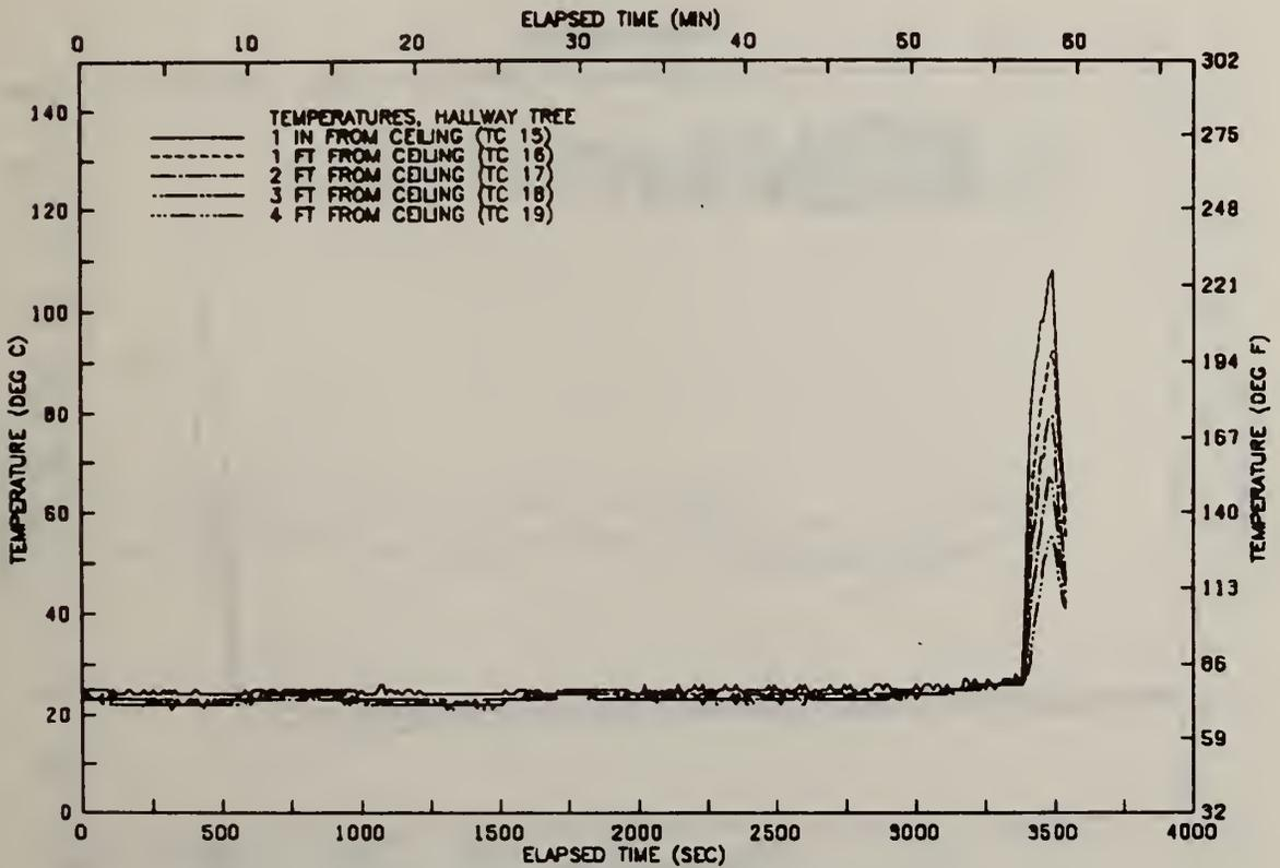
FIGURE A32 VERTICAL TEMP. PROFILE IN HALLWAY-TEST 04
