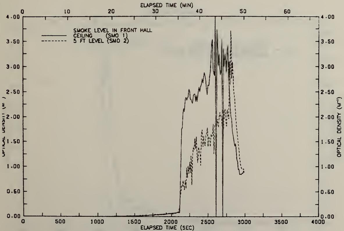
FIGURE B18 SMOKE LEVELS IN FRONT HALLWAY—TEST 15
