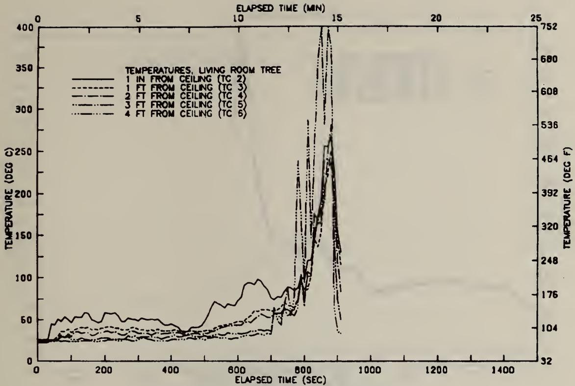
FIGURE A121 VERTICAL TEMP. PROFILE ABOVE CHAIR-TEST 13
