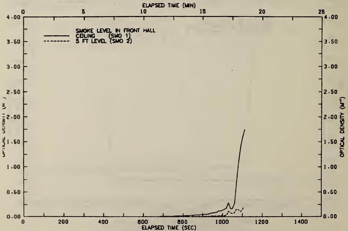
FIGURE B128 SMOKE LEVELS IN FRONT HALLWAY—TEST 25
