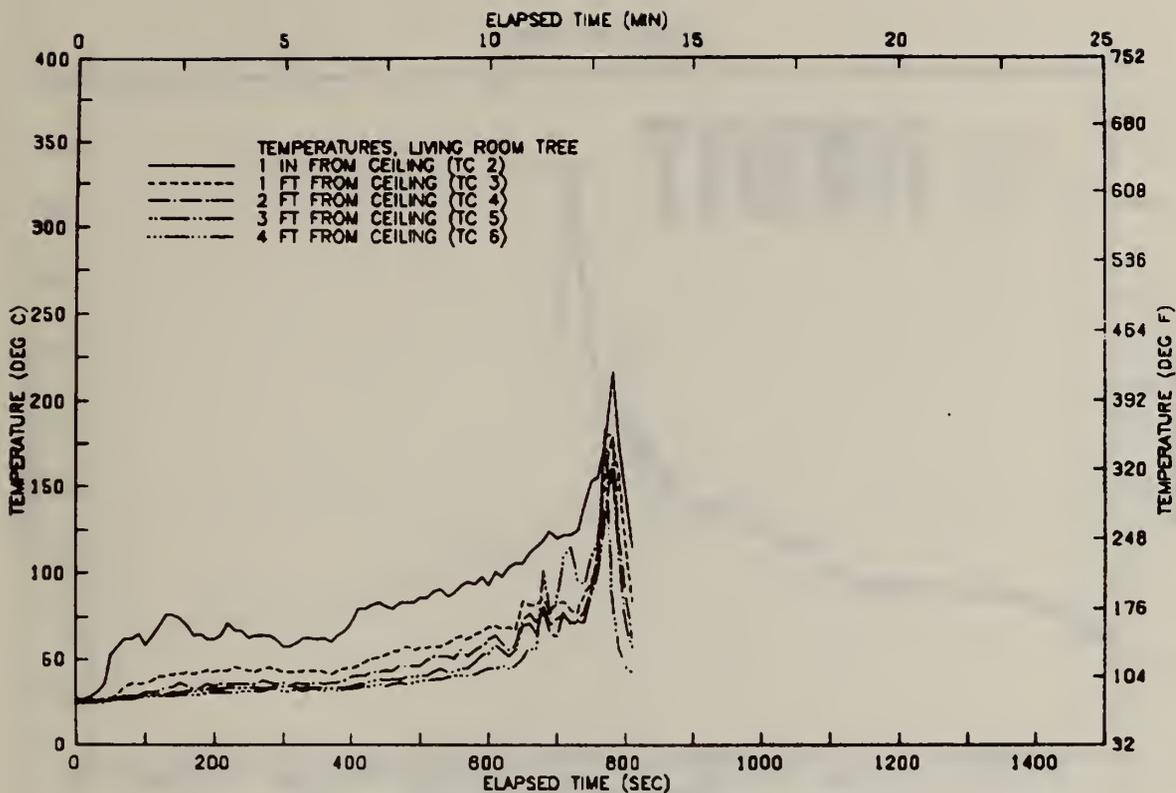
FIGURE A71 VERTICAL TEMP. PROFILE ABOVE CHAIR—TEST 08
