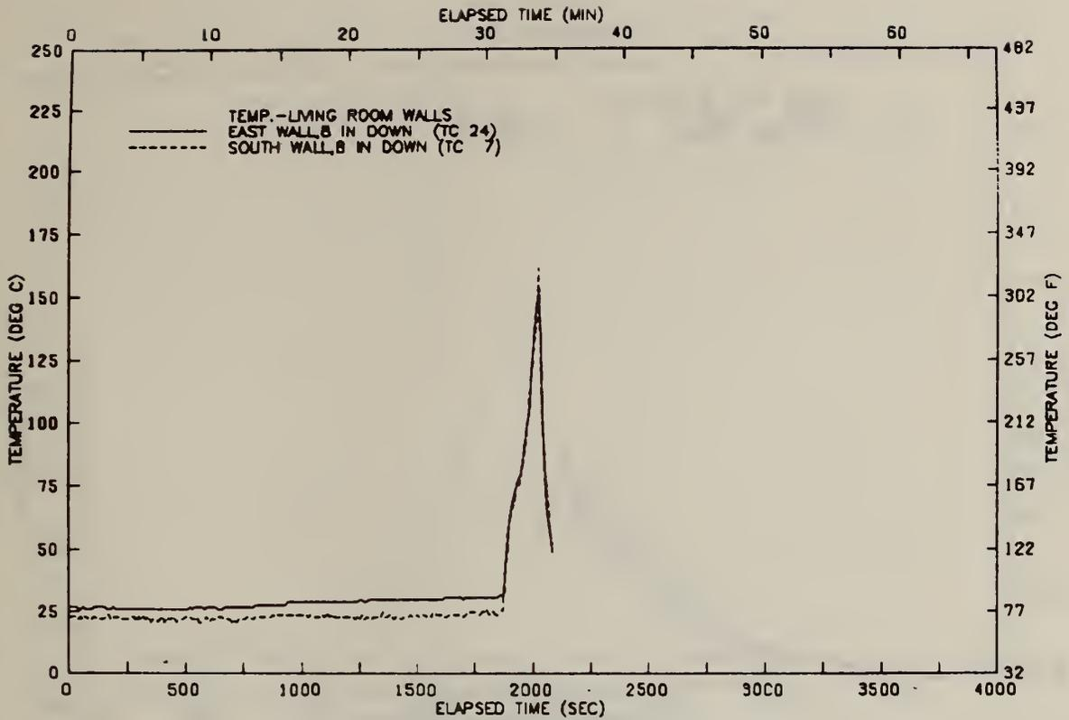
FIGURE A5 TEMPERATURE AT LIVING ROOM WALLS-TEST 01
