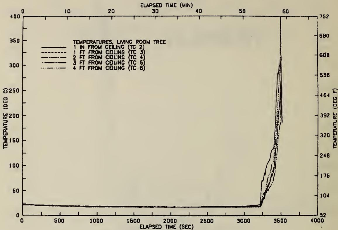
FIGURE B23 VERTICAL TEMP. PROFILE ABOVE CHAIR-TEST 16
