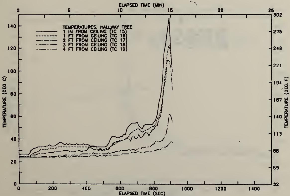
FIGURE A122 VERTICAL TEMP. PROFILE IN HALLWAY-TEST 13
