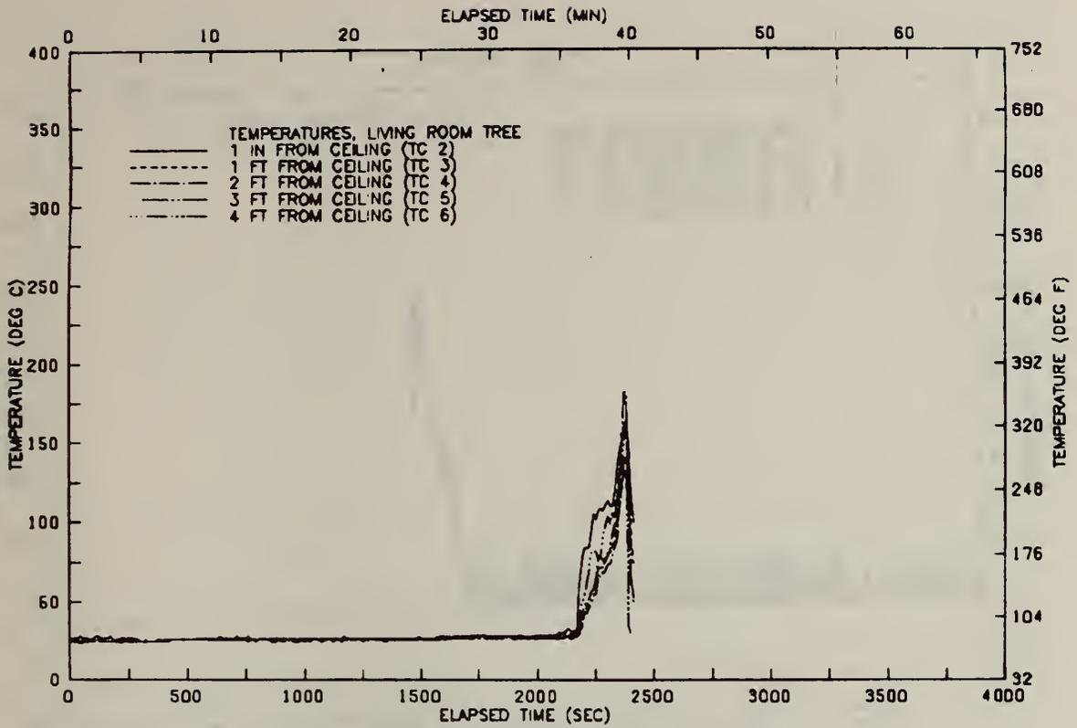
FIGURE A11 VERTICAL TEMP. PROFILE ABOVE CHAIR-TEST 02
