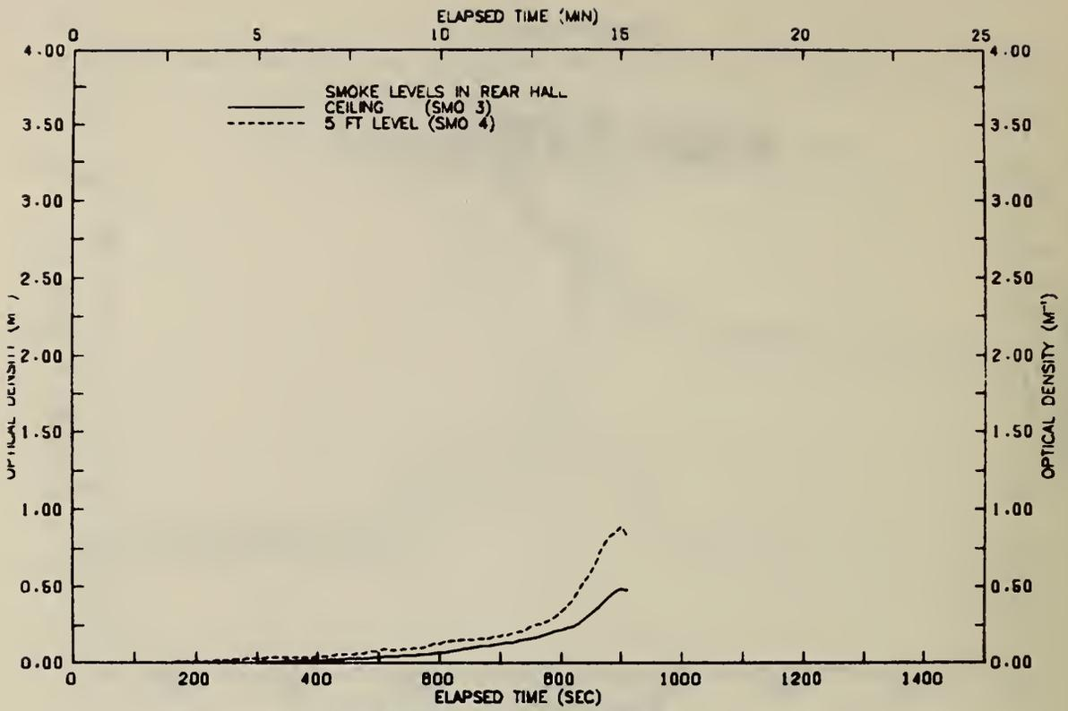
FIGURE B63 SMOKE LEVELS IN REAR HALLWAY-TEST 19
