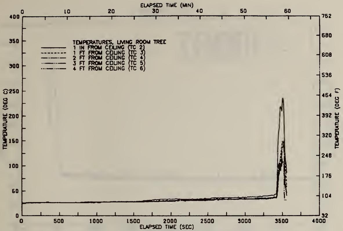
FIGURE A21 VERTICAL TEMP. PROFILE ABOVE CHAIR-TEST 03
