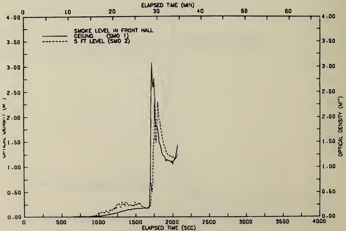
FIGURE B40 SMOKE LEVELS IN FRONT HALLWAY—TEST 17
