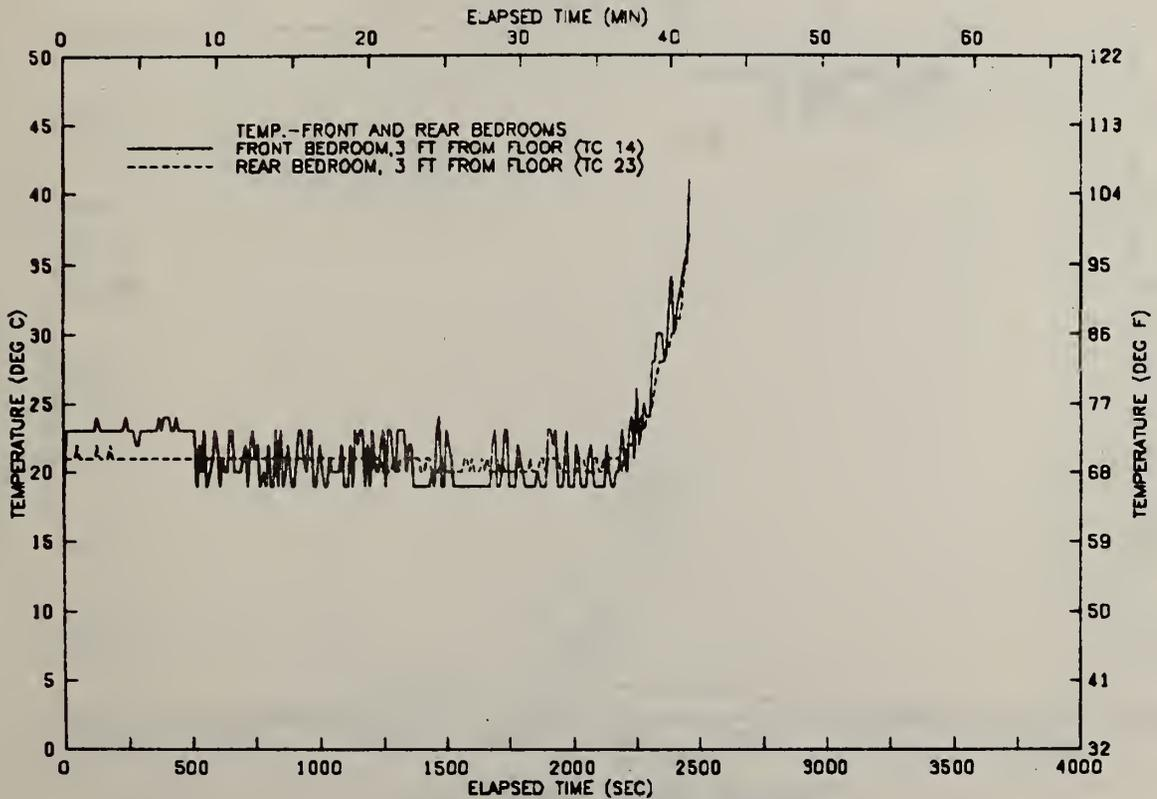
FIGURE B6 TEMP. IN FRONT AND REAR BEDROOMS—TEST 14
