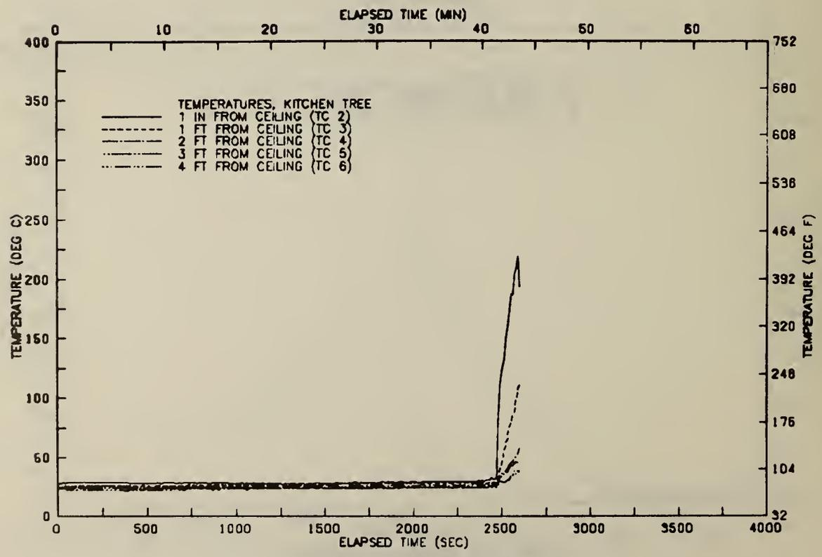
FIGURE B100 VERTICAL TEMP. PROFILE IN KITCHEN-TEST 23
