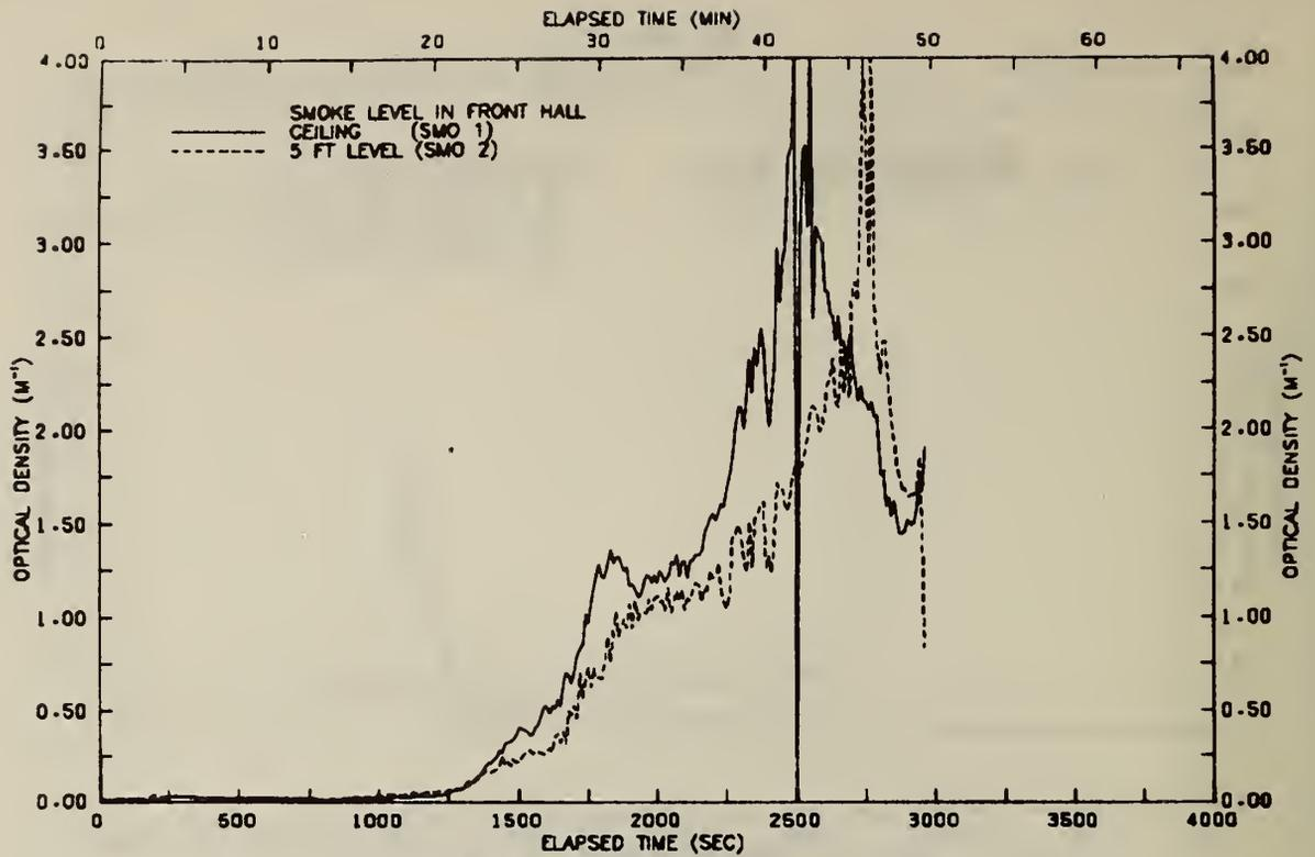
FIGURE A47 SMOKE LEVELS IN FRONT HALLWAY—TEST 05
