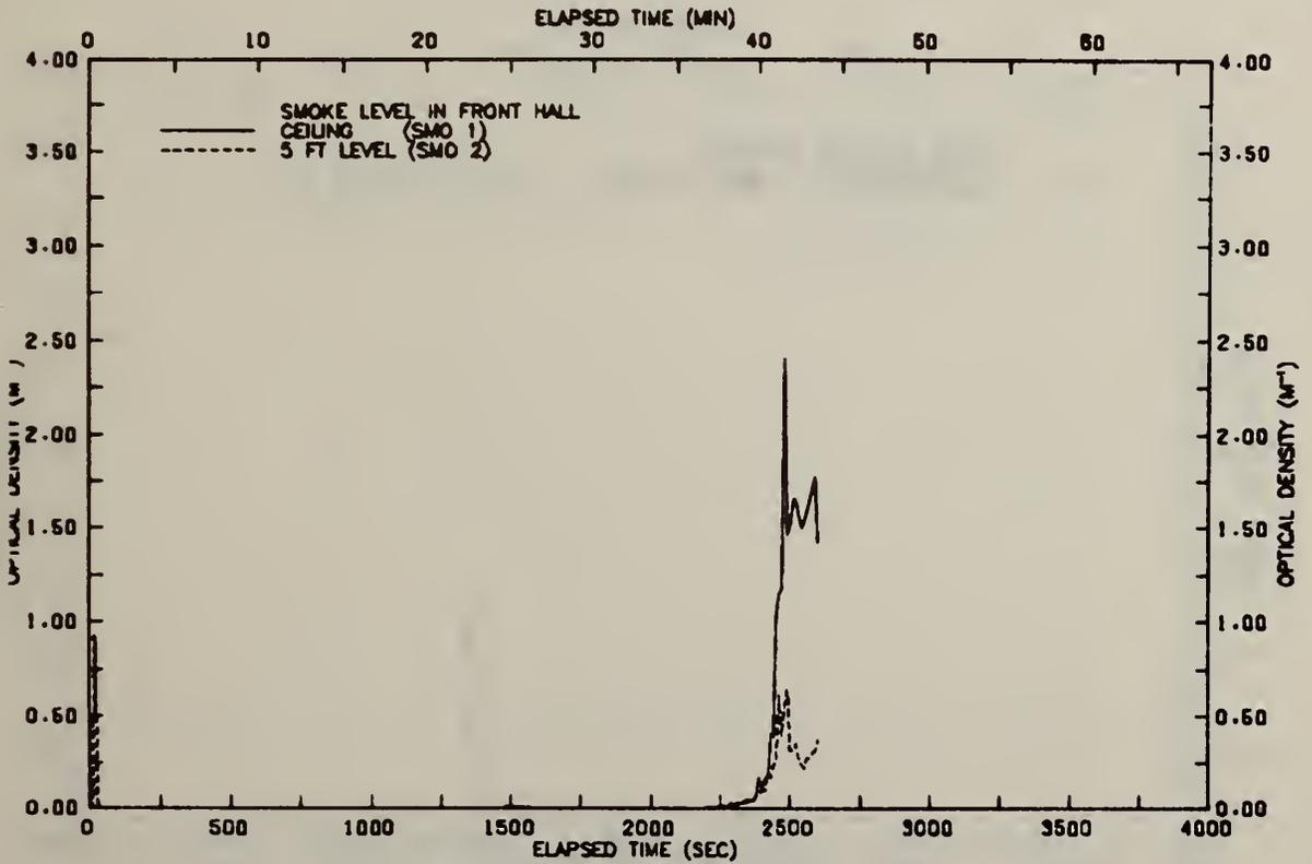
FIGURE B106 SMOKE LEVELS IN FRONT HALLWAY—TEST 23
