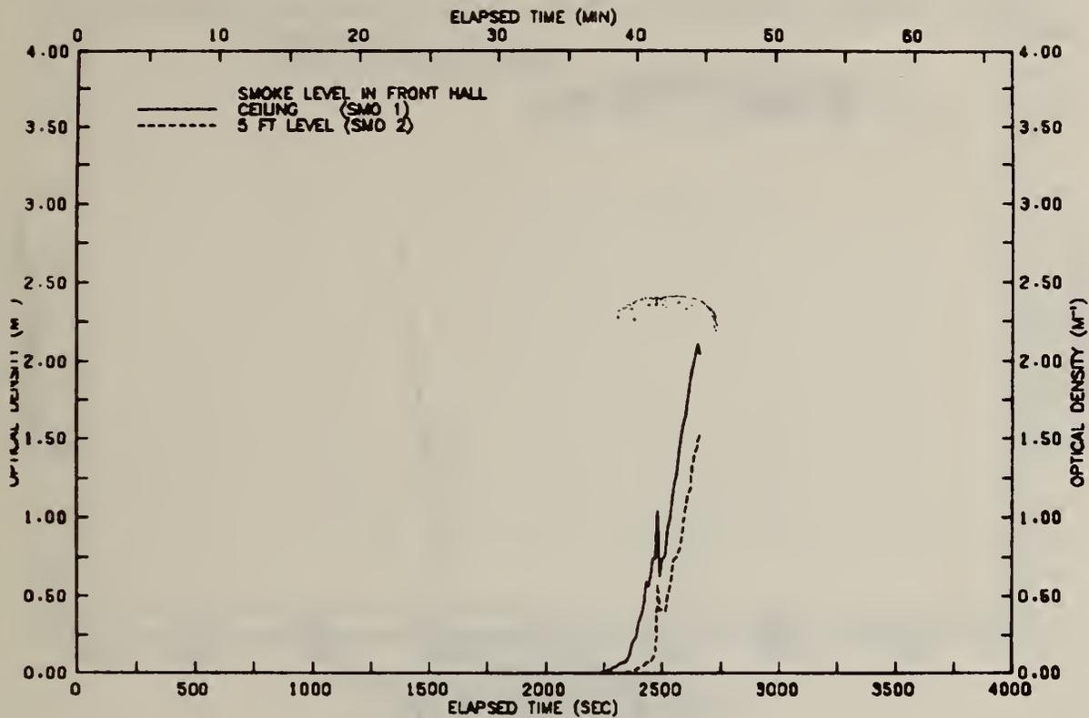
FIGURE B117 SMOKE LEVELS IN FRONT HALLWAY-TEST 24
