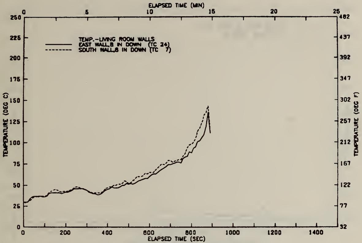
FIGURE A115 TEMPERATURE AT LIVING ROOM WALLS—TEST 12
