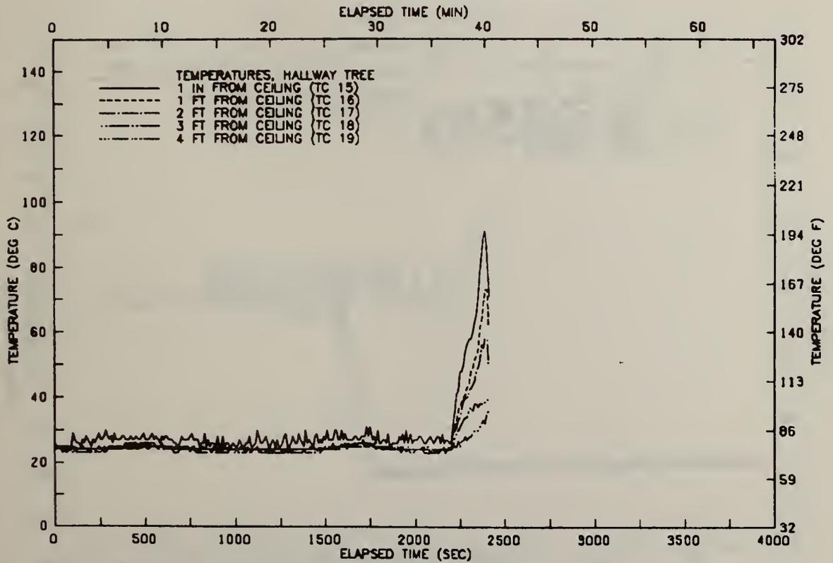
FIGURE A12 VERTICAL TEMP. PROFILE IN HALLWAY-TEST 02
