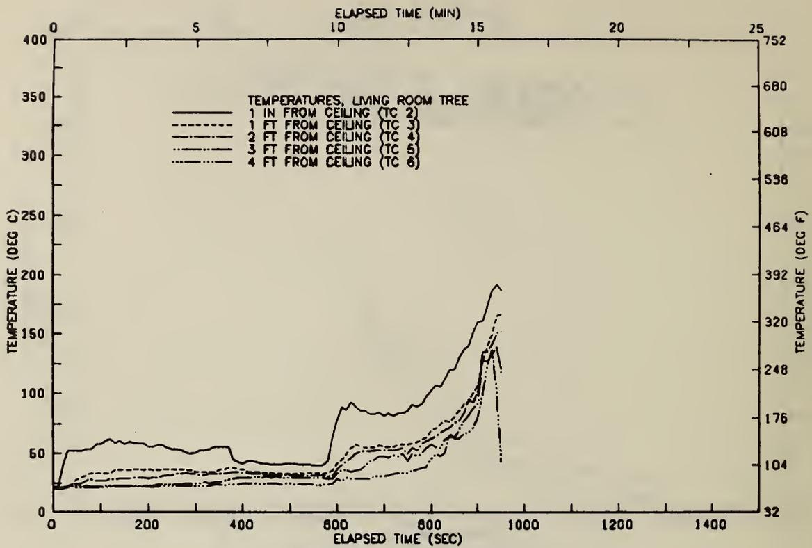
FIGURE B67 VERTICAL TEMP. PROFILE ABOVE CHAIR—TEST 20
