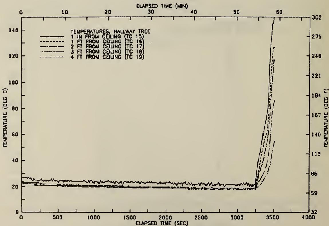
FIGURE B24 VERTICAL TEMP. PROFILE IN HALLWAY-TEST 16
