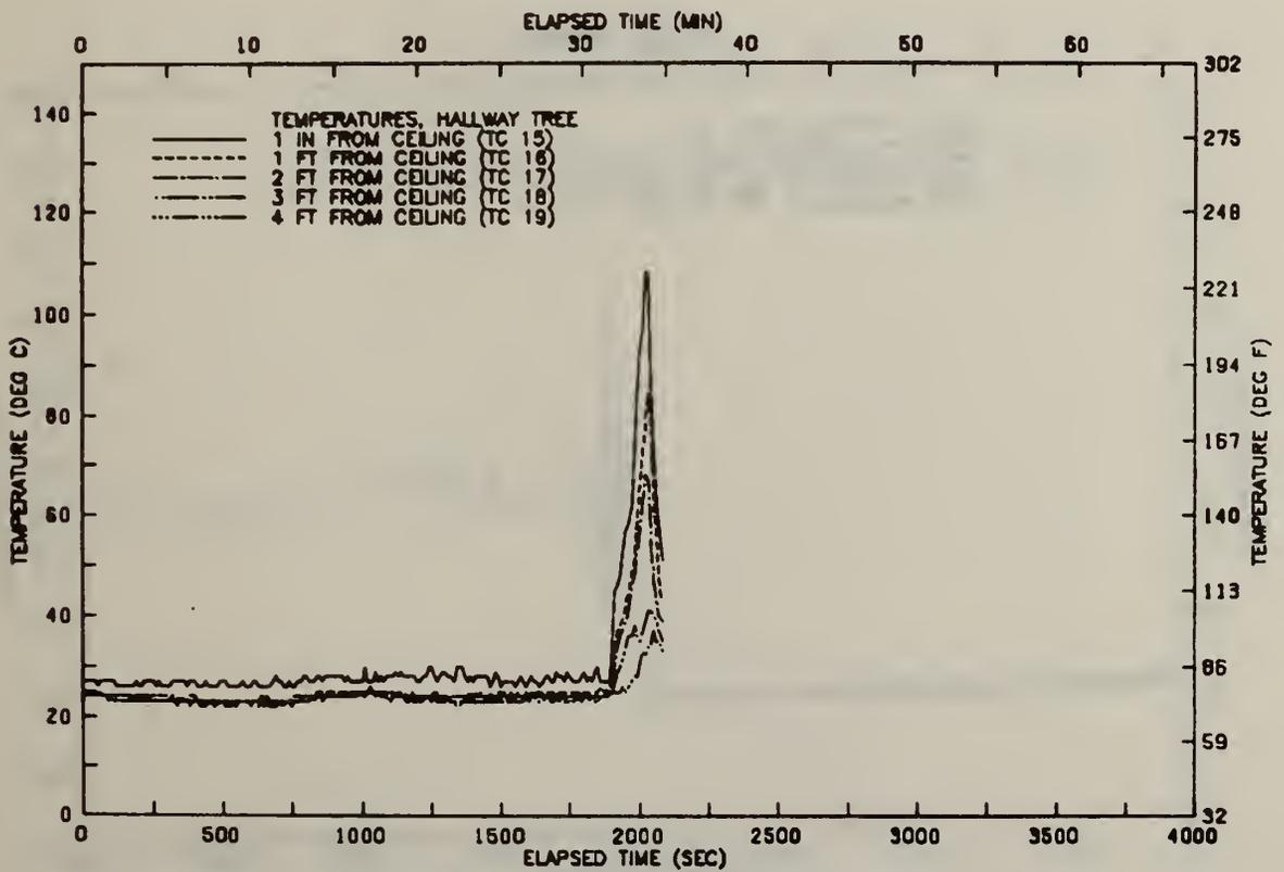
FIGURE A2 VERTICAL TEMP. PROFILE IN HALLWAY-TEST 01
