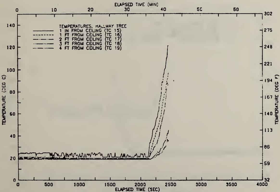
FIGURE B2 VERTICAL TEMP. PROFILE IN HALLWAY-TEST 14
