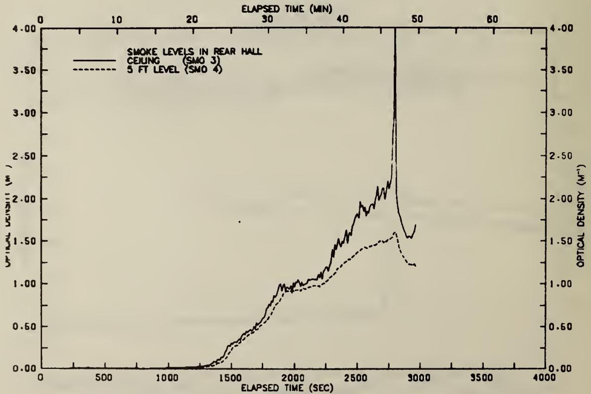
FIGURE A48 SMOKE LEVELS IN REAR HALLWAY—TEST 05
