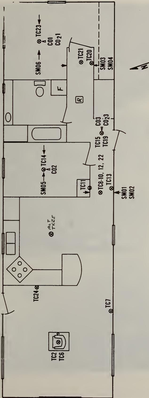
Figure 4. Mobile home floor plan and instrumentation locations
