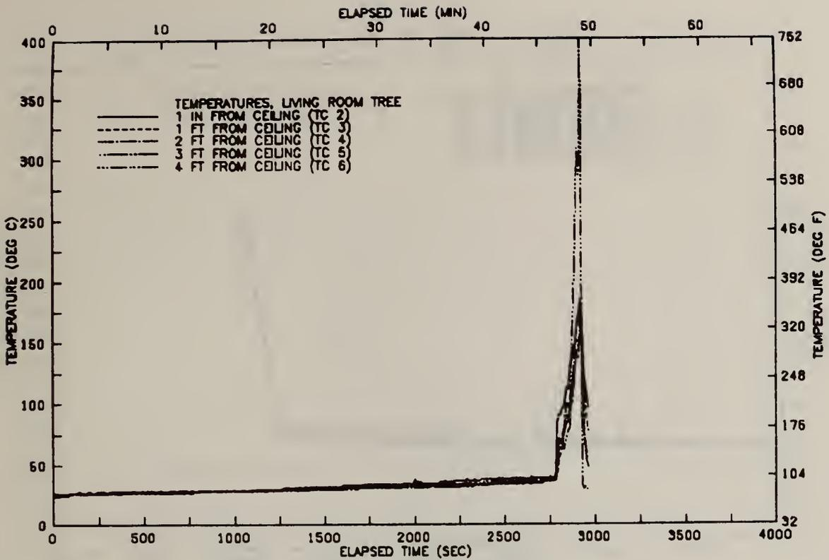
FIGURE A41 VERTICAL TEMP. PROFILE ABOVE CHAIR-TEST 05
