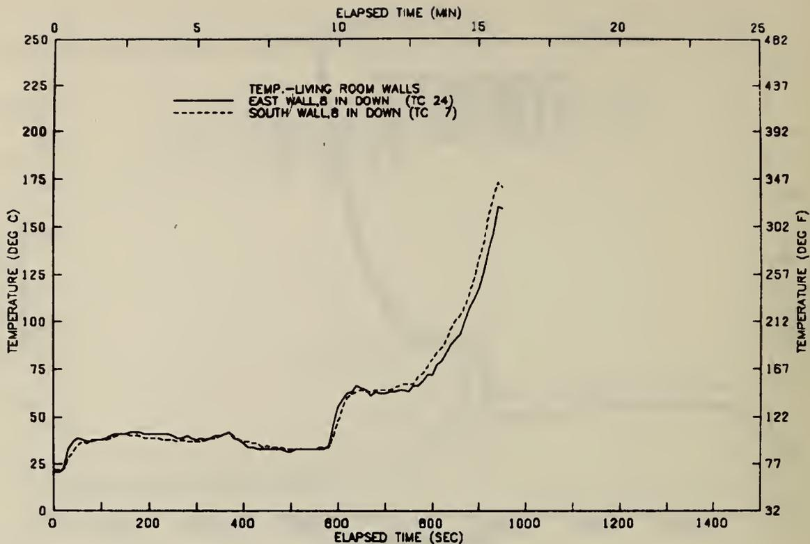
FIGURE B71 TEMPERATURE AT LIVING ROOM WALLS—TEST 20
