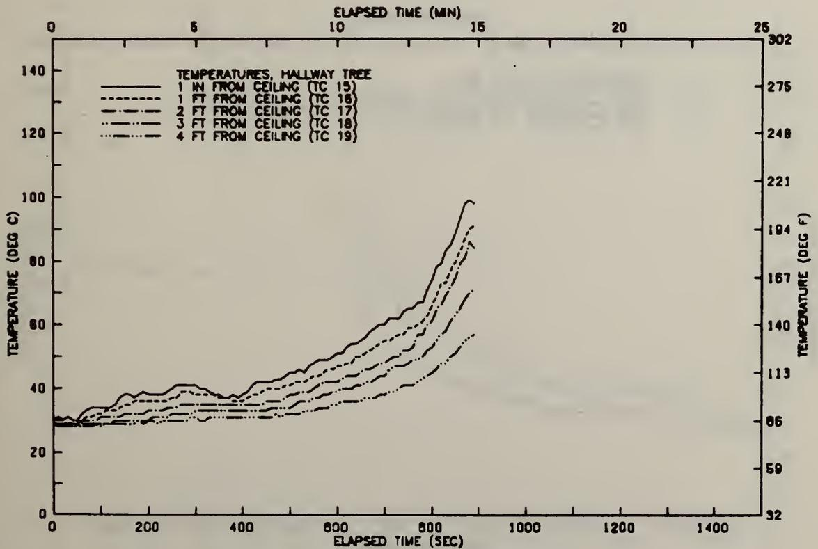
FIGURE A112 VERTICAL TEMP. PROFILE IN HALLWAY-TEST 12
