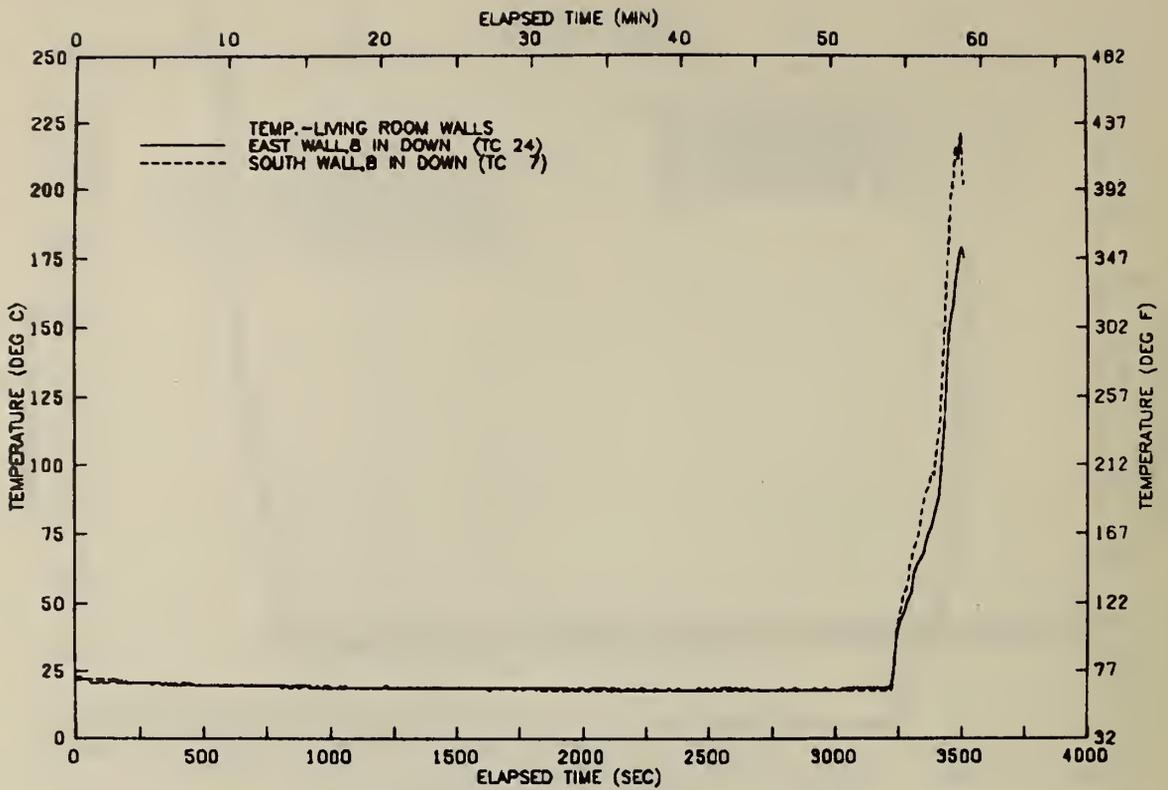
FIGURE B27 TEMPERATURE AT LIVING ROOM WALLS - TEST 16
