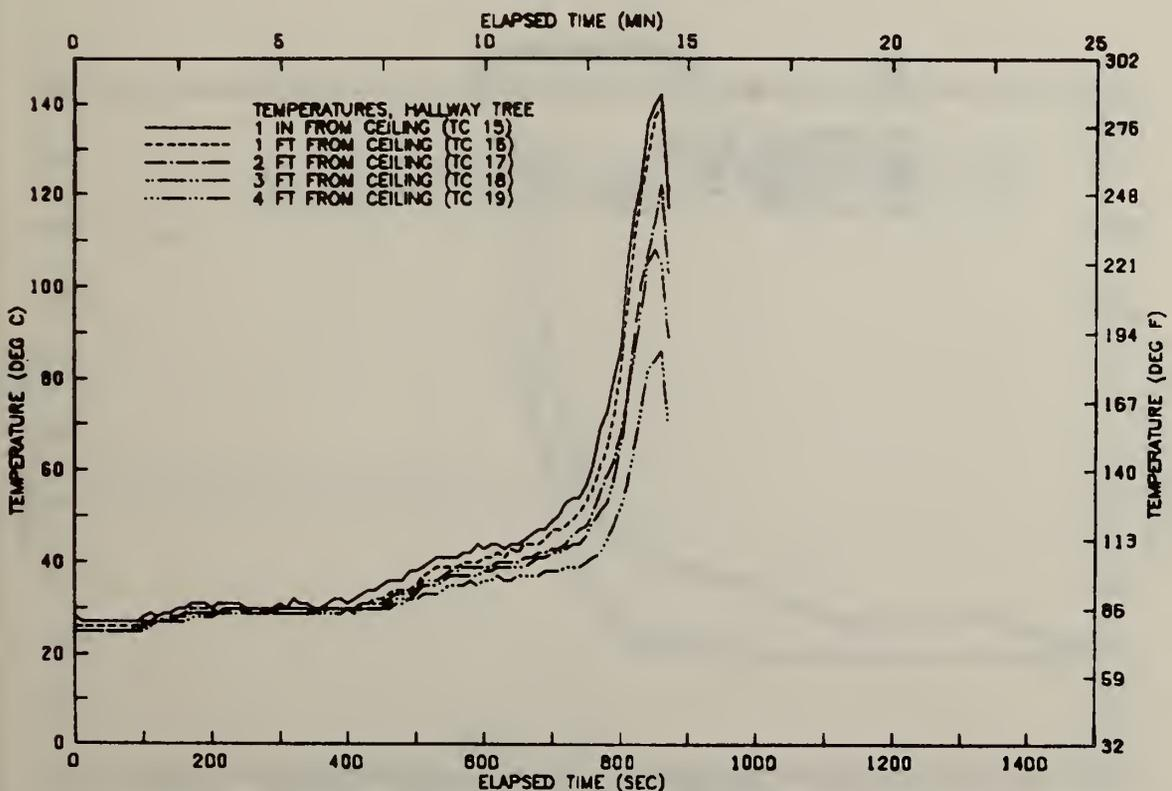
FIGURE A102 VERTICAL TEMP. PROFILE IN HALLWAY—TEST 11
