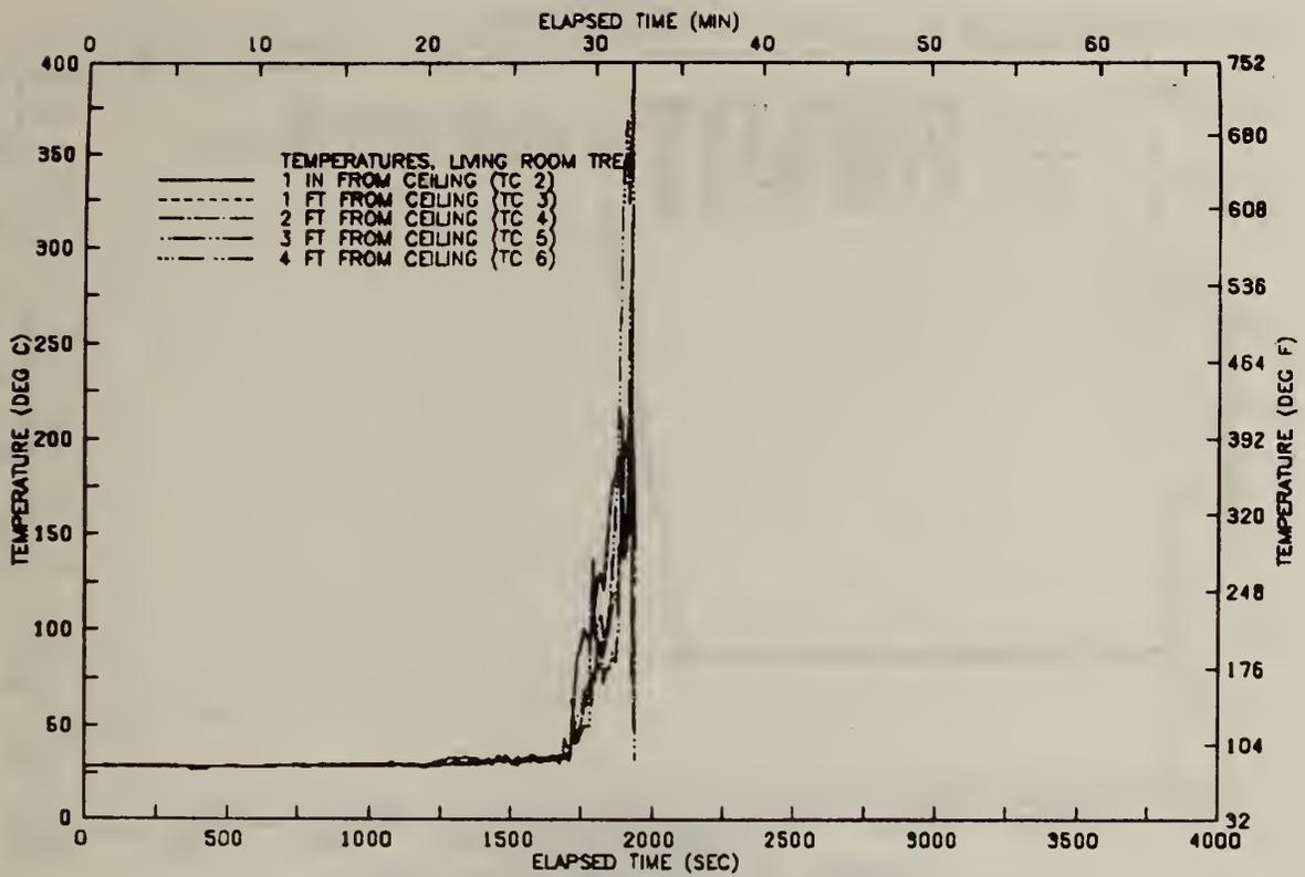
FIGURE A61 VERTICAL TEMP. PROFILE ABOVE CHAIR-TEST 07
