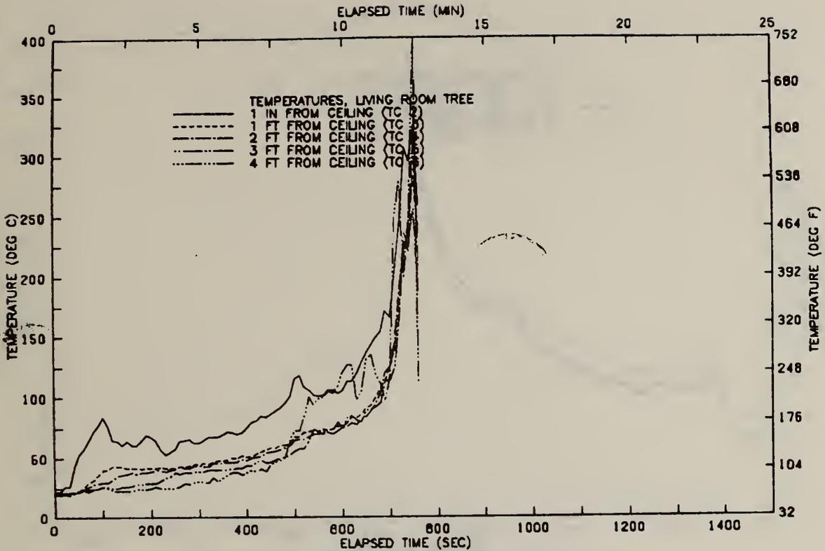
FIGURE B89 VERTICAL TEMP. PROFILE ABOVE CHAIR—TEST 22
