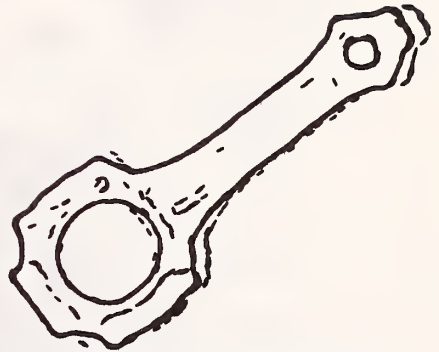
Result of applying Hueckel edge operator on Fig. 30 Output: 400 edge points containing location, direction, and average intensity on both sides.
