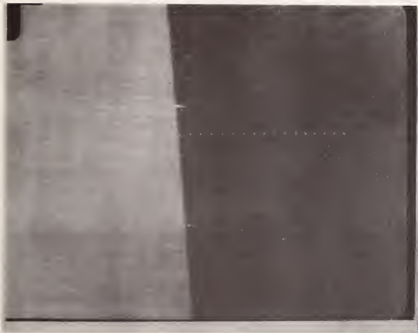
Figure D-2. Photomicrograph of silicon surface beveled with 0.1- \mu\text{m} diamond against ground glass. Top surface was polished with 0.5- \mu\text{m} diamond against soft cloth.
