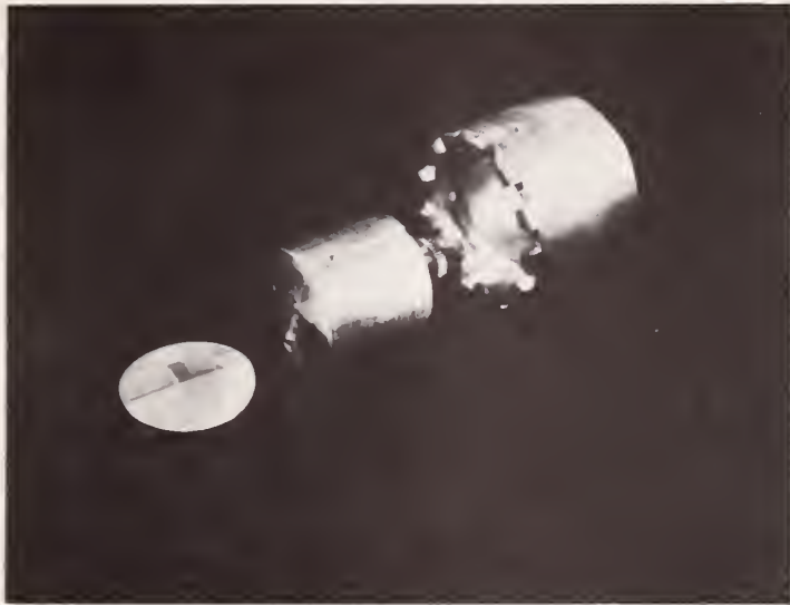
Figure 3-1. Silicon chip mounted on beveling block with piston and collar used in beveling procedure.
