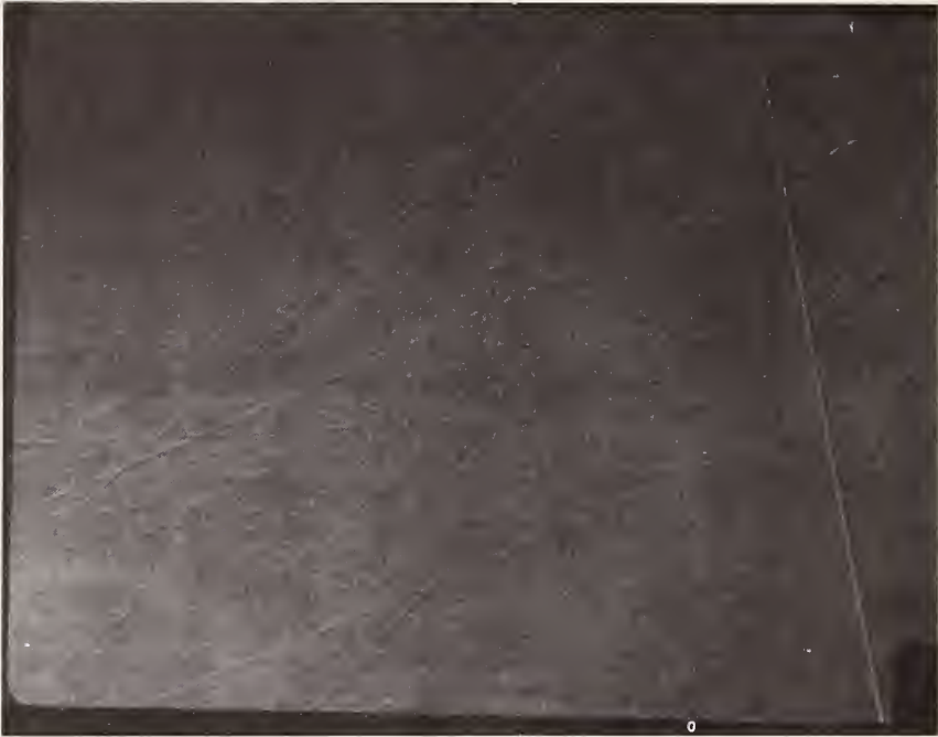
Figure C-11. Photomicrograph of silicon slice after polishing with 0.5- \mu\text{m} diamond (220X magnification).
