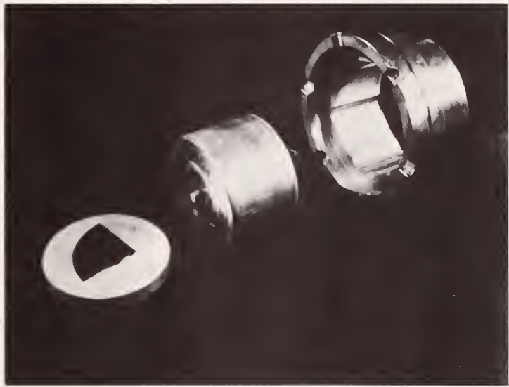
Figure C-1. Mounting block, piston, and collar used for top surface polishing.
