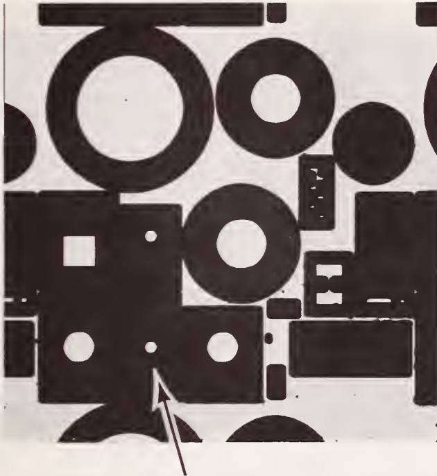
Figure A-2. Photomicrograph of plasma-etched mesas. The arrow indicates a particular device which is enlarged in figure A-3. See text for discussion of details.
