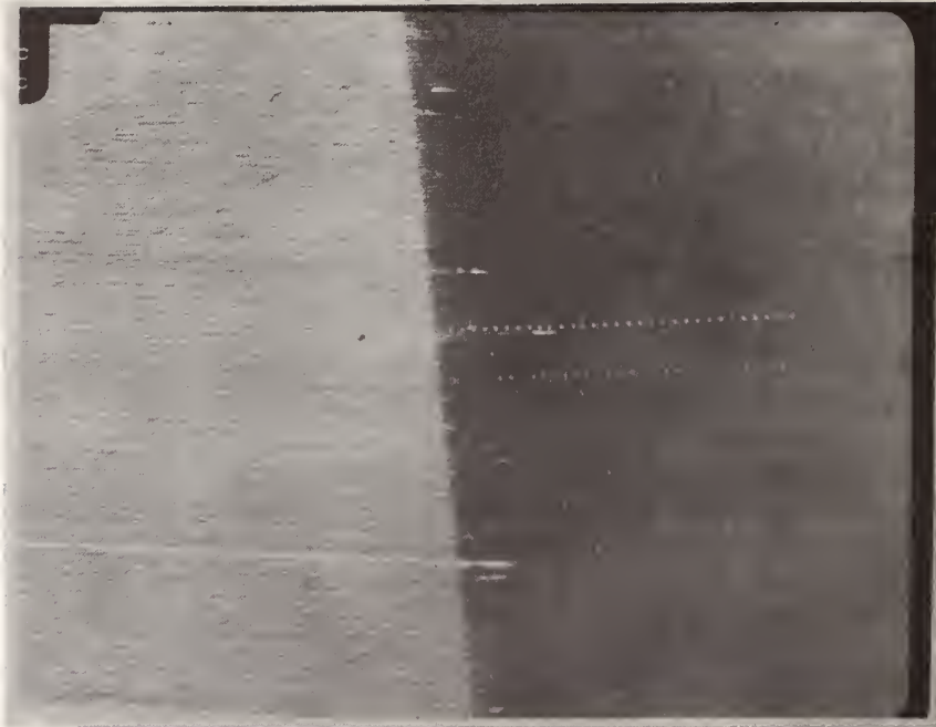
Figure D-1. Photomicrograph of silicon specimen beveled with 0.5- \mu\text{m} diamond against ground glass. Top surface was polished with 0.5- \mu\text{m} diamond against soft cloth.
