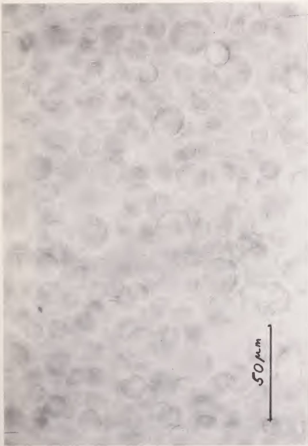
Fig. 10. a,b,c. These three transmitted light optical micrographs depict the same area of the wall of an intra-aortic balloon (polyurethane-polydimethyl siloxane elastomer). The inner face ("substrate-side") of the wall is facing upwards. In Fig. 10a, above, the microscope was focused on that face as closely as could be judged. In Figs. 10b,c the microscope was focused at slightly increasing depths below, but still close to the inner face of the balloon. Circular features may be seen in all those micrographs. It is evident from the overlapping between these features that they are not coplanar.
