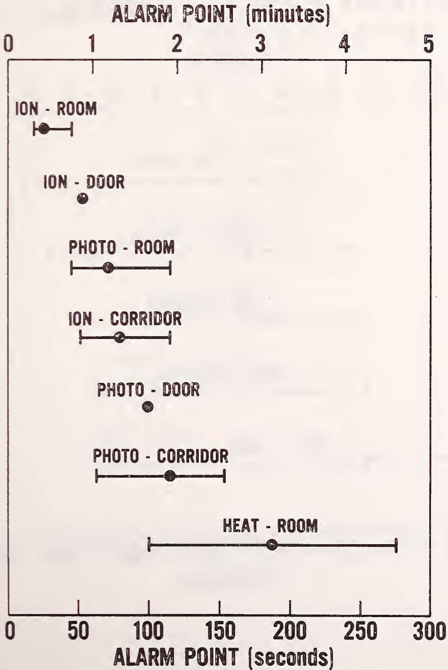
Figure 6. Detector alarm times
