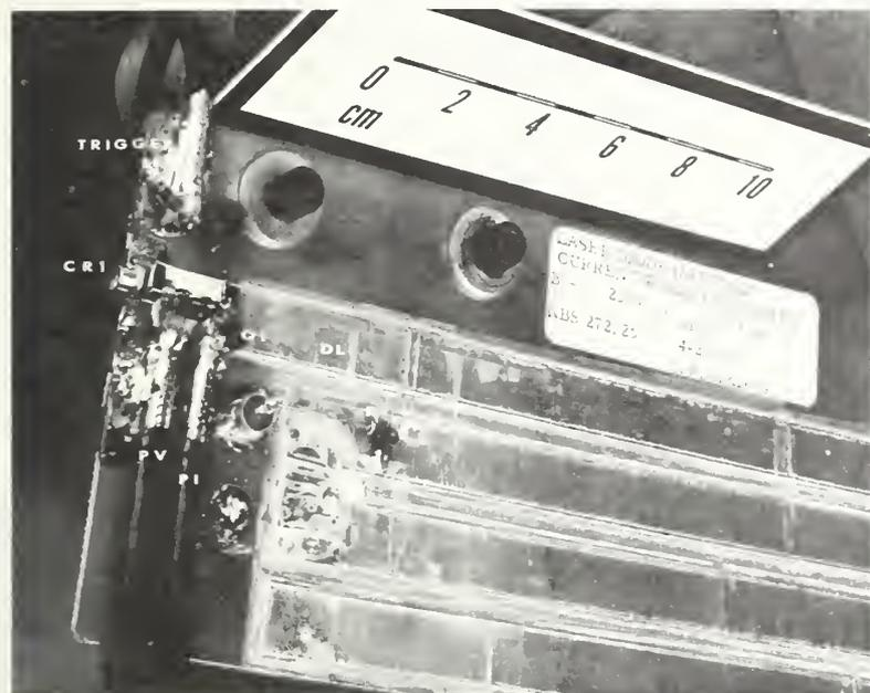
FIG. 2. Photograph of GaAs laser diode pulse generator.
