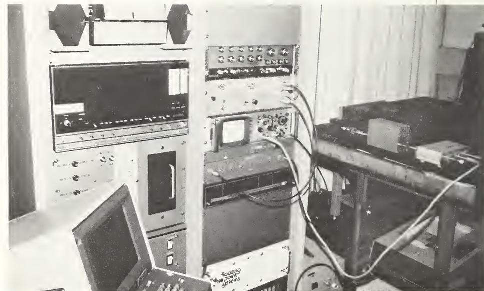
Figure 5. The NBS Automatic Pulse Measurement System.
