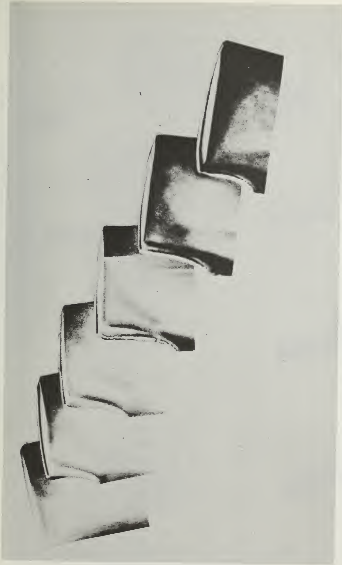
Figure 4. Artist's rendition showing blade trailing edge damage.
