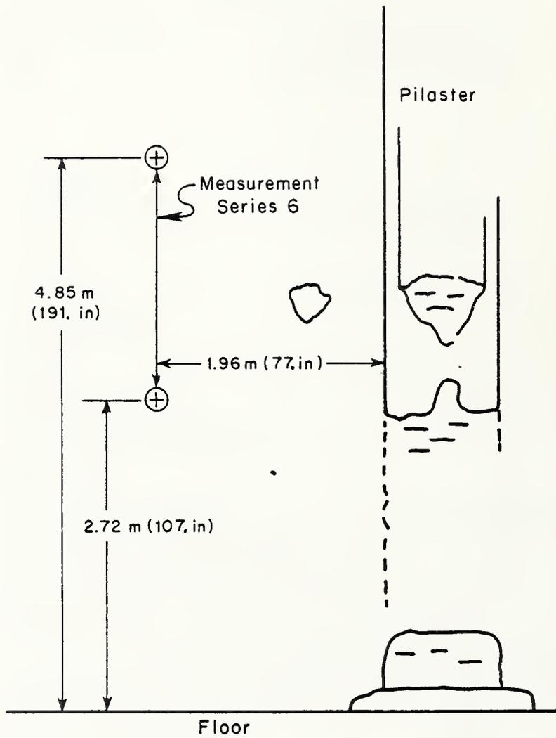
Figure 12. West nave wall position of measurement series 6. See figure 3 for the general location of measurement series 6.
