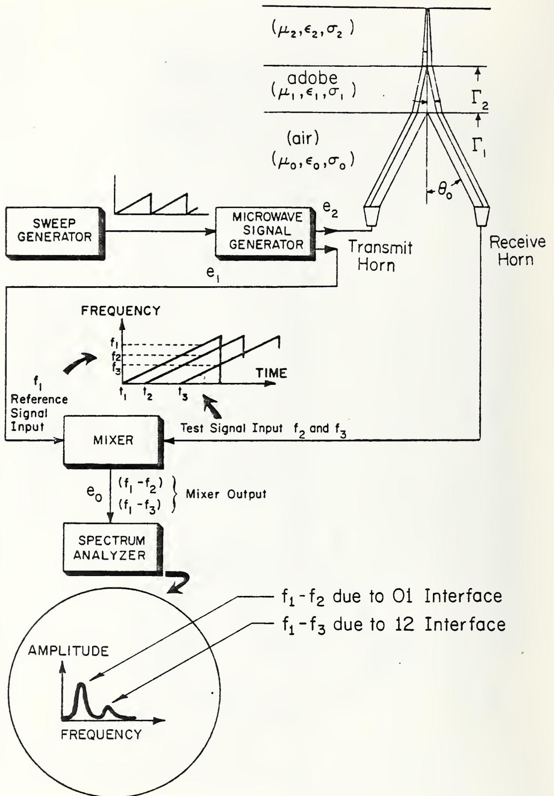
Figure 5. Block diagram of FM-CW electromagnetic system.
