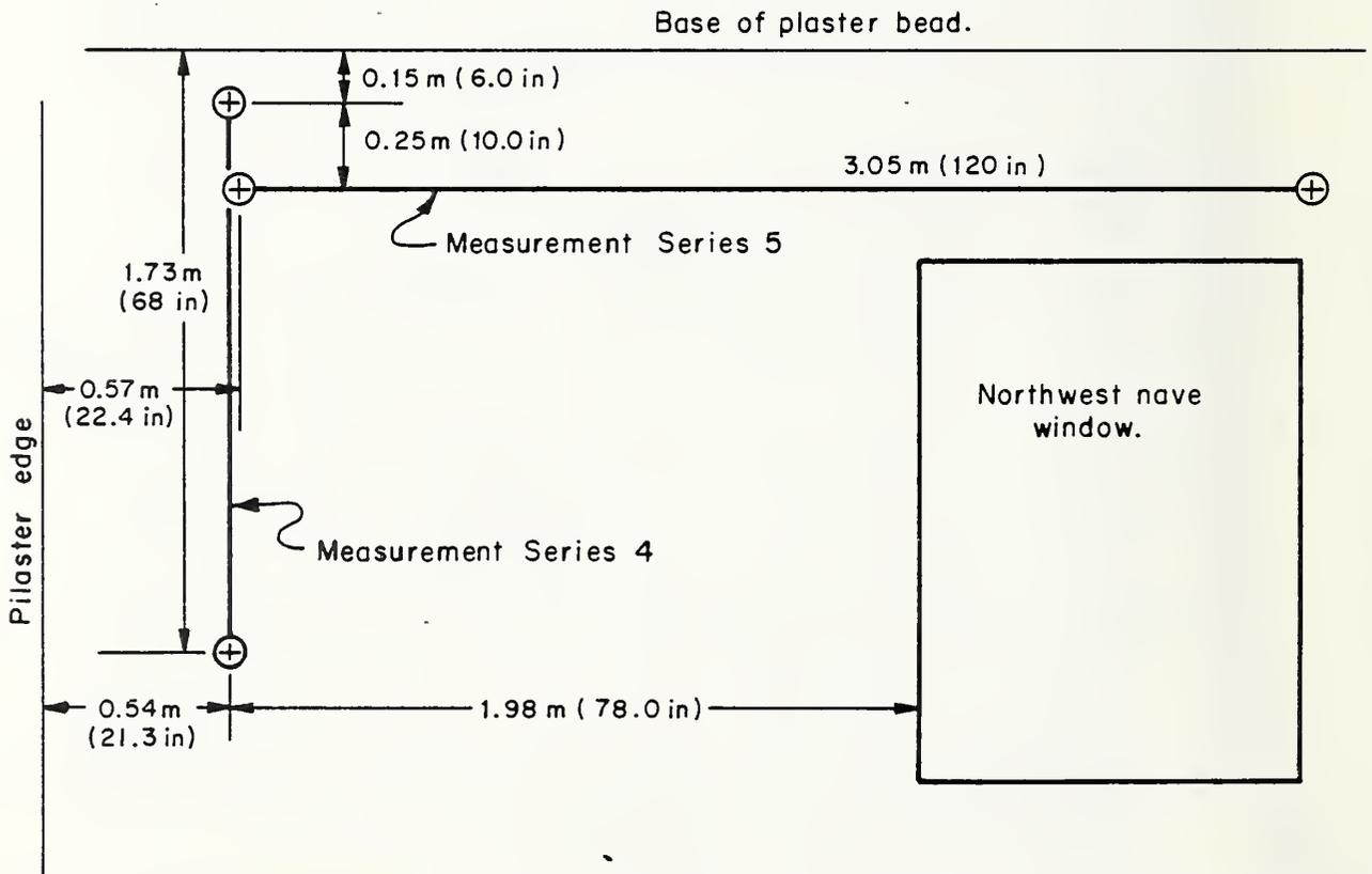
Figure 10. Northwest nave wall measurement positions of measurement series 4 and series 5. See figure 3 for the general location of these measurements.
