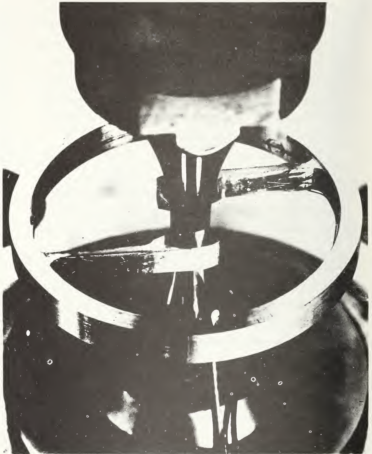
Figure 2 Diametral Strain Extensometer
