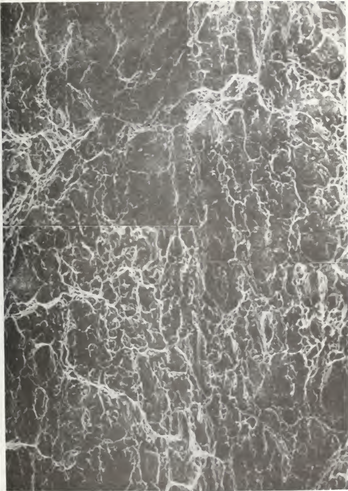
Figure 11. SEM photomicrograph of the fracture surface of a 76 K Charpy V impact specimen from an E316 weldment that was deliberately sensitized at 675°C for 24 hours (550X).
