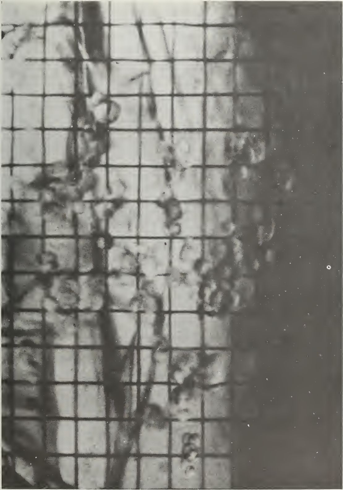
Figure 6. Aged Slush Oxygen Particles, Aged 24 Hours, Grid Size is 2mm square.
