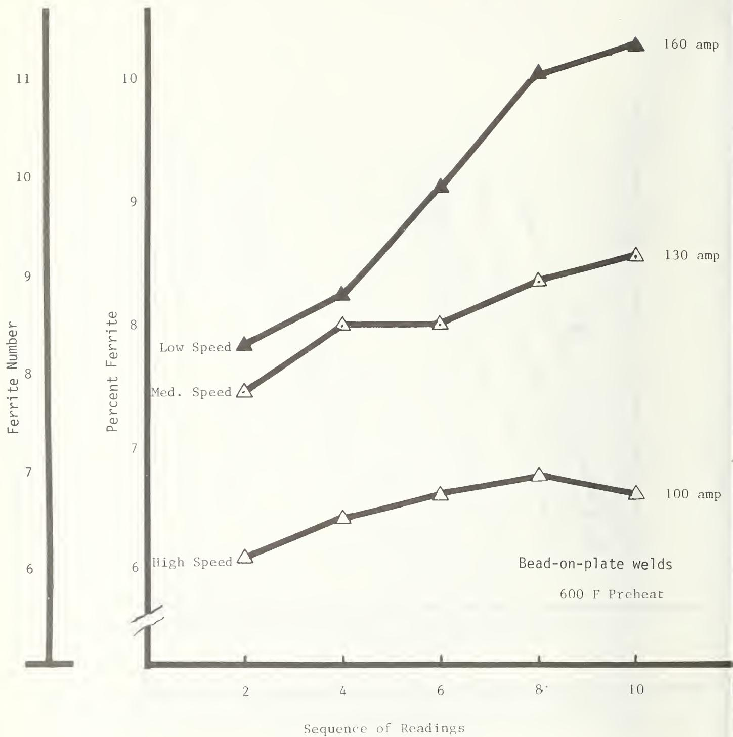
FIGURE 8. Ferrite content as a function of position in the test plate for three heat input levels and 600<sup>o</sup>F preheat
