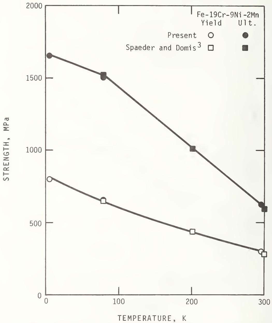
Figure 16. Strength property data for Fe-19Cr-9Ni-2Mn from the present study and from Spaeeder and Domis.<sup>3</sup>
