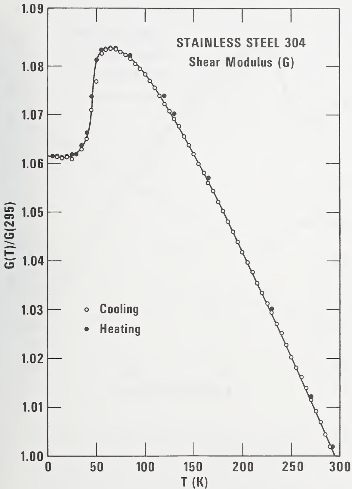
Figure 2. Temperature dependence of the shear modulus.
