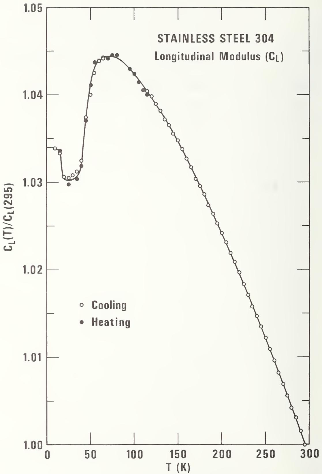
Figure 1. Temperature dependence of the longitudinal modulus.
