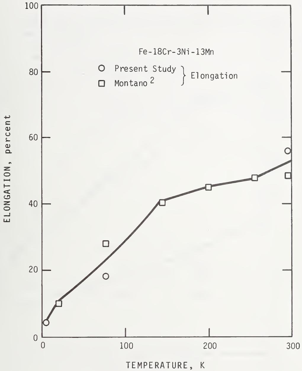
Figure 15. Elongation data for Fe-18Cr-3Ni-13Mn from the present study and from Montano.<sup>2</sup>
