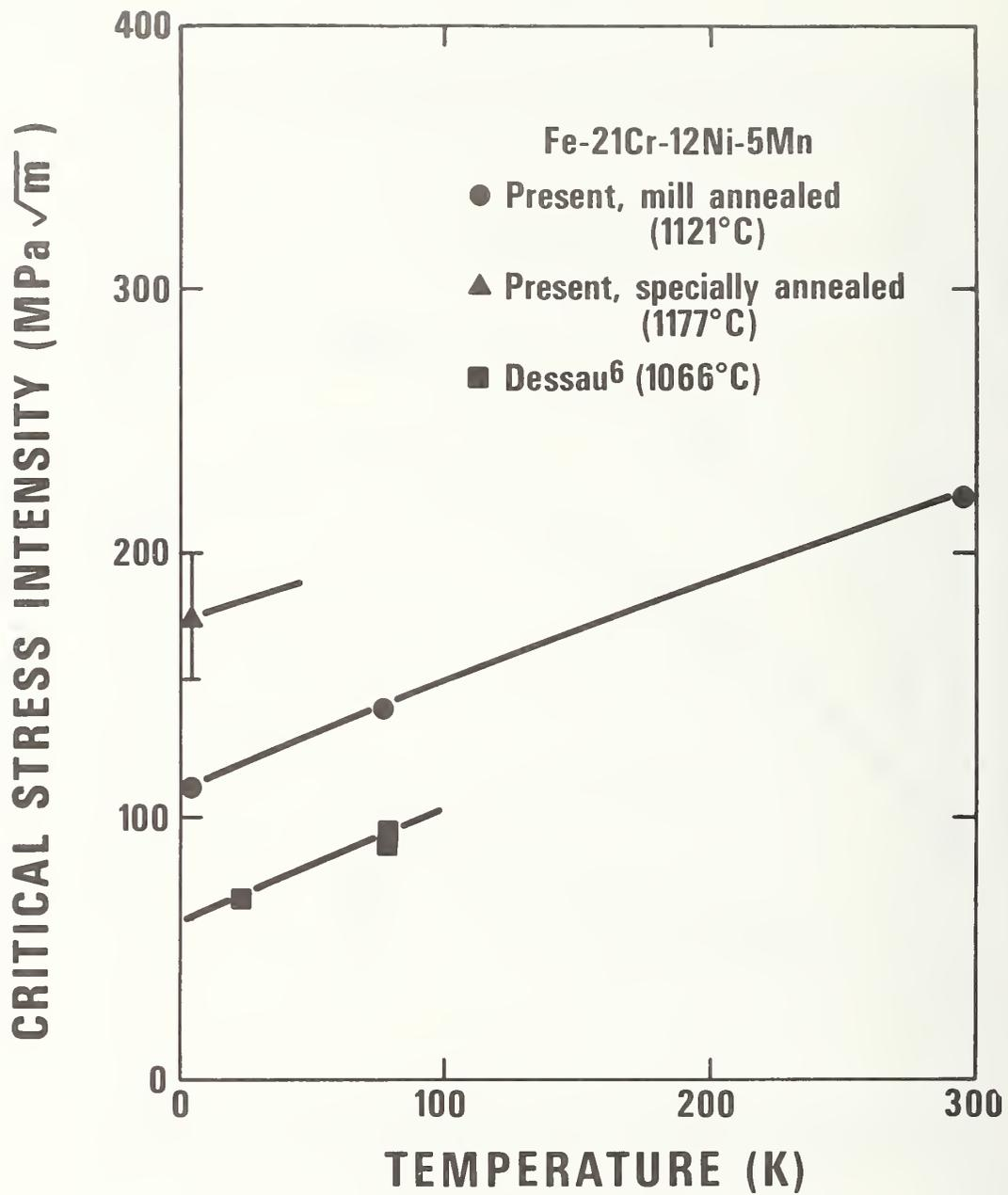
Figure 18. Three sets of toughness results for Fe-21Cr-12Ni-5Mn; two from the present study and one by Dessau.<sup>6</sup>
