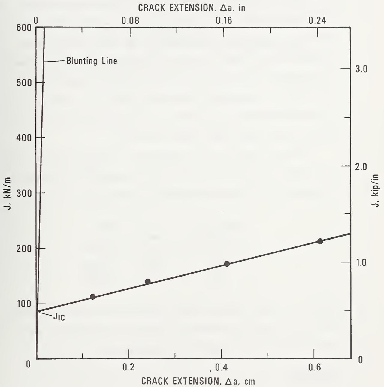
Figure 9 J-Integral Data at 4 K
