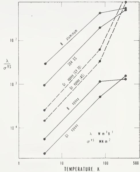
Fig. 1. Thermal conductivity to strength ratio for several uniaxial composites compared to welded stainless steel. From M. B. Kasen NBS.
