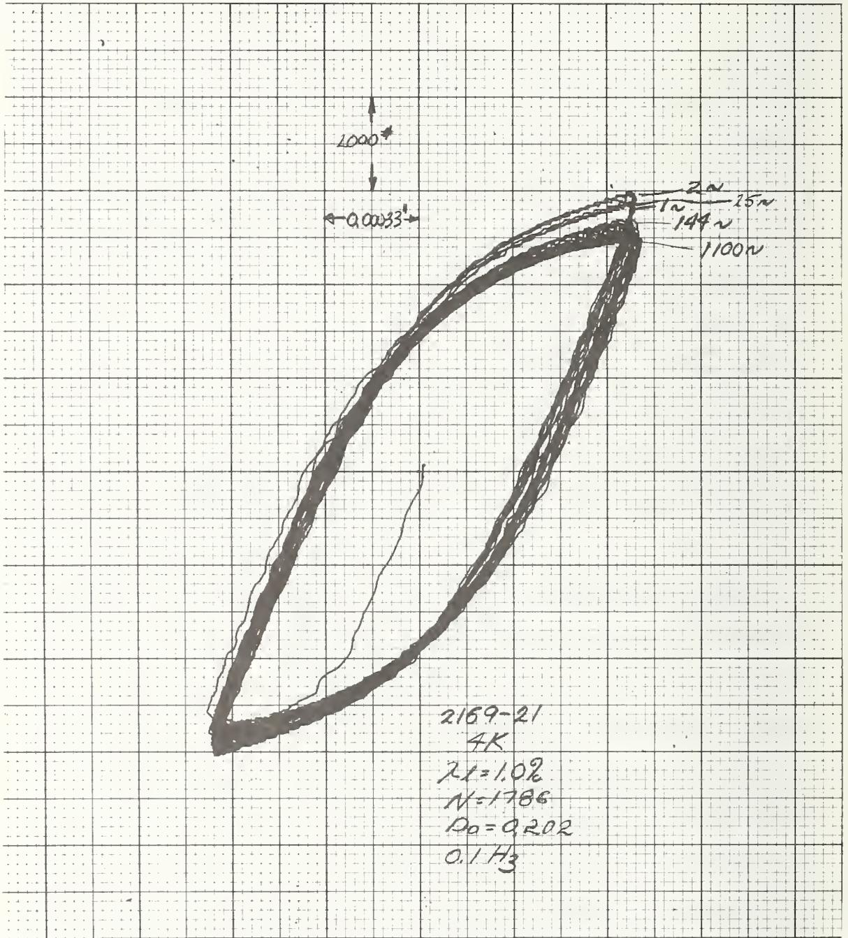
Figure 18 Load-Deflection Curve for Specimen 2169-21
