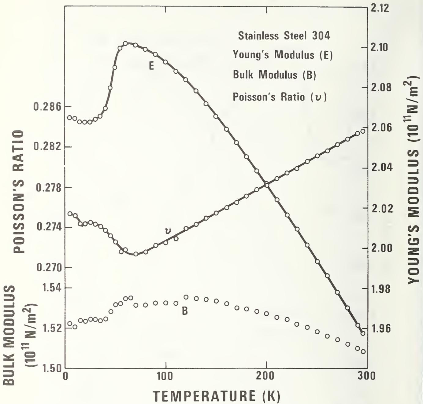
Figure 3. Temperature dependence of Young's modulus, the bulk modulus, and Poisson's ratio.
