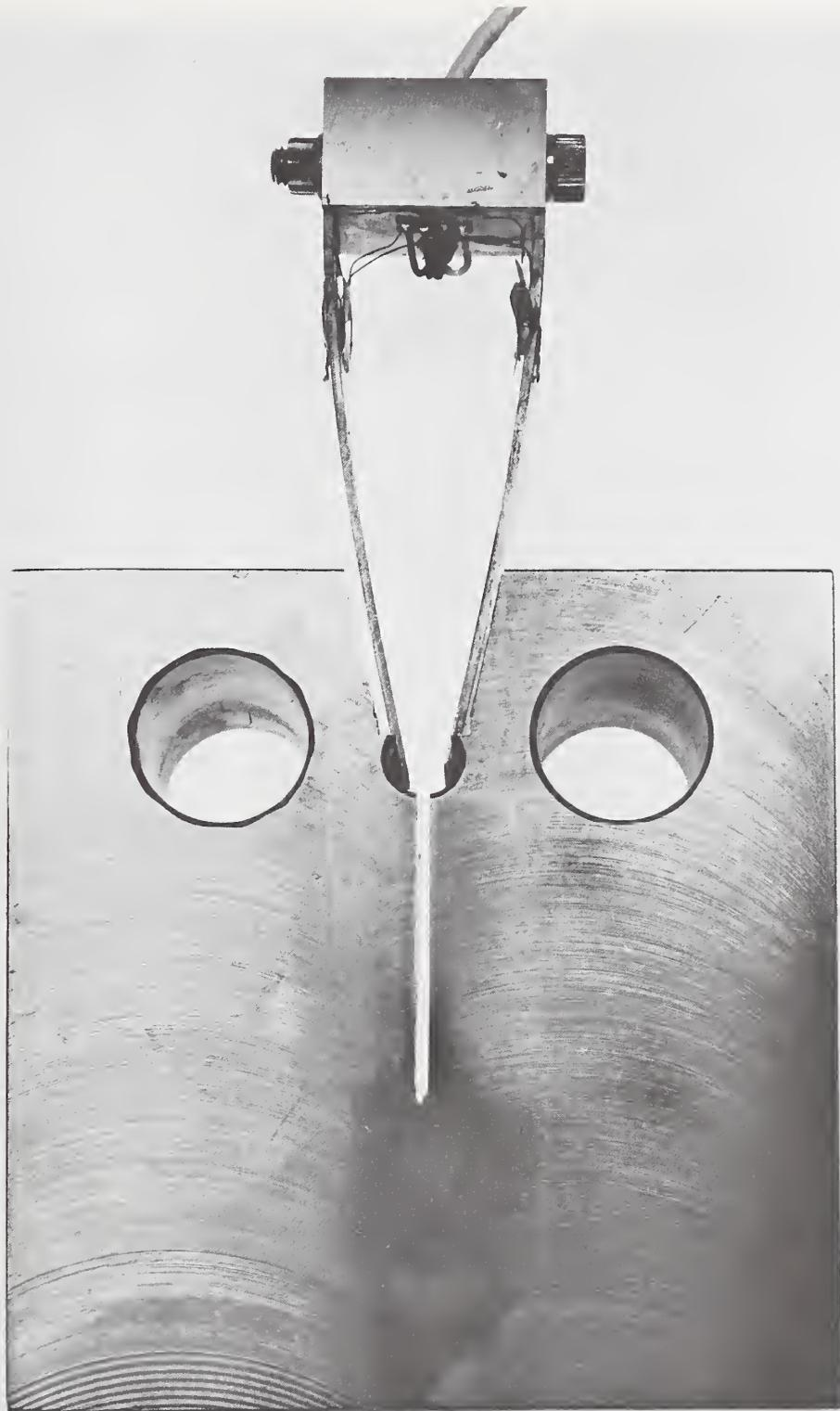
*Figure 2 Clip Gage Installed at the Loadline*
