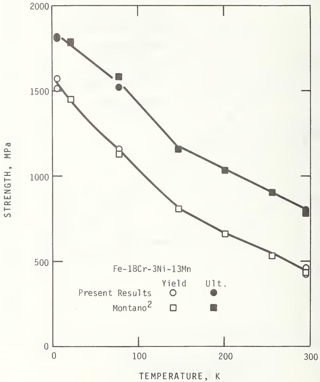
Figure 14. Strength property data for Fe-18Cr-3Ni-13Mn from the present study and from Montano.<sup>2</sup>
