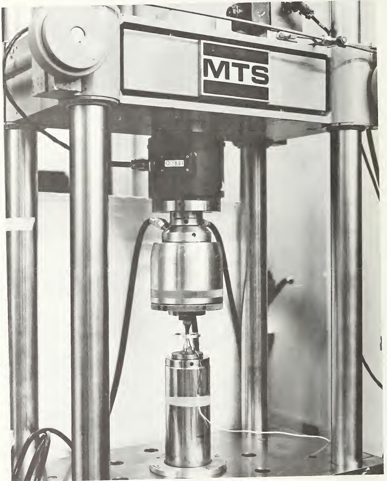
*Figure 3 Apparatus for 293 K Testing*
