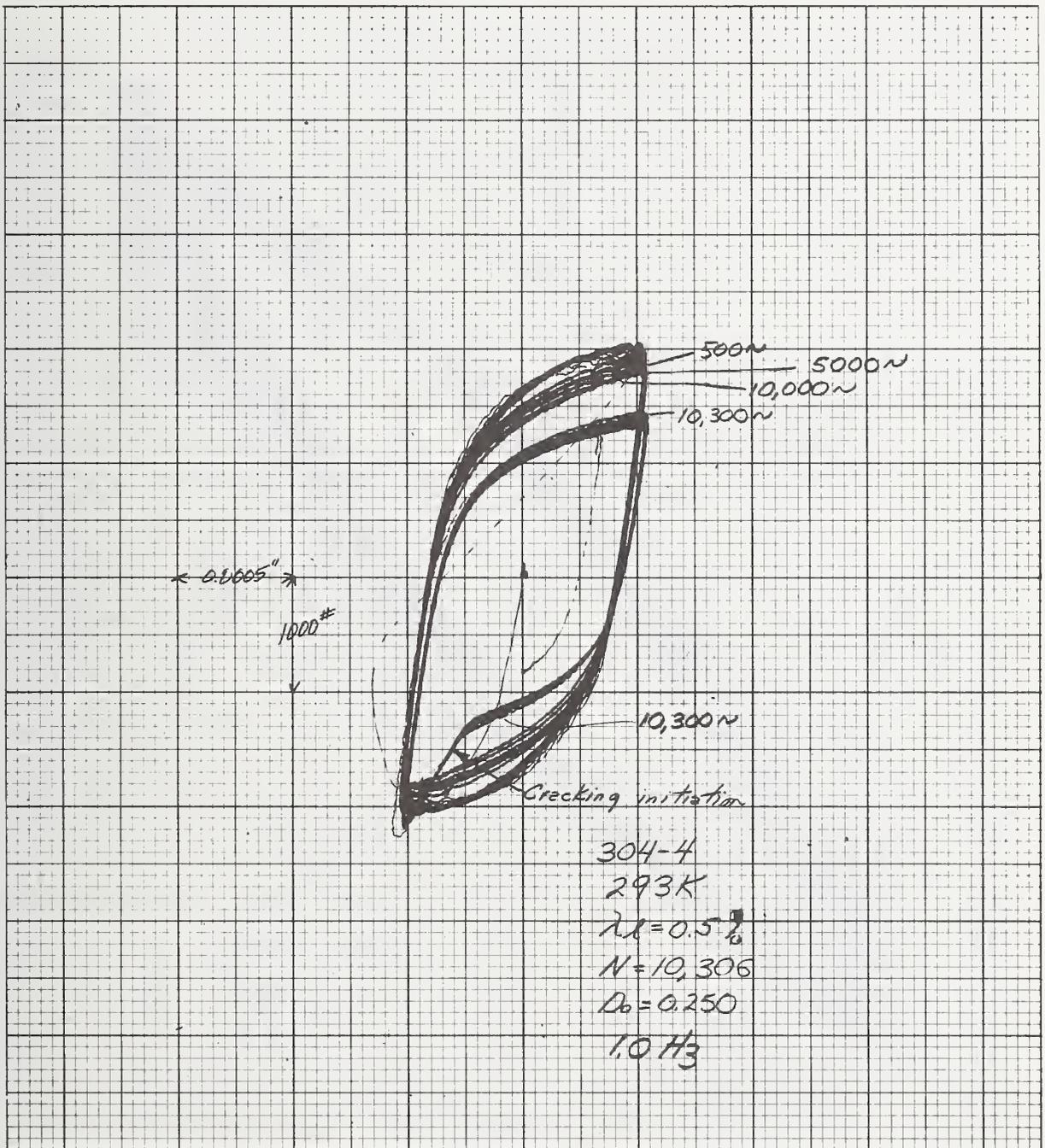
Figure 10 Load-Deflection Curve for Specimen 304-4
