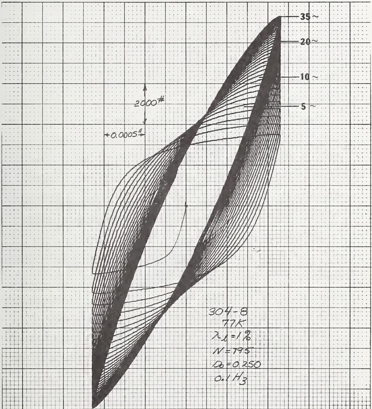
Figure 9 Load-Deflection Curve for Specimen 304-8
