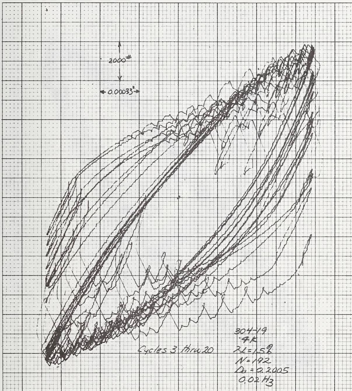
Figure 13 Load-Deflection Curve for Specimen 304-19 (Cycles 3 through 20)
