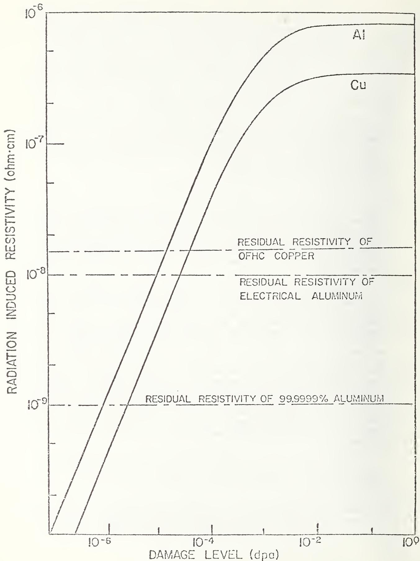
Figure III.D.1. Radiation induced resistivity of copper and aluminum. From UWMK III.
