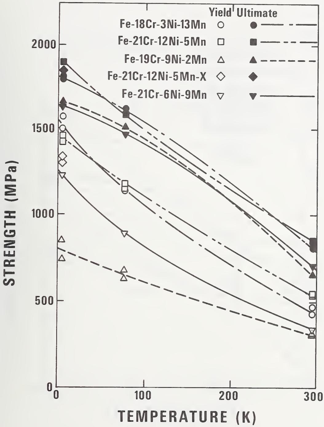
Figure 11. Yield and ultimate strengths of materials used in the present study.
