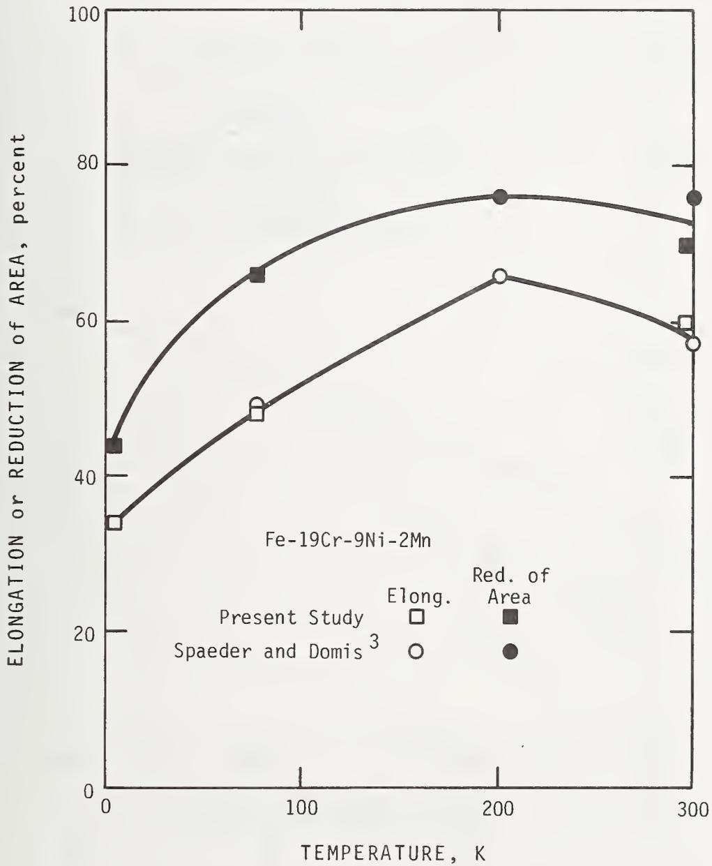
Figure 17. Elongation and reduction of area data for  ${}^3\text{Fe-19Cr-9Ni-2Mn}$  from the present study and from Spaeder and Domis.<sup>3</sup>
