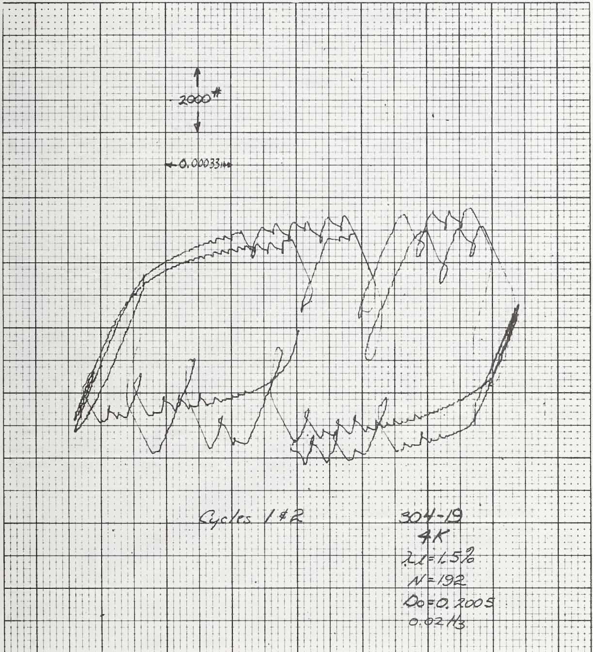
Figure 12 Load-Deflection Curve for Specimen 304-19 (Cycles 1 and 2)
