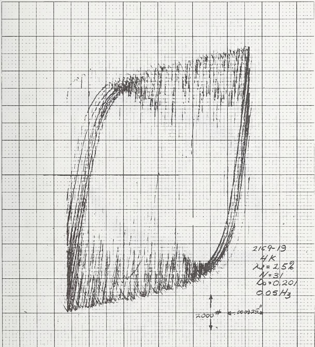
Figure 19 Load-Deflection Curve for Specimen 2169-19
