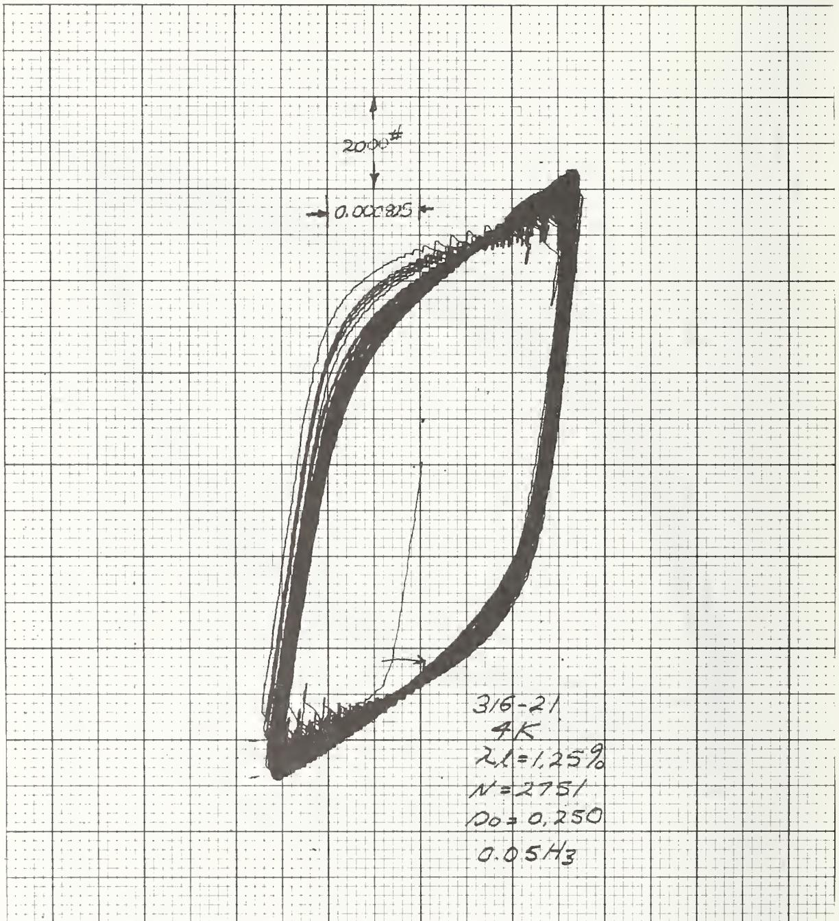
Figure 23 Load-Deflection Curves for Specimen 316-21
