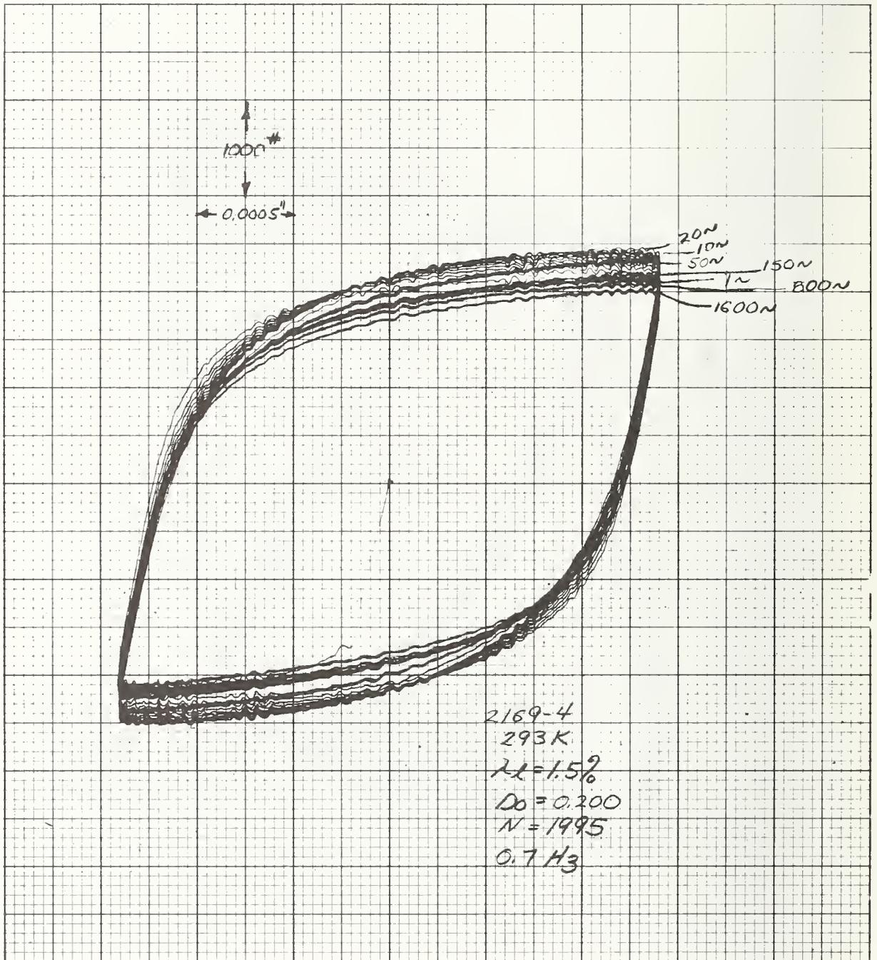
Figure 20 Load-Deflection Curve for Specimen 2169-4
