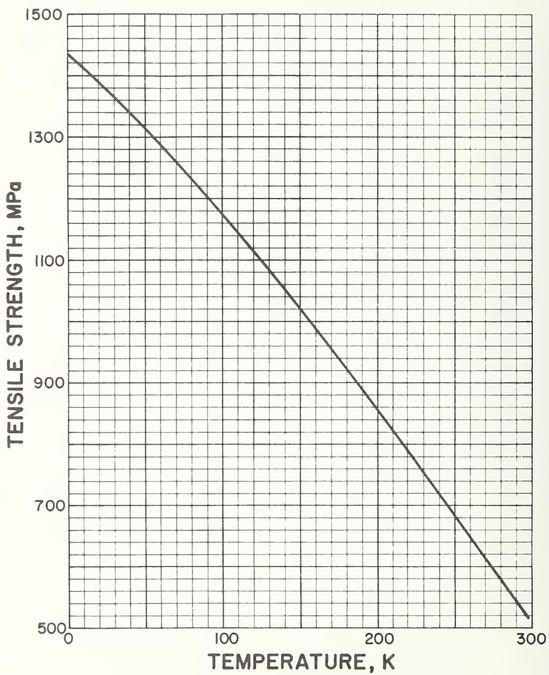
Figure 1. Tensile strength of AISI 316 stainless steel.
