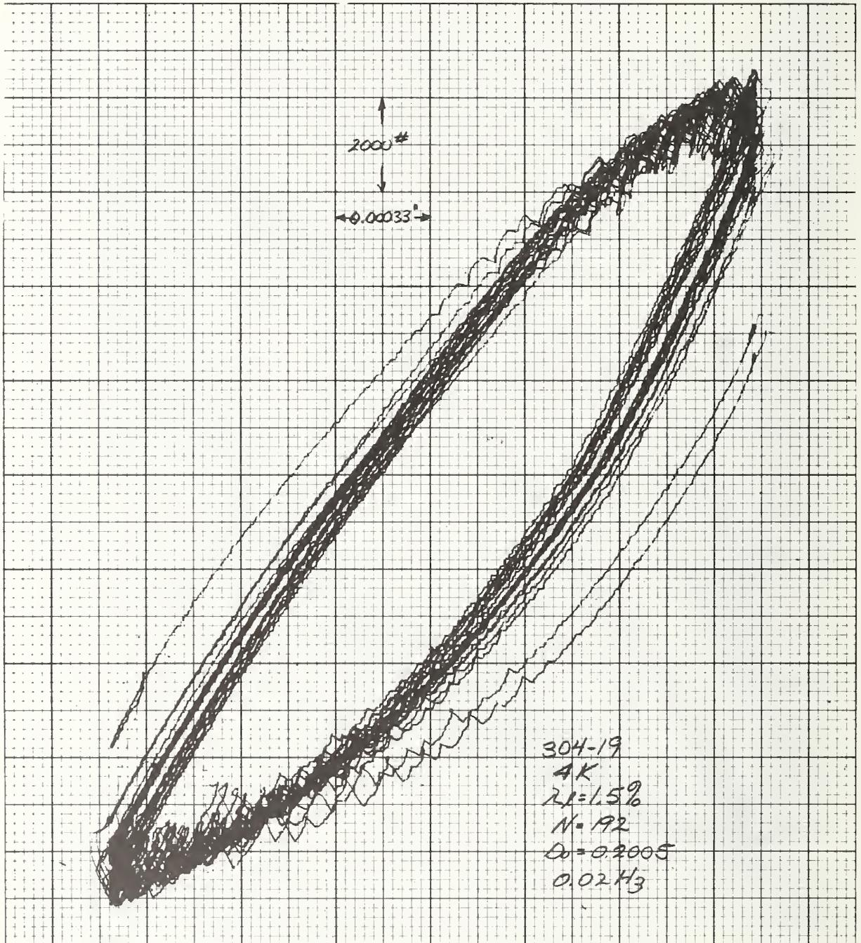
Figure 14 Load-Deflection Curve for Specimen 304-19 (Cycles 21 through 40)
