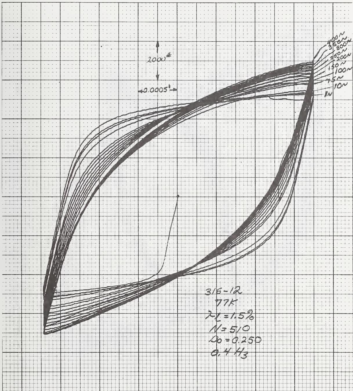
Figure 22 Load-Deflection Curves for Specimen 316-12
