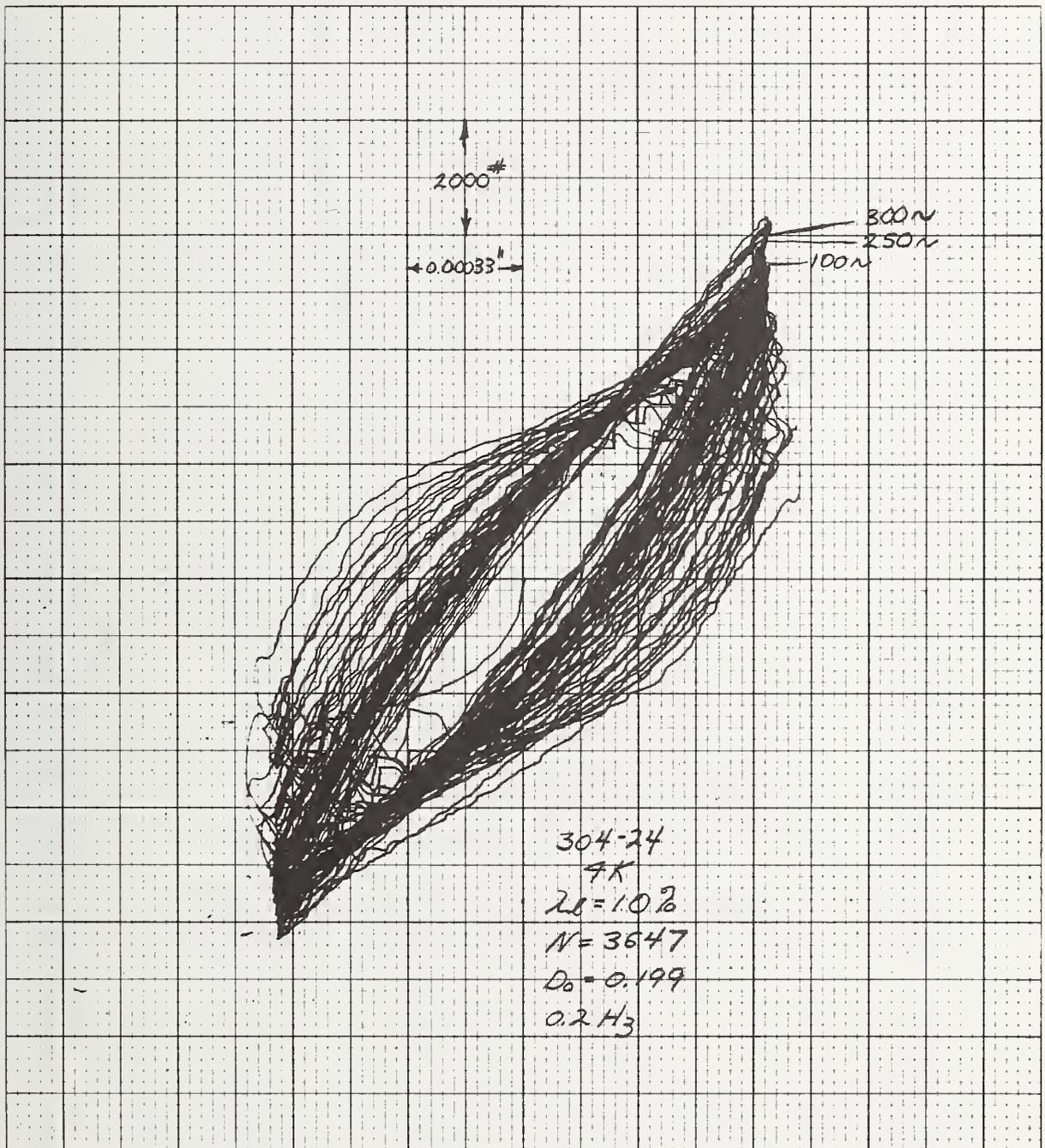
Figure 15 Load-Deflection Curve for Specimen 304-24
