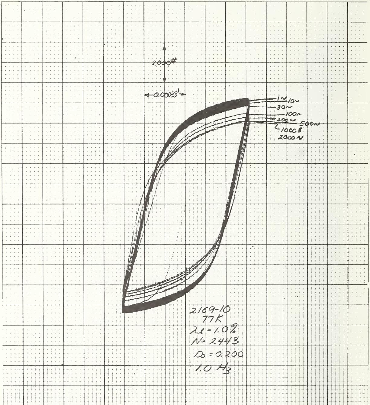
Figure 17 Load-Deflection Curve for Specimen 2169-10
