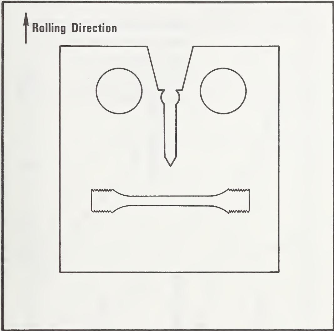
Figure 5. c. Relative orientation of fracture toughness and tensile specimens and plate stock.
