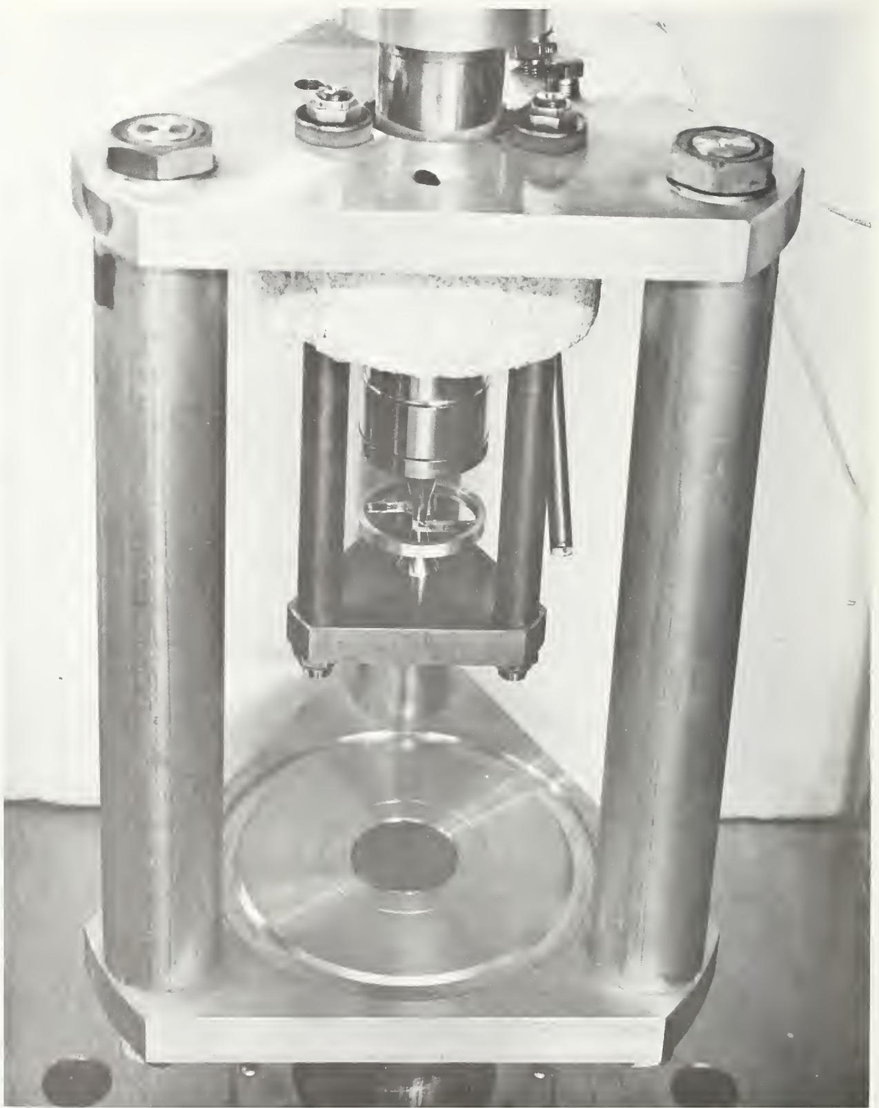
*Figure 5 Load Train for 4 K Testing*
