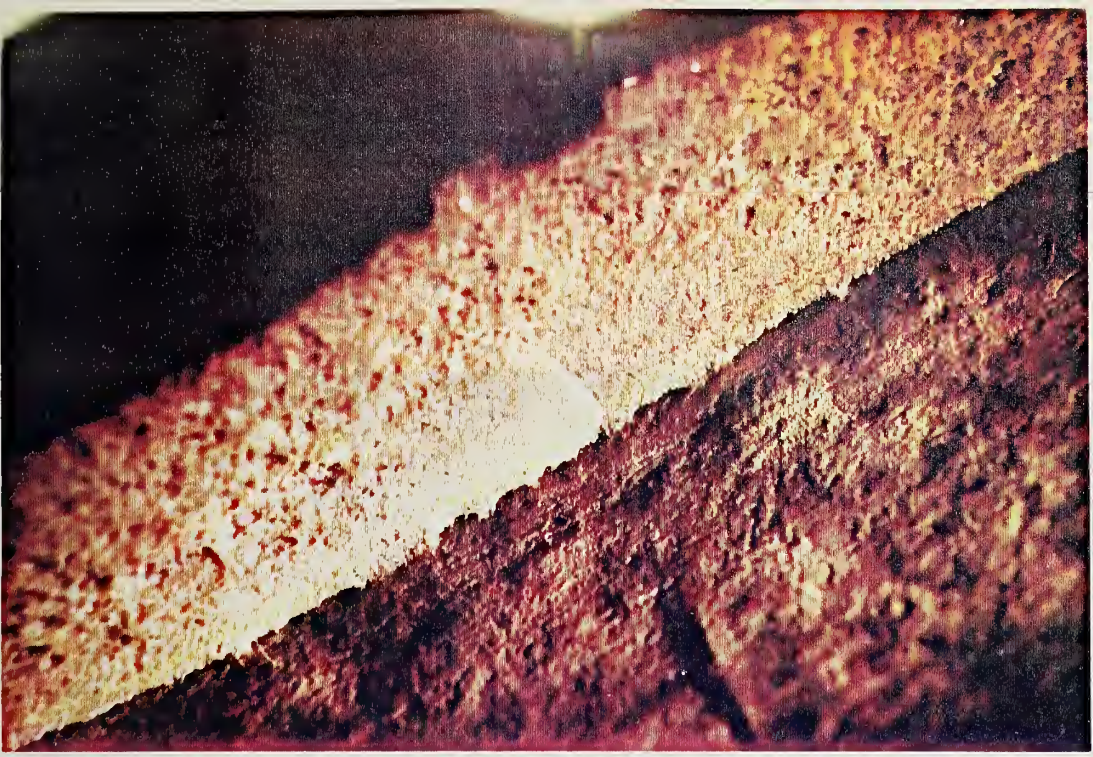
Figure 8a. Fracture origin on piece RR-12 before cleaning, viewed toward inside wall.
