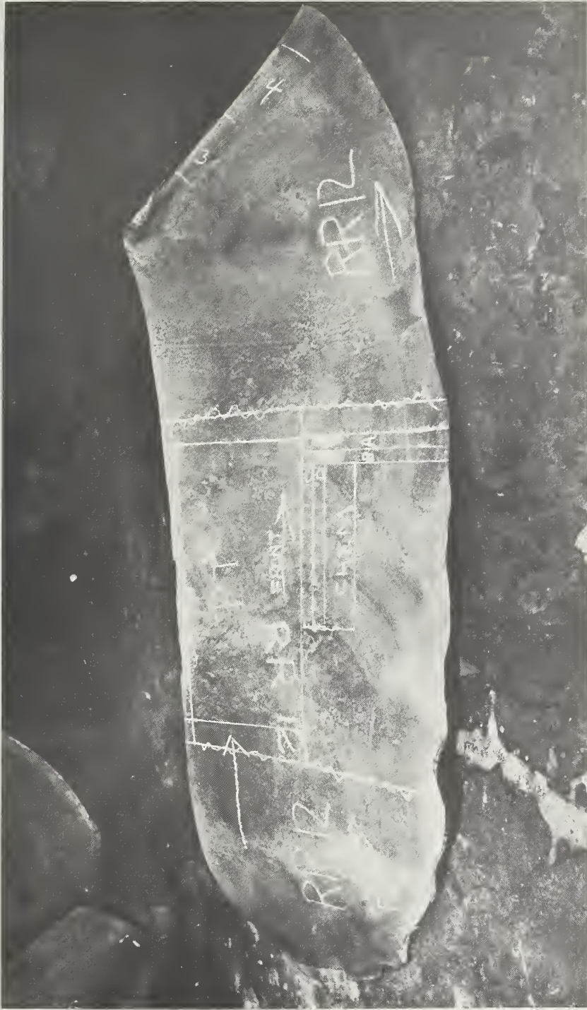
Figure 5. Inside wall of piece RR-12 showing location of specimen taken for chemical analysis. The arrows point in the longitudinal direction. This piece is about 30-inches wide by about 50-inches long. (Photo courtesy of M. Bolinger, Jr., Gladstone Laboratories, Inc., Cincinnati, Ohio.)
