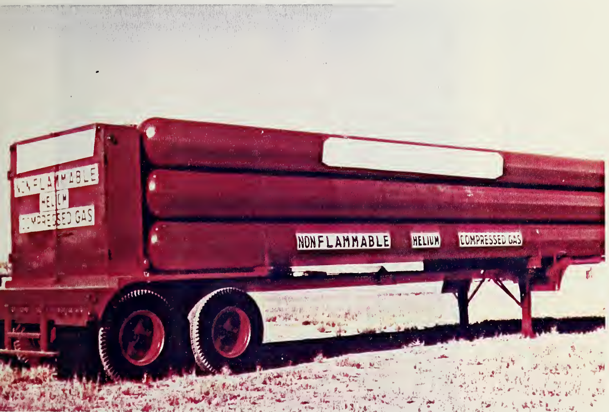
Figure 4. Intact tube trailer composed of specification DOT 3T cylinders. The array of cylinders on the trailer is 3-high by 4-wide. (Photo courtesy of Mr. W. Piehl, Western Sales and Testing, Inc., Amarillo, Texas.)
