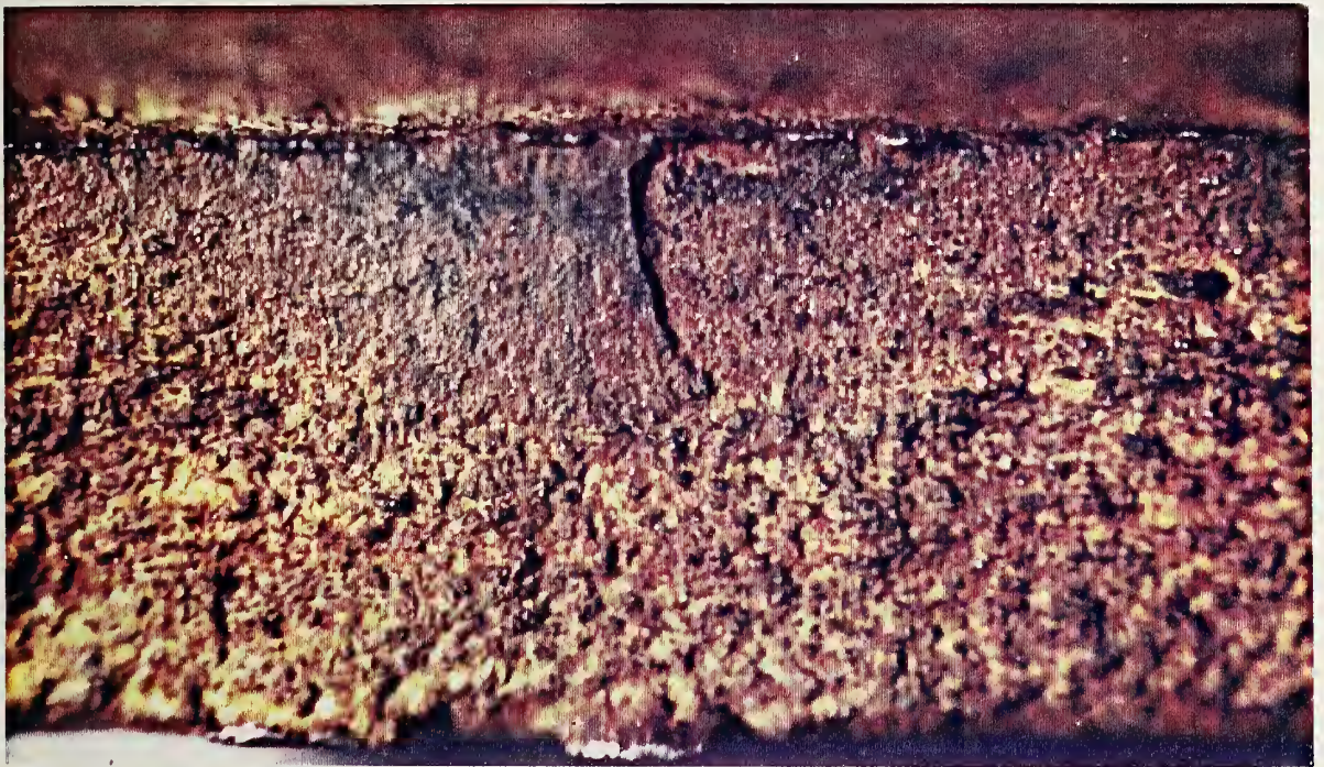
Figure 21. Close-up view of the fracture origin after stripping three cellulose acetate replicas. The black product on the fracture surface became evident as the orange-brown product was stripped away. This view is towards the inside wall.
