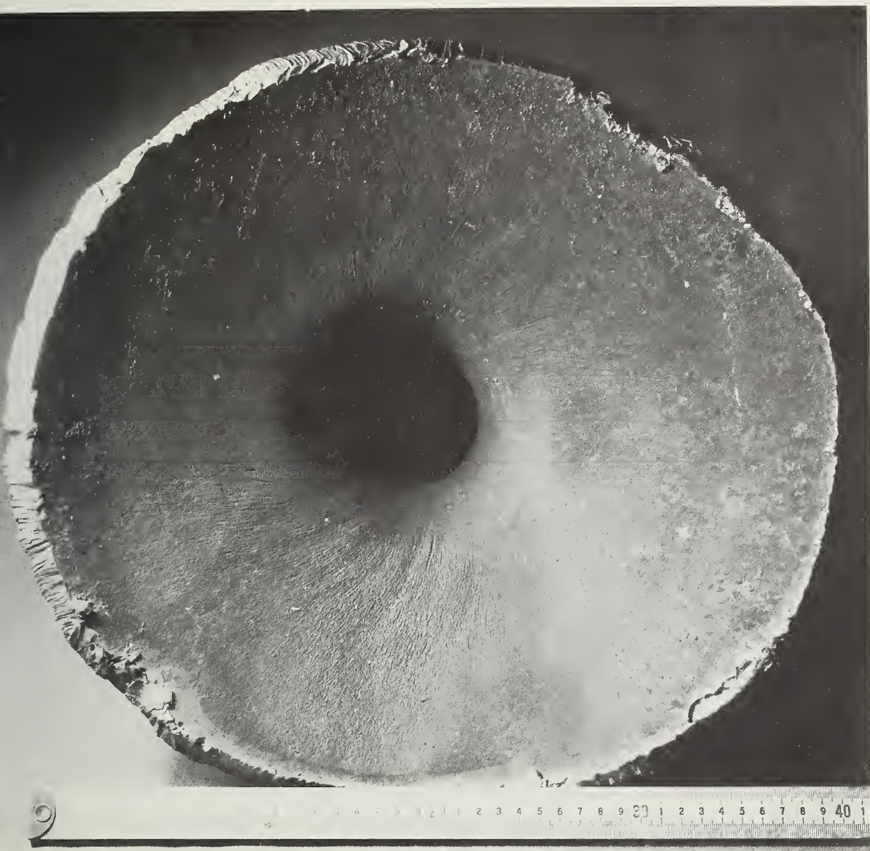
Figure 9a. Forging seams evident on inside wall at front head of cylinder 10041. The scale is in centimeters.
