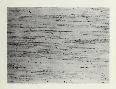
Figure 2. Microstructure of 7049-T73510 aluminum extrusion (long transverse direction). Etched, Keller's etch, X 50.
