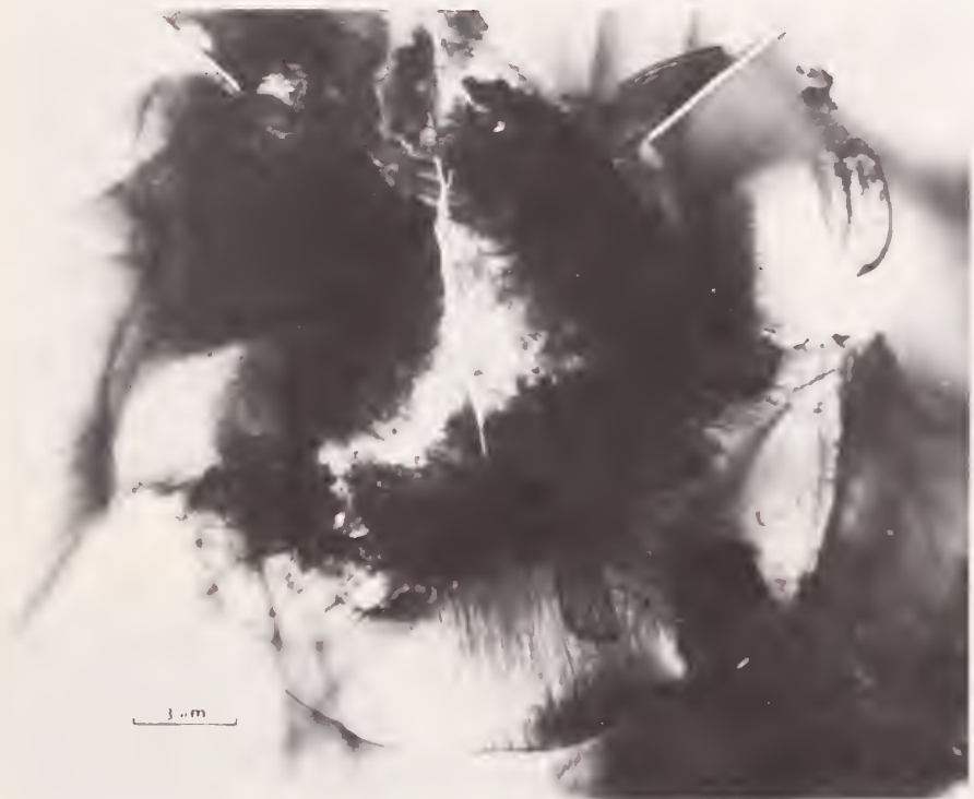
Fig. 13. Impact site in SiC produced by 150 \mu\text{m} SiC particles at a velocity of 94 m/s and a 90° impact angle. (Courtesy of Hockey).
