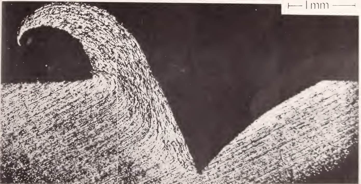
Fig. 7. (a) Impact geometry and crater produced in steel. Velocity and rake angle are shown.
