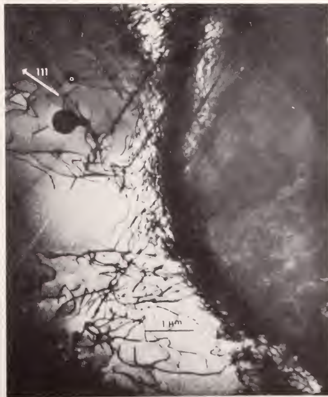
Fig. 5. (a) Impact crater in 310 stainless steel produced by 50 \mu m glass sphere at 20° attack angle at 59 m/s.
