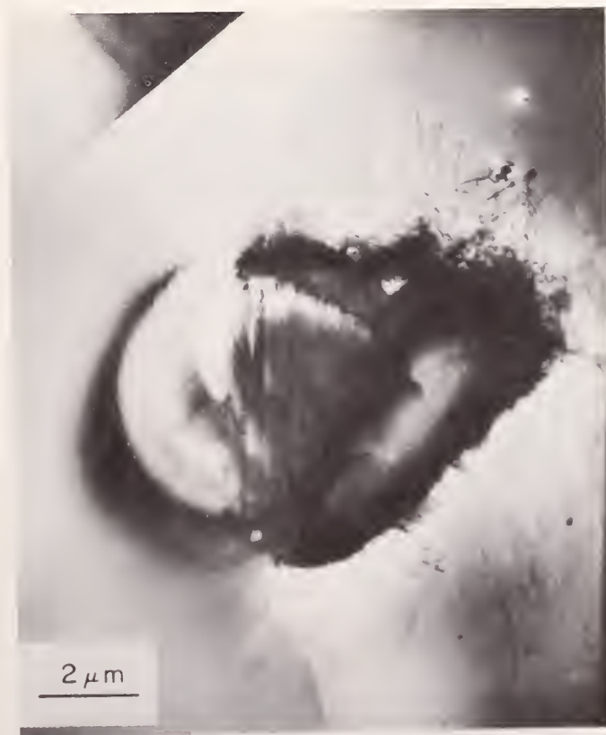
Fig. 4. Impact craters in 310 stainless steel produced by 50 \mu\text{m} \text{Al}_2\text{O}_3 particles at 59 m/s. (a) SEM and (b) TEM micrographs of crater produced at 90° attack angle. (Ives and Ruff, 1978a).
