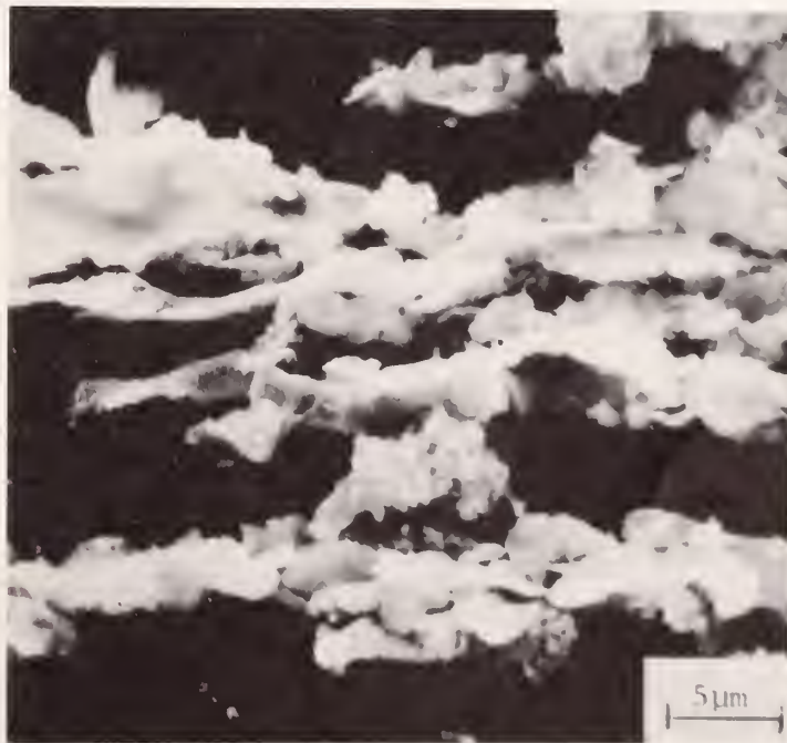
Fig. 34. Scanning electron micrographs of (a) the surface of abraded 1015 steel and (b) steel debris particles recovered after wear under dry conditions at 2.2 N load. (Ruff, 1978).
