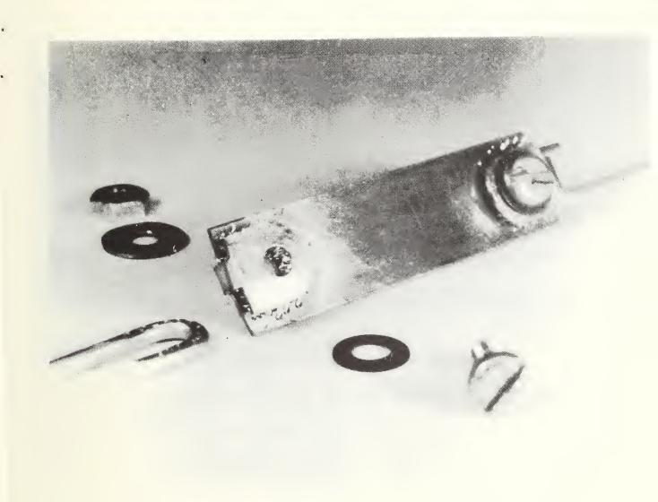
Figure 2 - Experimental connector for aluminum or copper wire designed to be used with Belleville washers so as to compensate for the creep of the wire. The screw does not carry current.
