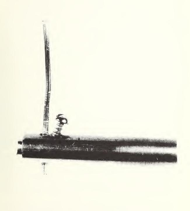
Figure 4 - Experimental connector for wire using a screw wedge.
