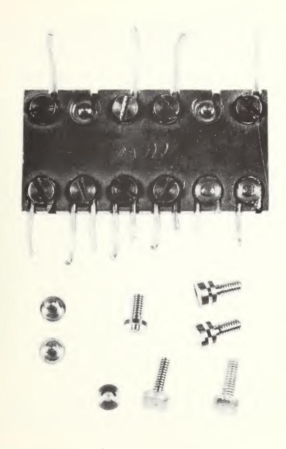
Figure 1 - Experimental connector designed for a particular size of aluminum wire. Also shown are special screws, the heads of which are sheared off when the proper tightening torque is reached.
