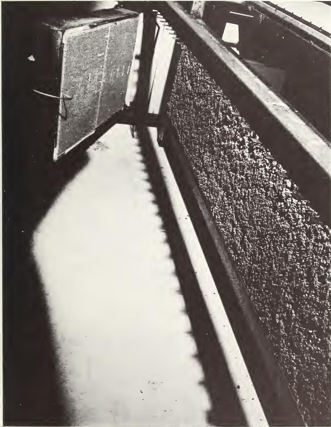
Figure B2. Horizontally-mounted attic floor insulation specimen
