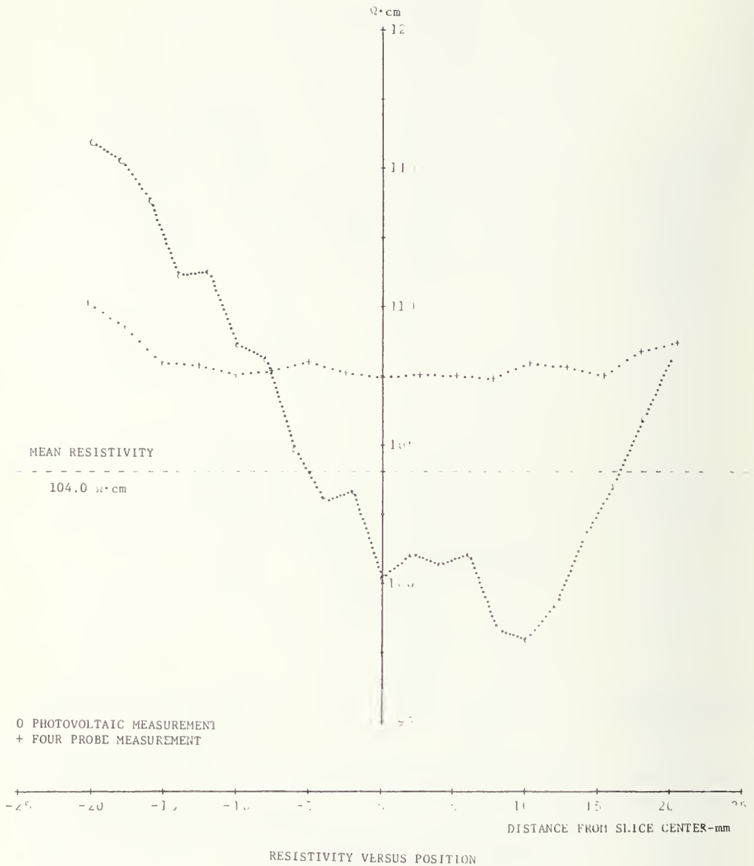
Figure 2-10. Comparison of four-probe and photovoltaic resistivity profiles for an NTD specimen with normal resistivity gradient.
