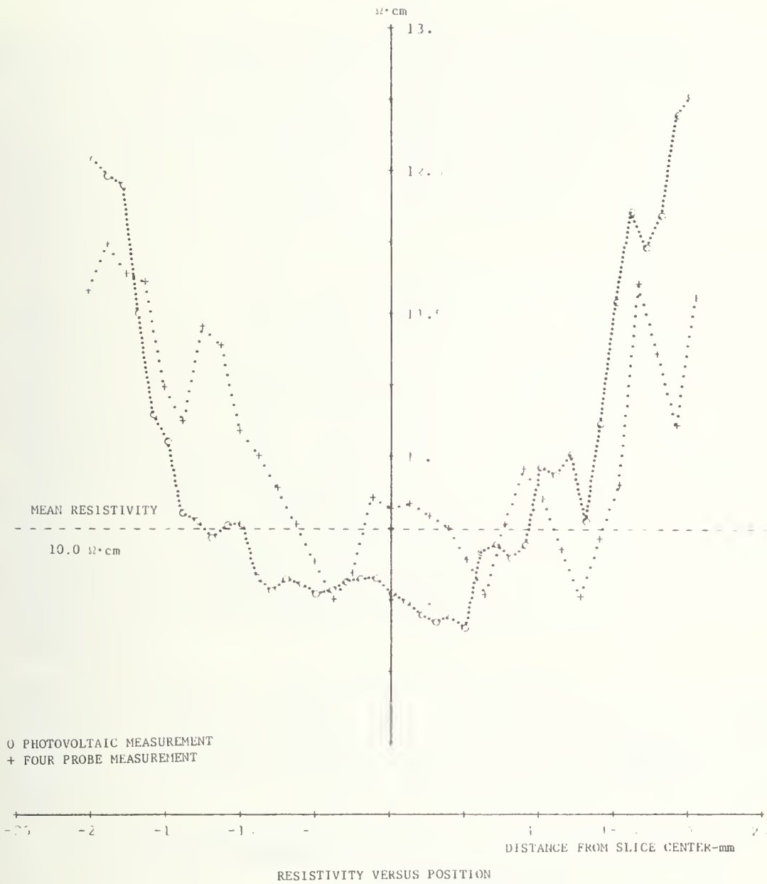
Figure 2-9. Comparison of four-probe and photovoltaic resistivity profiles for an n -type silicon slice of nominal resistivity of 10 \Omega \cdot \text{cm} .
