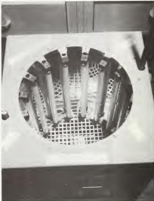
Fig. 3. Interior view of the photochemical reactor.
