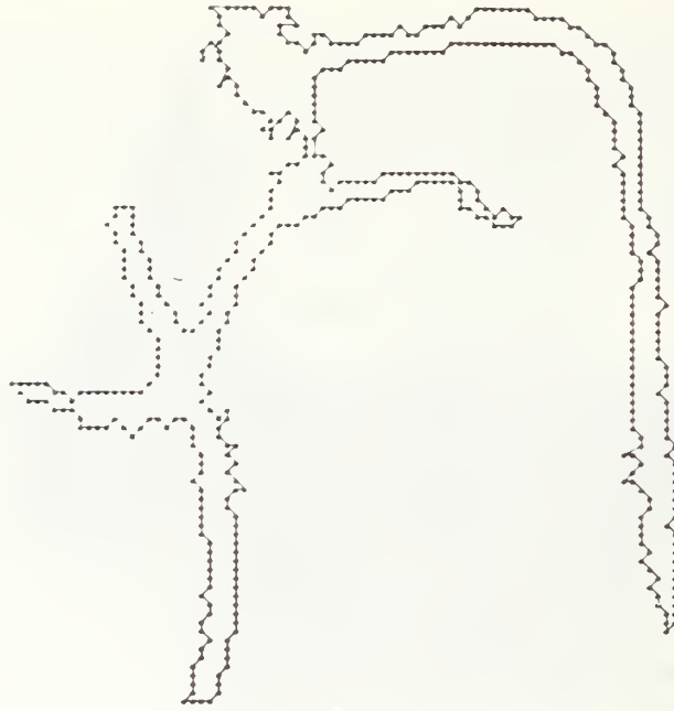
Figure 17: Boundary points of single connected blob extracted from Figure 4 by thresholding at mean density, 157
