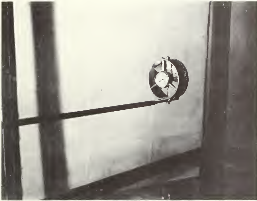
FIGURE 1. THE ANEMOMETER MOUNTED IN THE TUNNEL.
