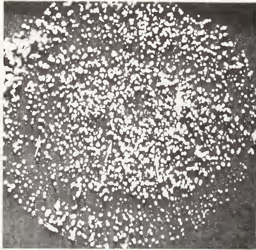
Fig. 7. A neon field ion micrograph obtained from a 304 stainless steel specimen, 30K, 12,500 volts. Arrows indicate crystal net plane rings.
