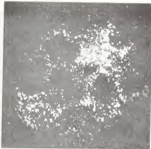
Fig. 10. A field ion micrograph obtained from the same specimen as imaged in Fig. 8, imaged in a neon and hydrogen gas mixture, 30K, 15,000 volts.
