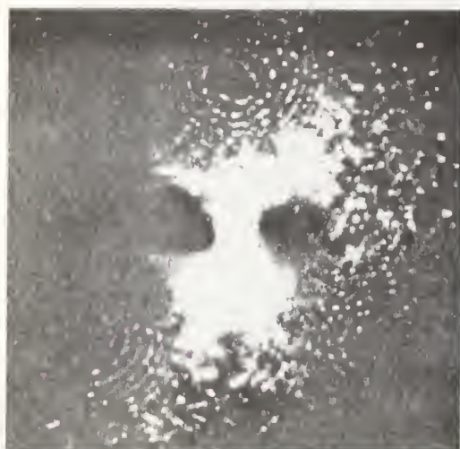
Fig. 12. A hydrogen field ion micrograph obtained from the same iron specimen as used in Fig. 11, 30K, 6600 volts.
