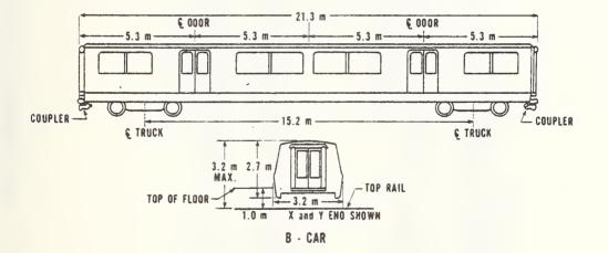
Figure 1. Exterior views of A-car and B-car configurations
