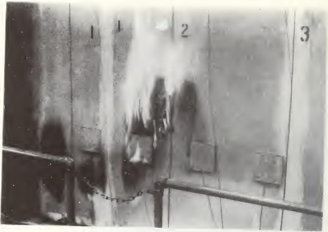
Figure 45. Test FE 2 - Burn-through at end of test
