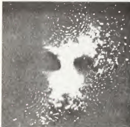
Fig. 12. A hydrogen field ion micrograph obtained from the same iron specimen as used in Fig. 11, 30K, 6600 volts.
