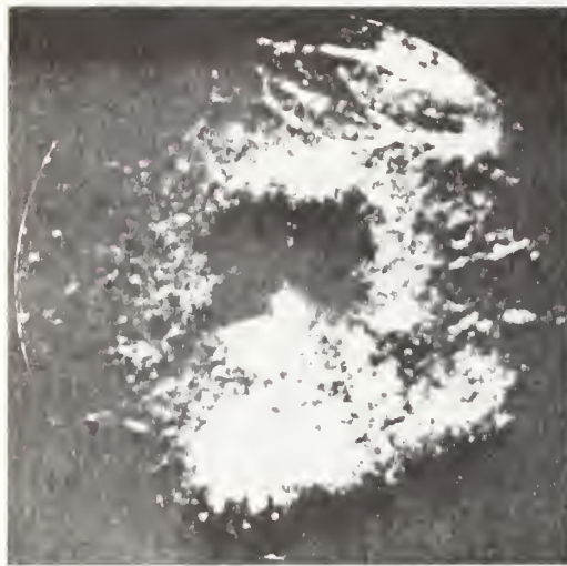
Fig. 4. A hydrogen field ion micrograph obtained from a 1080 steel specimen at room temperature, 8800 volts. See text for additional details.
