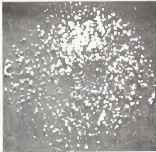
Fig. 2. A hydrogen field ion micrograph obtained from the same 1080 steel specimen as imaged in Fig. 1, 25K, 2600 volts. Note the appearance of two dark areas near the center of the micrograph. Both are artifacts that appear in most of the following micrographs.
