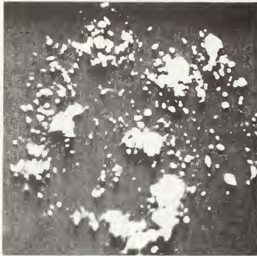
Fig. 3. A field ion micrograph obtained from the same 1080 steel specimen as imaged in Fig. 1, following its exposure to the hydrogen imaging conditions described in Fig. 2, and imaged in a 55% helium and 45% neon gas mixture, 25K, 5000 volts.
