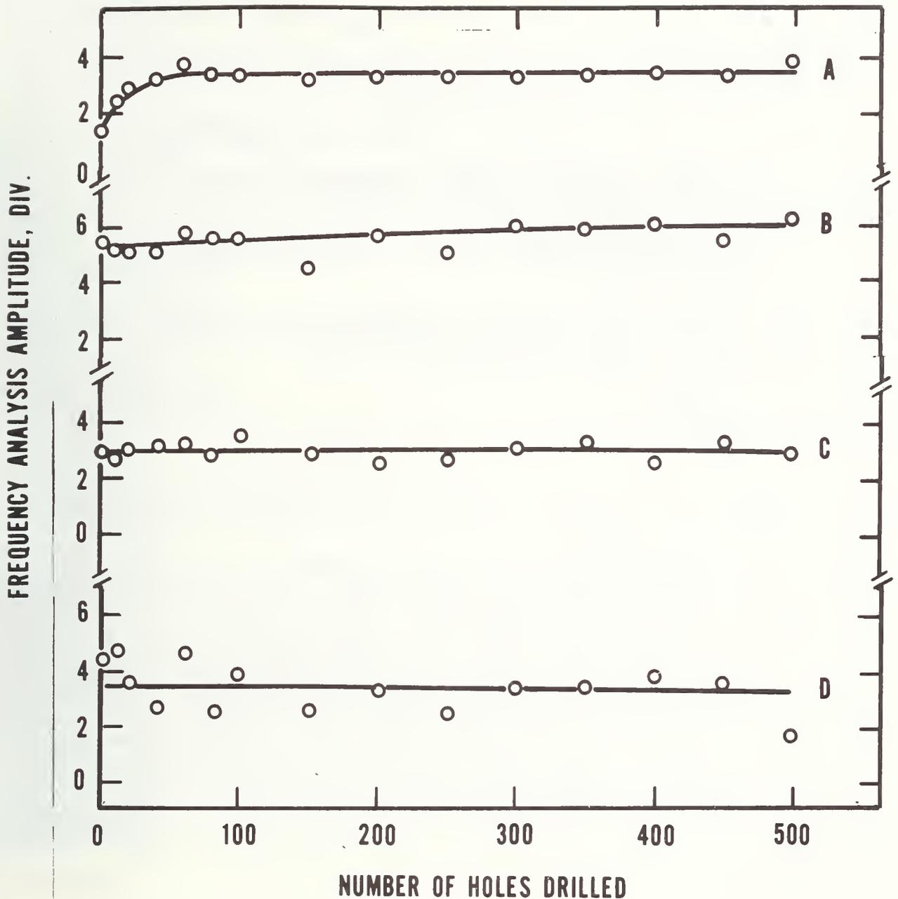
Figure 11: Plots of spectral amplitude at selected frequencies as a function of number of holes drilled. Data for both force and torque are shown. The amplitude data are scaled from the four frequency-analysis oscilloscope photographs taken for each set of holes drilled in steel. (Typical oscilloscope photographs are shown in figures 9 and 10.)
