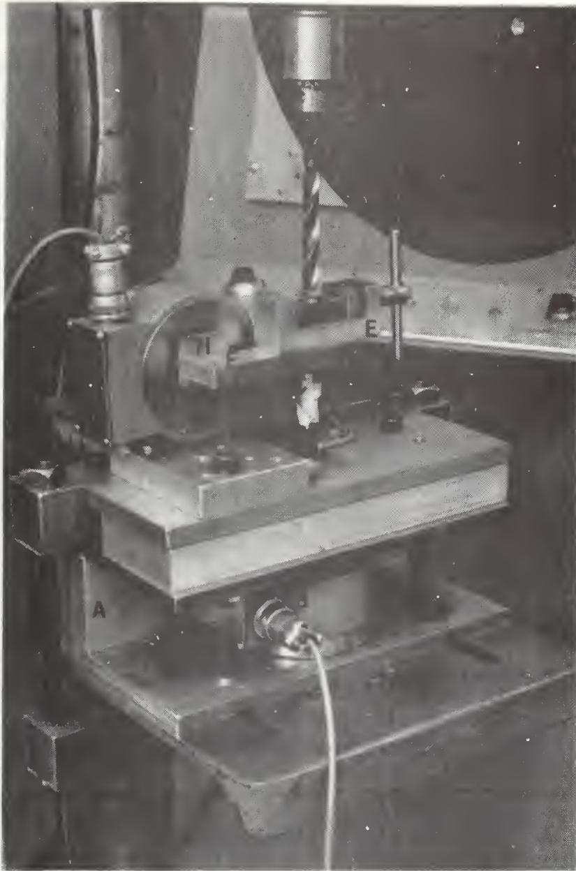
Figure 5: Force-and-torque measuring fixture - second model. Identified are the length of U-channel (A) into which the load cell (B) measuring downward force is mounted: the brass rod (C) instrumented with strain gage (D) and supporting vise (E) with arm (F). Also shown are the load cell (G) measuring torque and shims (H) for adjusting torque preload. The workpiece is in the vise at (I).
