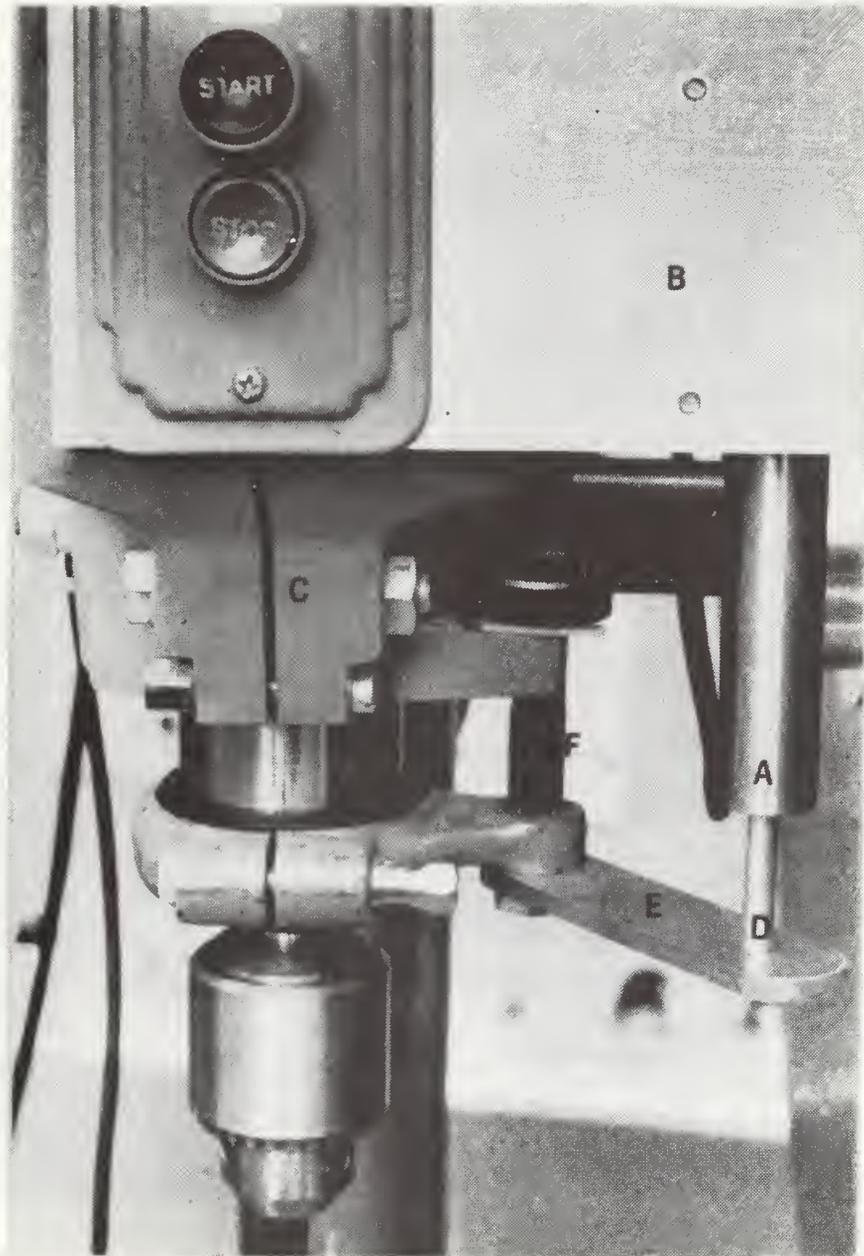
Figure 3: Displacement-measuring instrumentation. Identified are the LVDT transducer sensing coil (A) mounted by means of bracket (B) to the head casting (C). The transducer armature (D) is mounted by a bracket (E) attached to the vertical stop screw (F).
