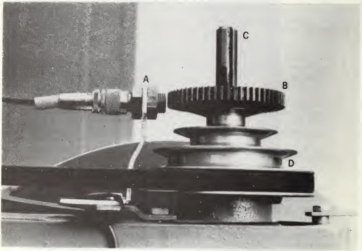
Figure 2: Drill spindle-speed instrumentation. Identified are the magnetic sensing coil (A) and the 60-tooth steel gear (B) mounted on the spindle shaft (C). One of the two stepped pulleys of the belt drive is shown at (D).
