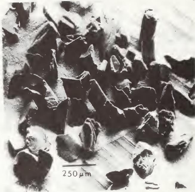
Figure 1. Scanning electron micrograph illustrating angular morphology of silicon carbide particles used in impact damage and erosive wear studies.
