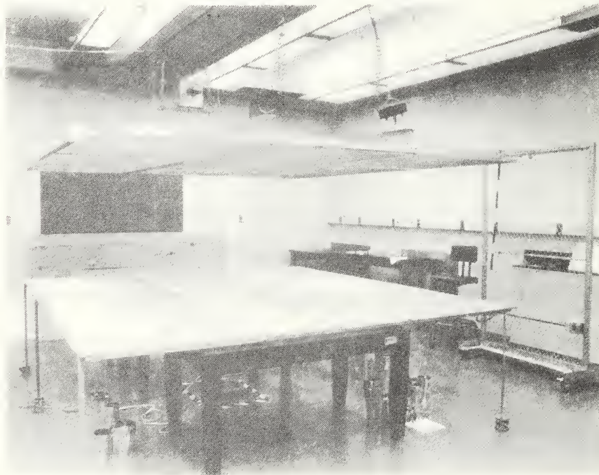
Figure 10. Large parallel plates with 1 m separation. Each plate consists of nine 1 m x 1 m tightly stretched aluminum window screens mounted on an aluminum frame.
