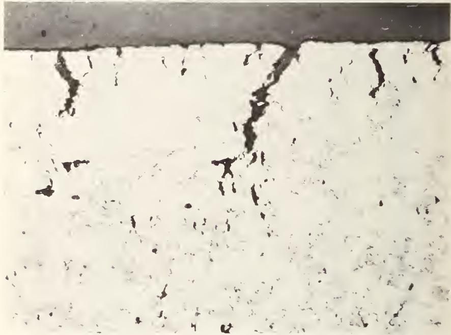
Figure 9. Photomicrograph of the etched cross-section of the Inconel 671 specimen in Figure 7. 500X.
