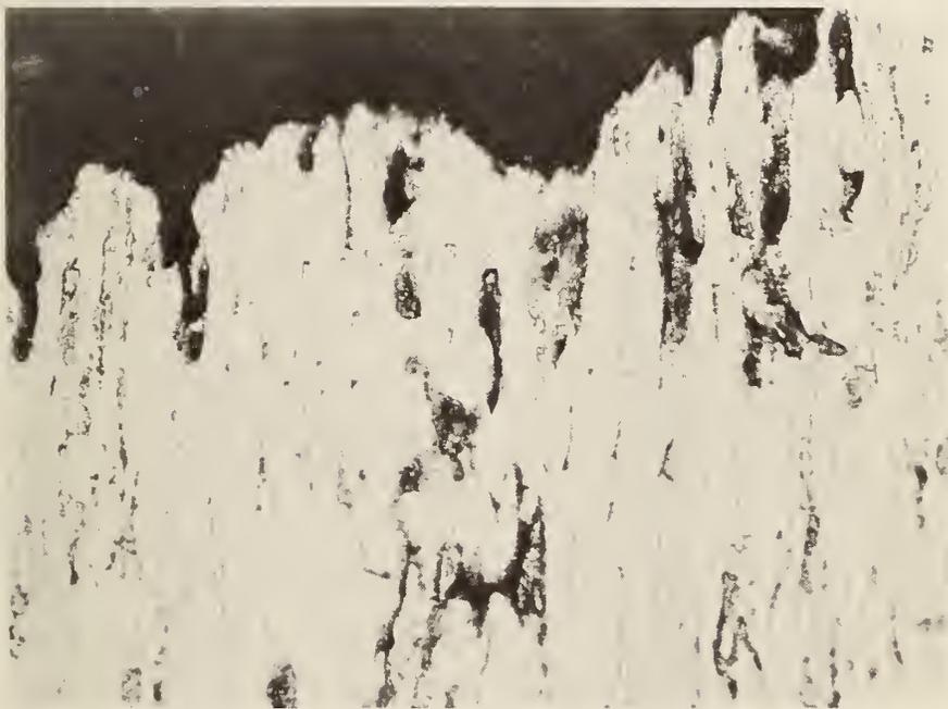
Figure 6. Photomicrograph of the etched cross-section near the fracture of the 446 stainless steel specimen in Figure 2. 500X.
