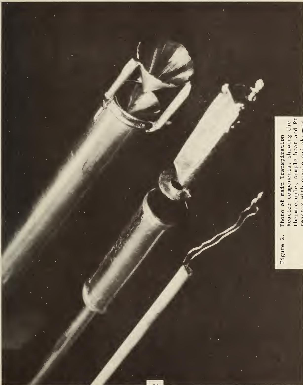
Figure 2. Photo of main Transpiration Reactor components, showing the thermocouple, sample boat and Pt reactor with nozzle and skimmer attached.
