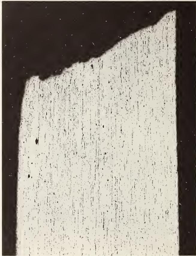
Figure 11. Photomicrograph of the etched cross-section near the fracture of an Inconel 671 specimen tested at 450°C (840°F) at  $1 \times 10^{-6} \text{s}^{-1}$  in ultra-pure helium. 25X.
