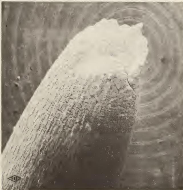
Figure 2. Scanning electron micrograph of a 446 stainless steel specimen tested at 600°C (1100°F) at a strain rate of  $1 \times 10^{-6} \text{s}^{-1}$  in ultra-pure helium. 20X.
