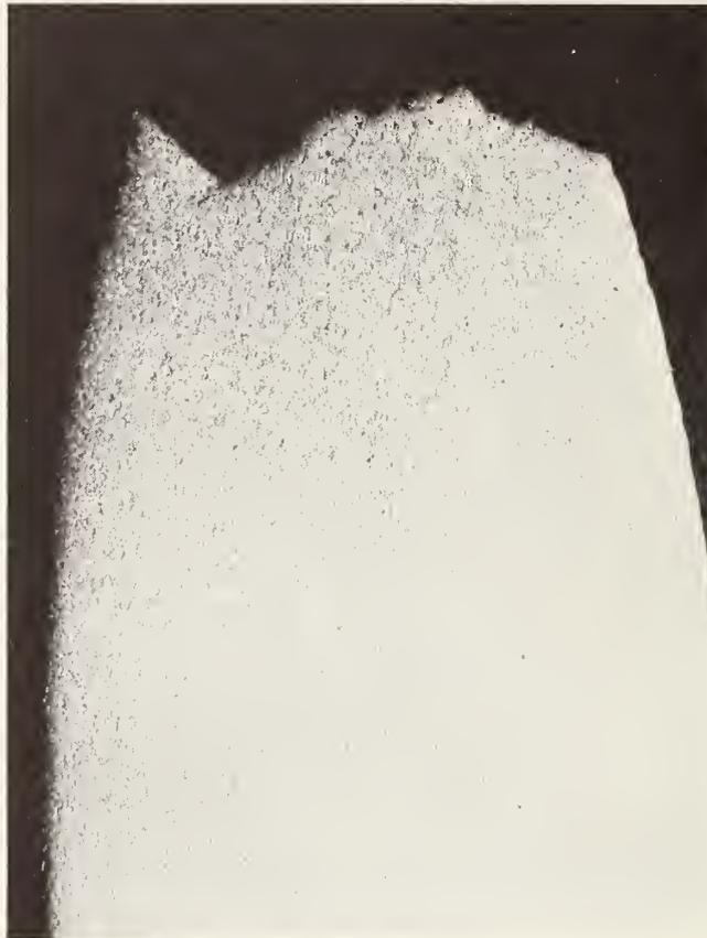
Figure 3. Photomicrograph of the etched cross-section of the 446 stainless steel specimen in Figure 1. 25X.
