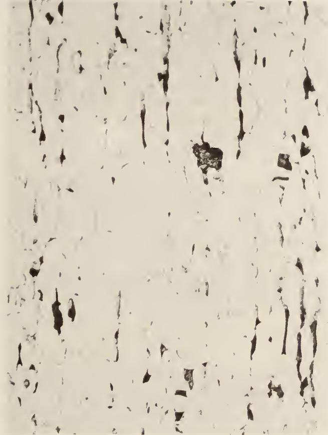
Figure 12. Photomicrograph of the etched cross-section of the Inconel 671 specimen in Figure 11. 500X.
