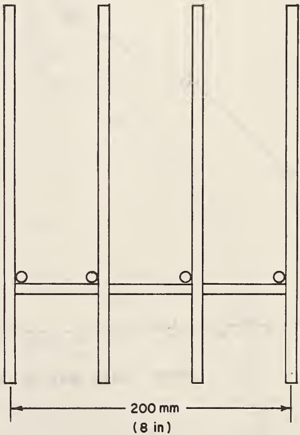
Figure 7. Mattress Sample Holder for Small Scale Compartment
