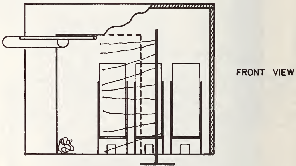
Figure 4. Front and Plan Views of Small Scale Compartment Showing Location of Samples, Alcohol Troughs and Instrumentation
