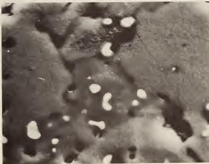
Fig. 7. Polished surface of spinel near lead-out, G.E. anode (5000X).
