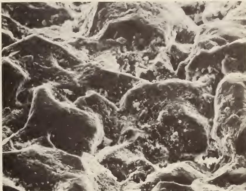
Fig. 6. Secondary electron image of insulator surface, G.E. cathode assembly (800X), Plasma flow was from top to bottom.
