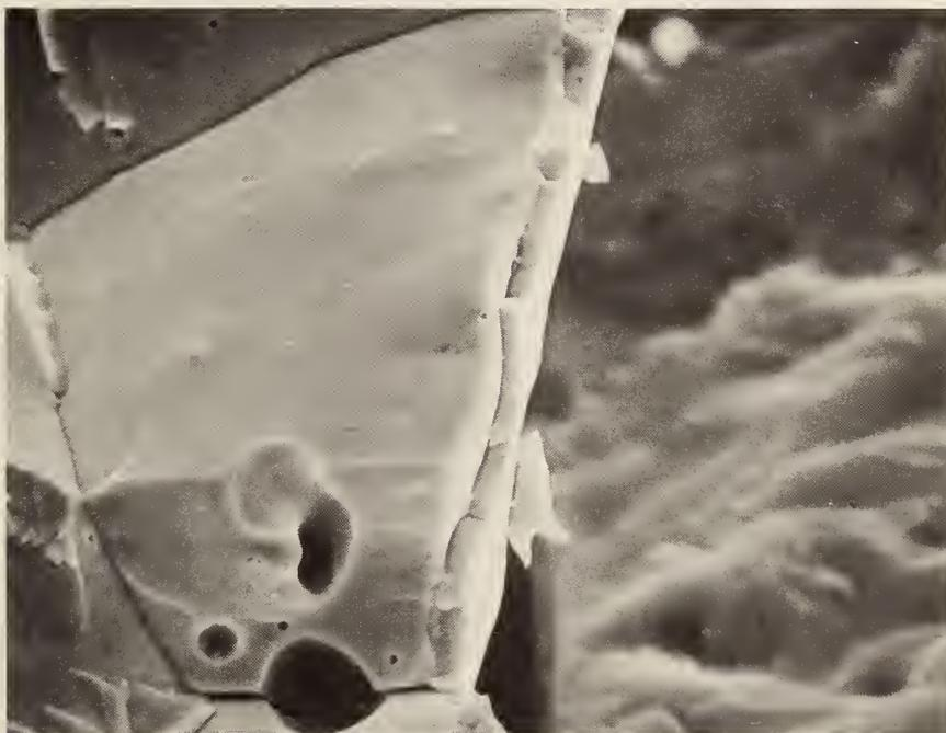
Fig. 2 c. Thin skin adhering to Mo wall (left) at interface with melt (right) 7000X).
