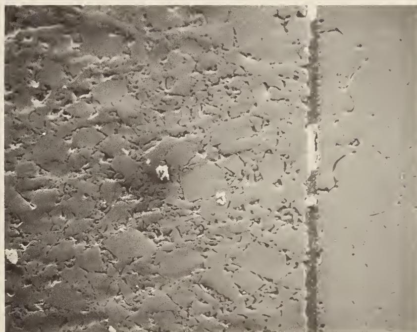
Fig. 19 . 100 SEM micrograph showing separation of MgO (coarse-ground material) and MAFF-31.
