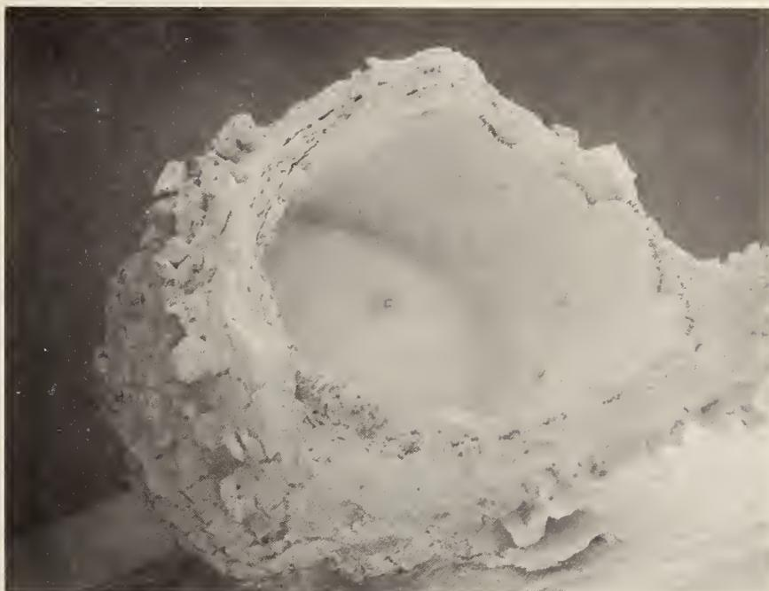
Fig. 1. Fractured surface of Ta capsule with  $(KAlO_2)_{70}(SiO_2)_{30}$  sealed inside, run at  $\sim 2200$  °C in forming gas. Remainder of melt is visible in bottom (40X).
