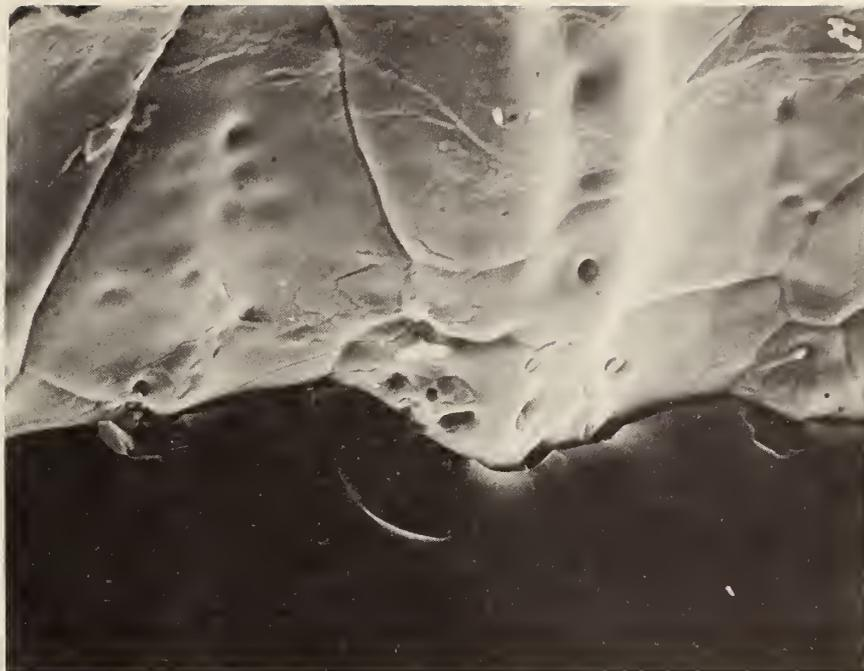
Fig. 2 b. Contact between melt and Mo (1400X).
