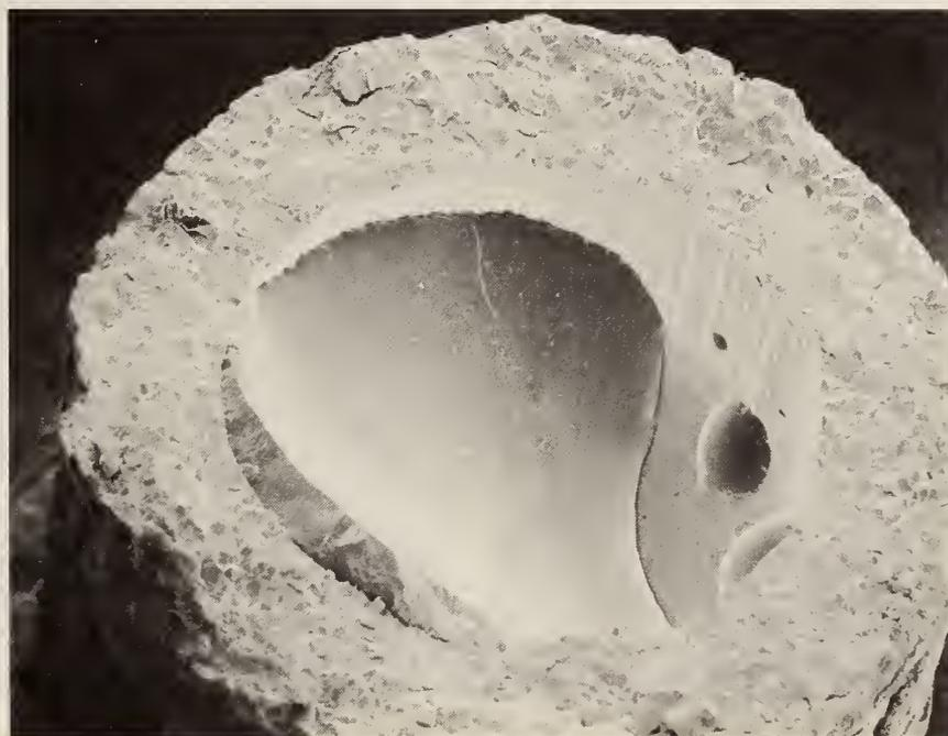
Fig. 2 a. Mo capsule, experiment identical to Fig. 1. Melt in bottom of capsule (35X).
