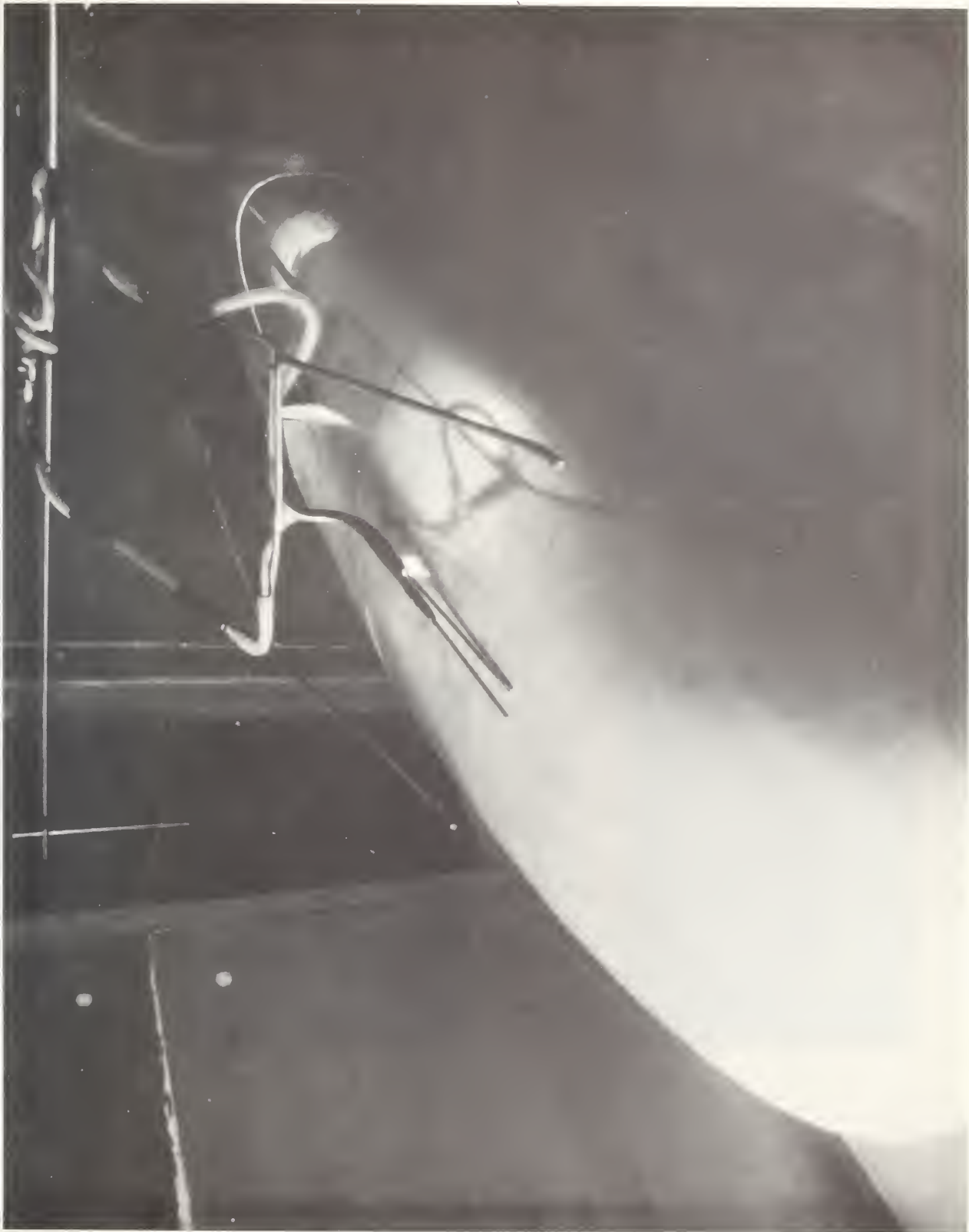
FIGURE 9. SURFACE-TUBE ARRANGEMENT FOR DETECTING TRANSITION
