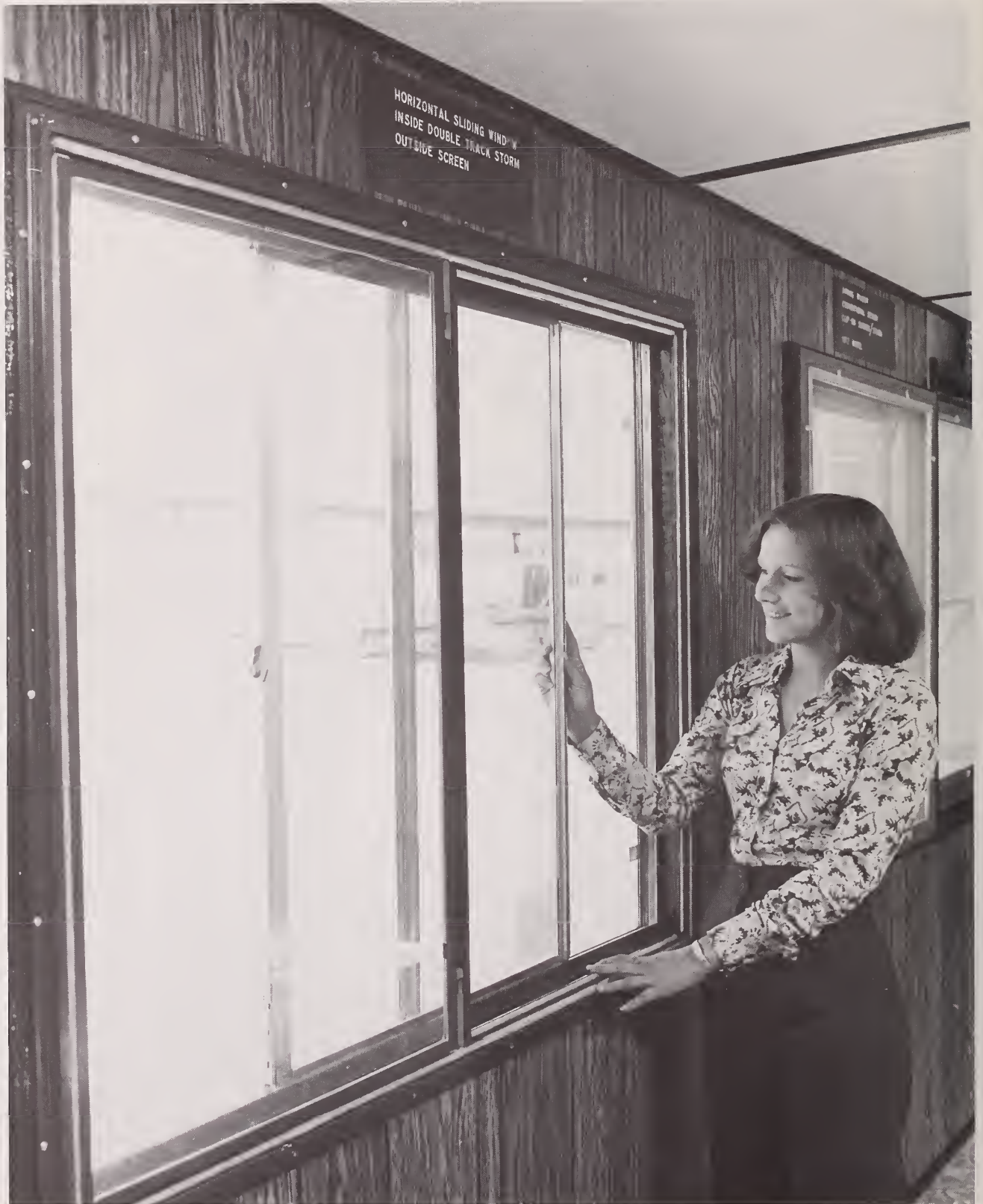
Figure 23. Egress Test. Specimen 5. Opening prime window
