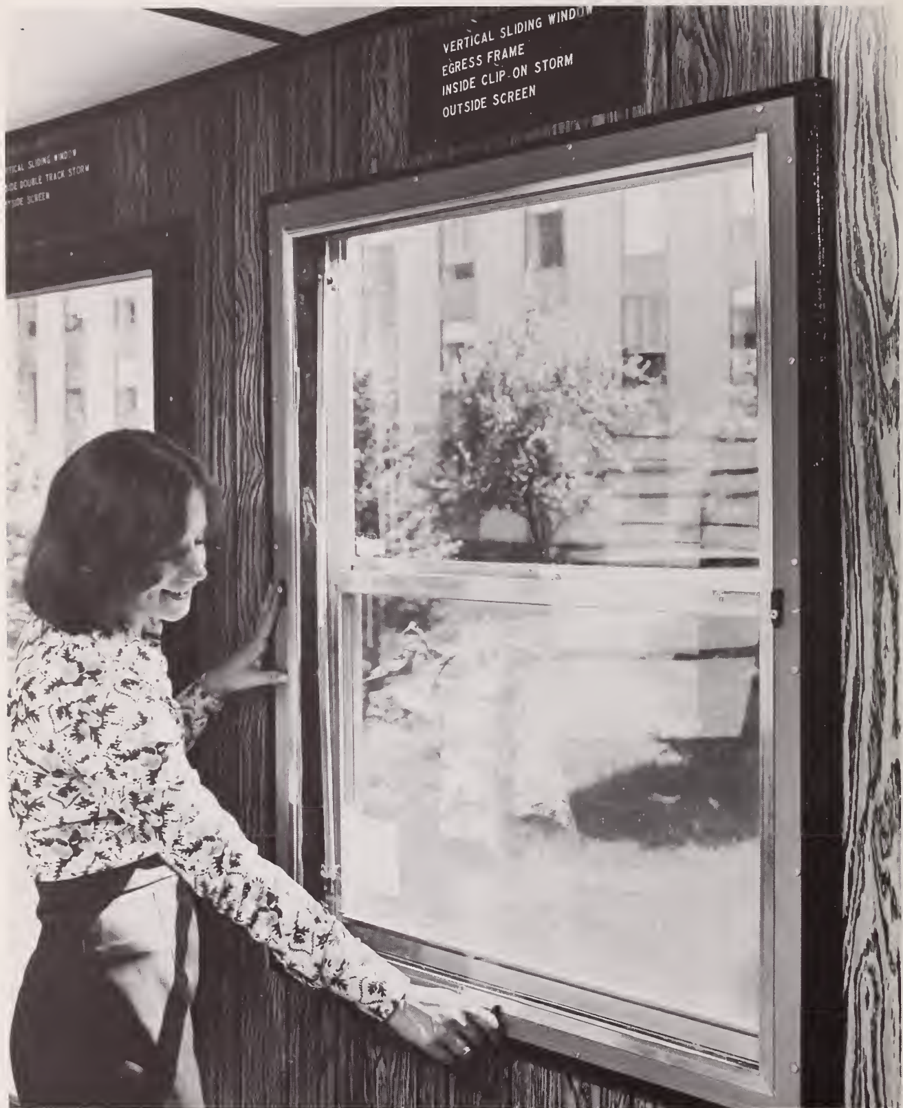
Figure 17. Egress Test. Specimen 3. Releasing storm window retaining clip Releasing one of three clips which retain inside clip-on storm window. The same storm window frame is used on specimen 4.
