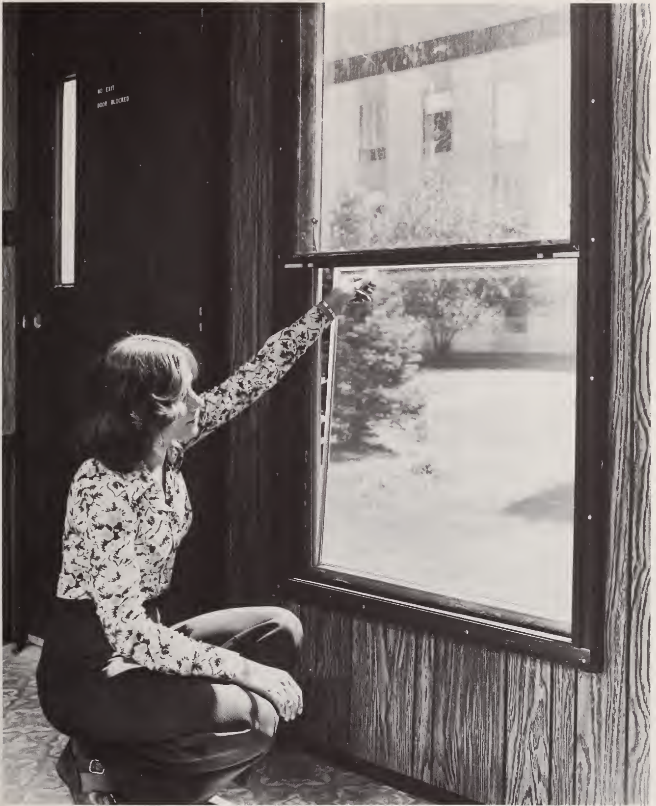
Figure 28. Egress Test. Specimen 7. Releasing screen
