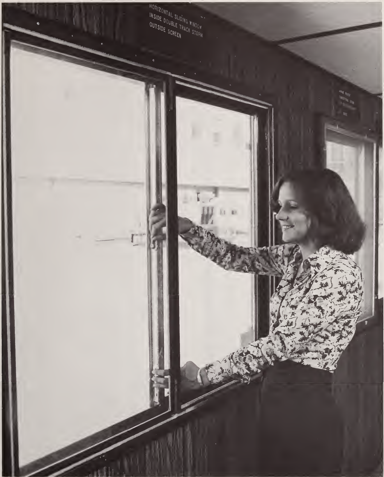
Figure 22. Egress Test. Specimen 5. Unlatching prime window Note that latch mechanism is blocked by remaining storm window.
