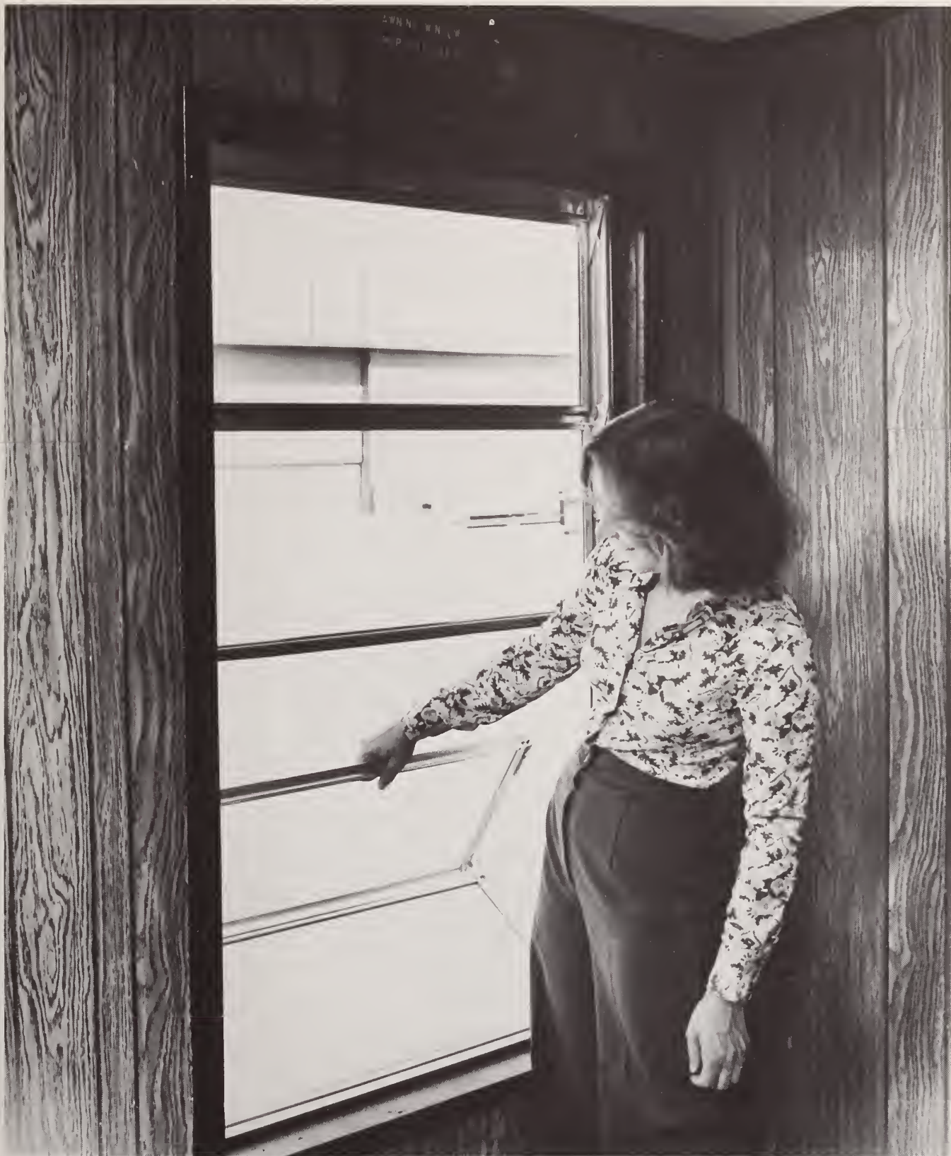
Figure 26. Egress Test. Specimen 6. Opening window When dropped, hinged window falls flat against side of mobile home.
