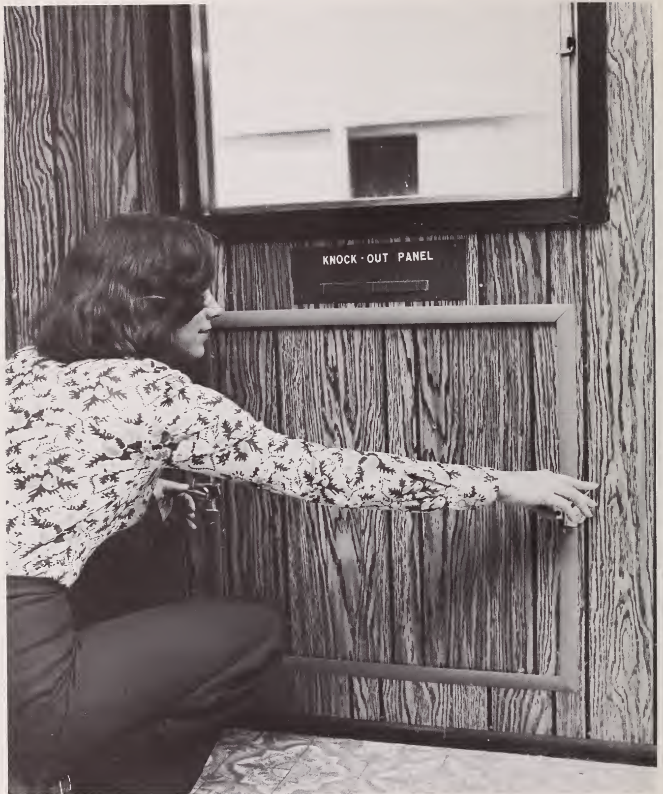
Figure 29. Egress Test. Specimen 8. Unlatching panel
