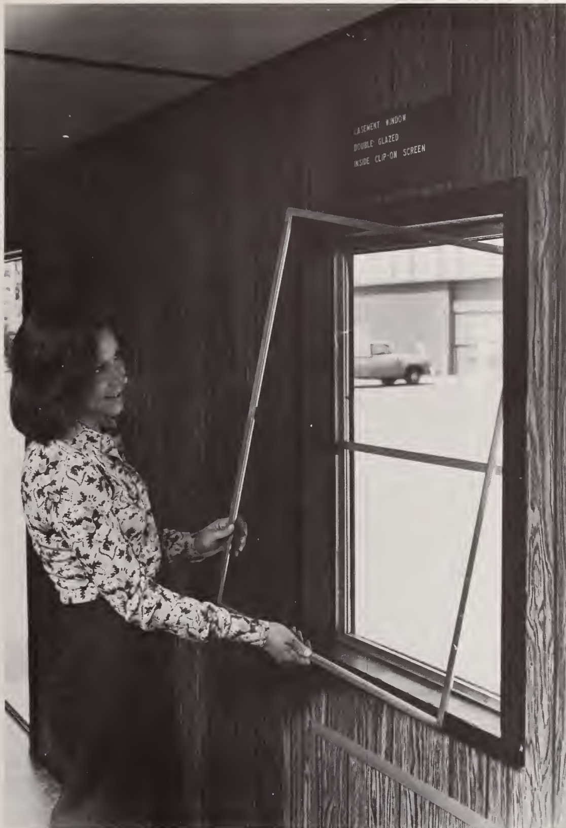
Figure 14. Egress Test. Specimen 1. Removing screen
