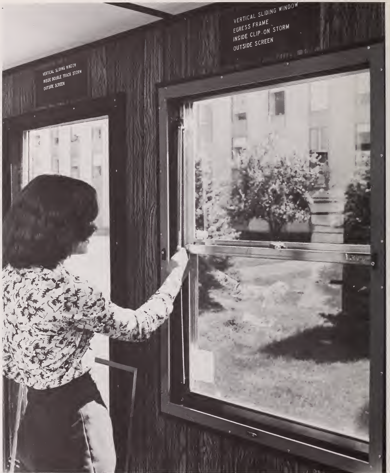
Figure 19. Egress Frame. Specimen 3. Operating egress mechanism Pulling down on vertical bar to release egress mechanism. The same procedure is used on specimen 4.
