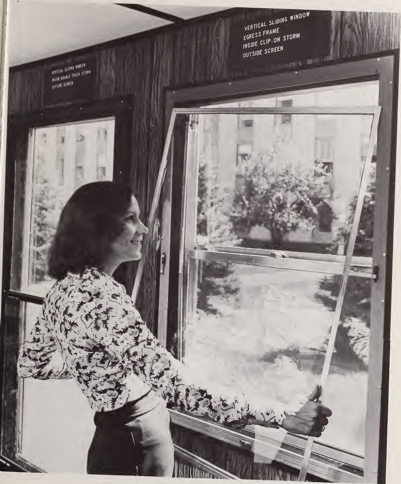
Figure 18. Egress Test. Specimen 3. Removing screen The same procedure is used on specimen 4.
