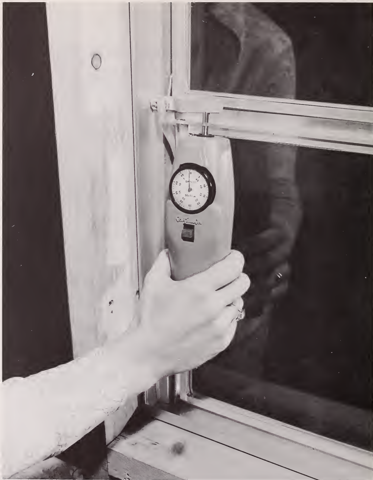
Figure 13. Use of Force Gage. Procedure used to measure force required to open window latch.
