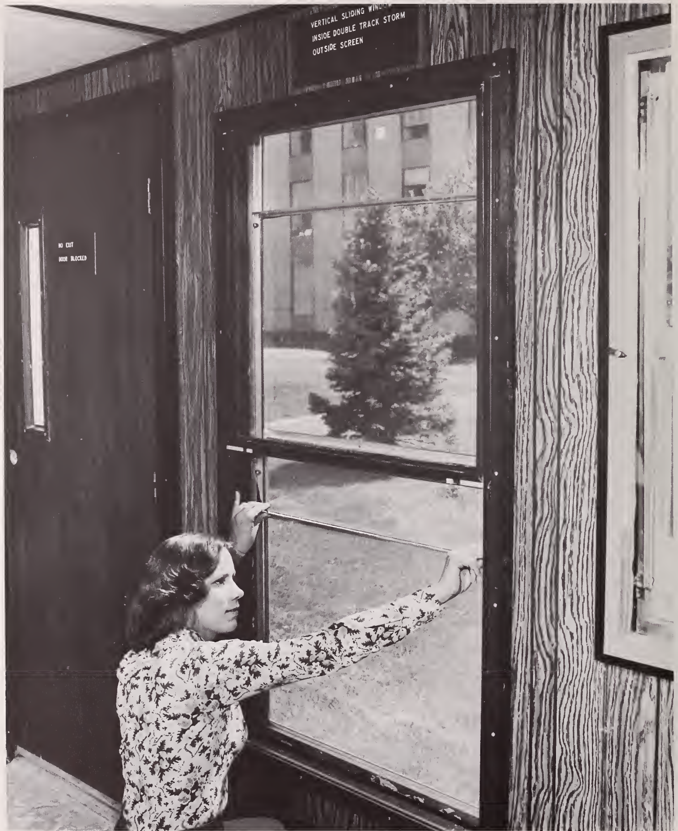
Figure 27. Egress Test. Specimen 7. Opening prime window
