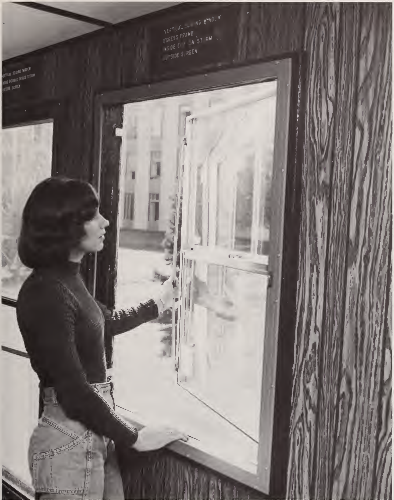
Figure 20. Egress Test. Specimen 4. Pushing window open The same egress frame is used on specimen 3.
