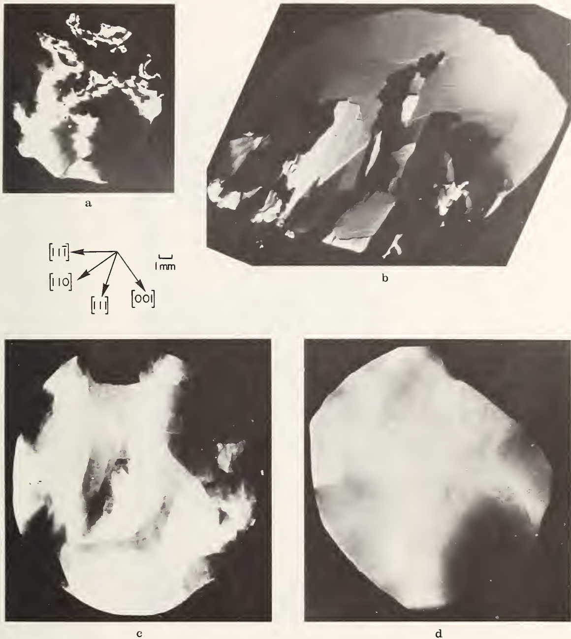
Fig. 3 ACT ( \bar{2}20 ) surface reflection topographs of nickel crystals of increasing perfection; a) grown with a [110] seed; b) grown with a [100] seed, indicating misorientation of about 100 seconds of arc; c) grown with a [111] seed under poor diameter control, indicating misorientation of about 20 seconds of arc; d) grown with a [111] seed and good diameter control, indicating absence of subgrain structure.
