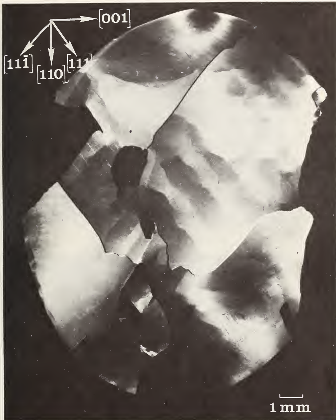
Fig. 8 ACT (\bar{2}20) surface reflection topograph of nickel crystal showing subgrain boundaries some of which are parallel to \langle 111 \rangle directions. The misorientation of these subgrains is about 300 sec.
