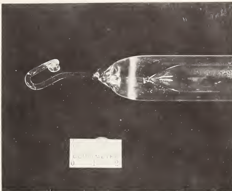
Figure 1. Modified growth tube. Annular space between growth tube and outer tube evacuated for thermal insulation. Heat flow path is 3 mm fused silica rod connecting tubes at left end.
