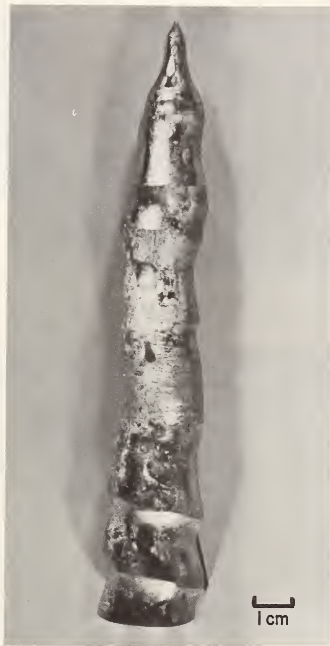
Fig. 2 Czochralski-grown Ni single crystal boule #274200 with spiral growth form. This shape is to be contrasted with the usual cylindrical growth form obtained by the Czochralski technique. Note also the small bottleneck which has been obtained near the seed material.
