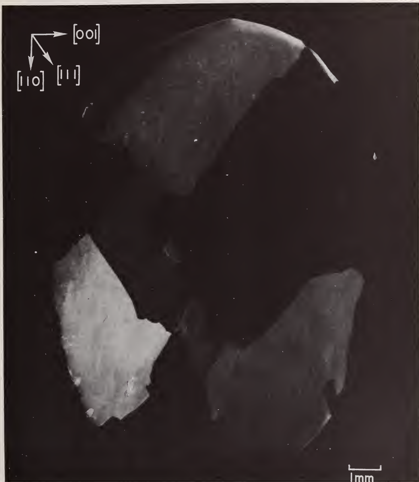
Fig. 13. ACT 2\bar{2}0 surface reflection topograph of Ni crystal #194231 grown in the \langle 001 \rangle direction.
