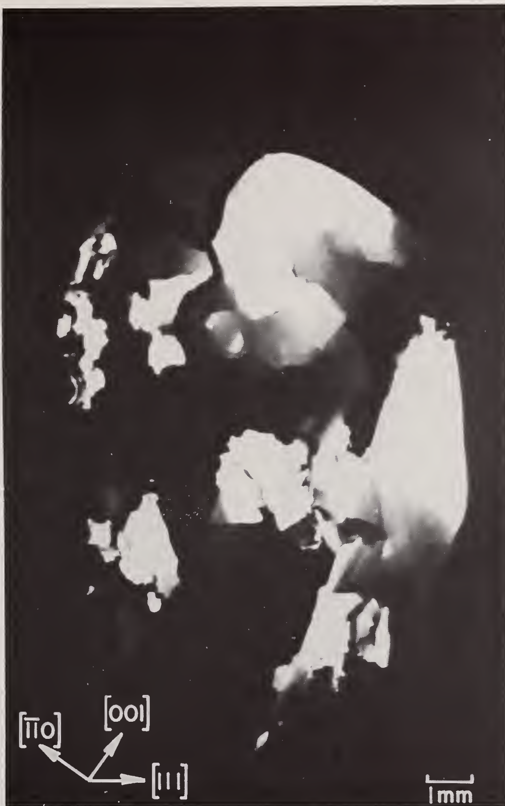
Fig. 4. ACT \bar{2}20 surface reflection topograph of as-grown Ni crystal #130221 grown with a bottleneck and with poor diameter control. Note the large sub-grains.
