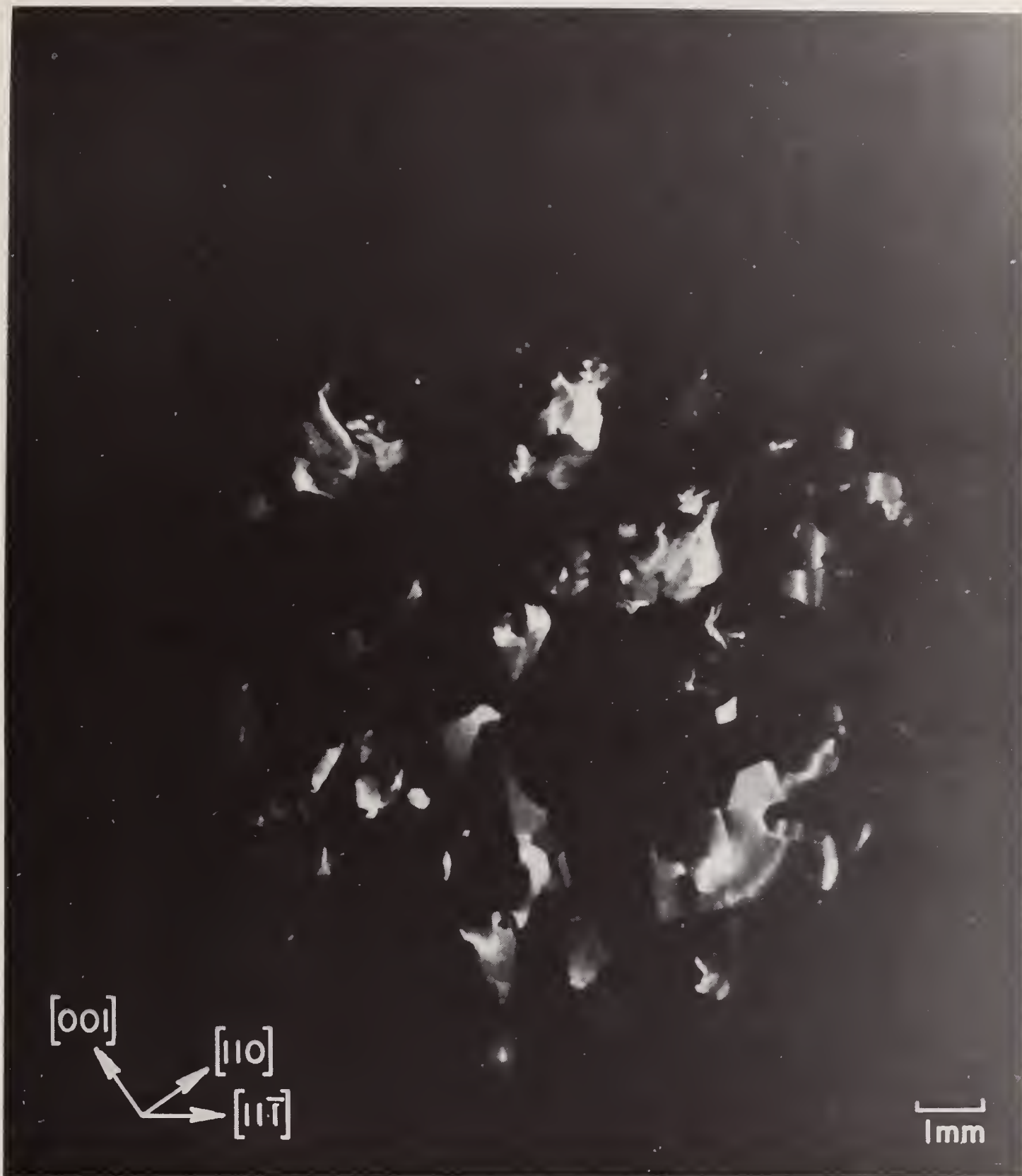
Fig. 3. ACT \bar{2}20 surface reflection topograph of a very poor quality as-grown Ni crystal (#120223) grown without a bottleneck and with poor diameter control. Note the very small subgrains.
