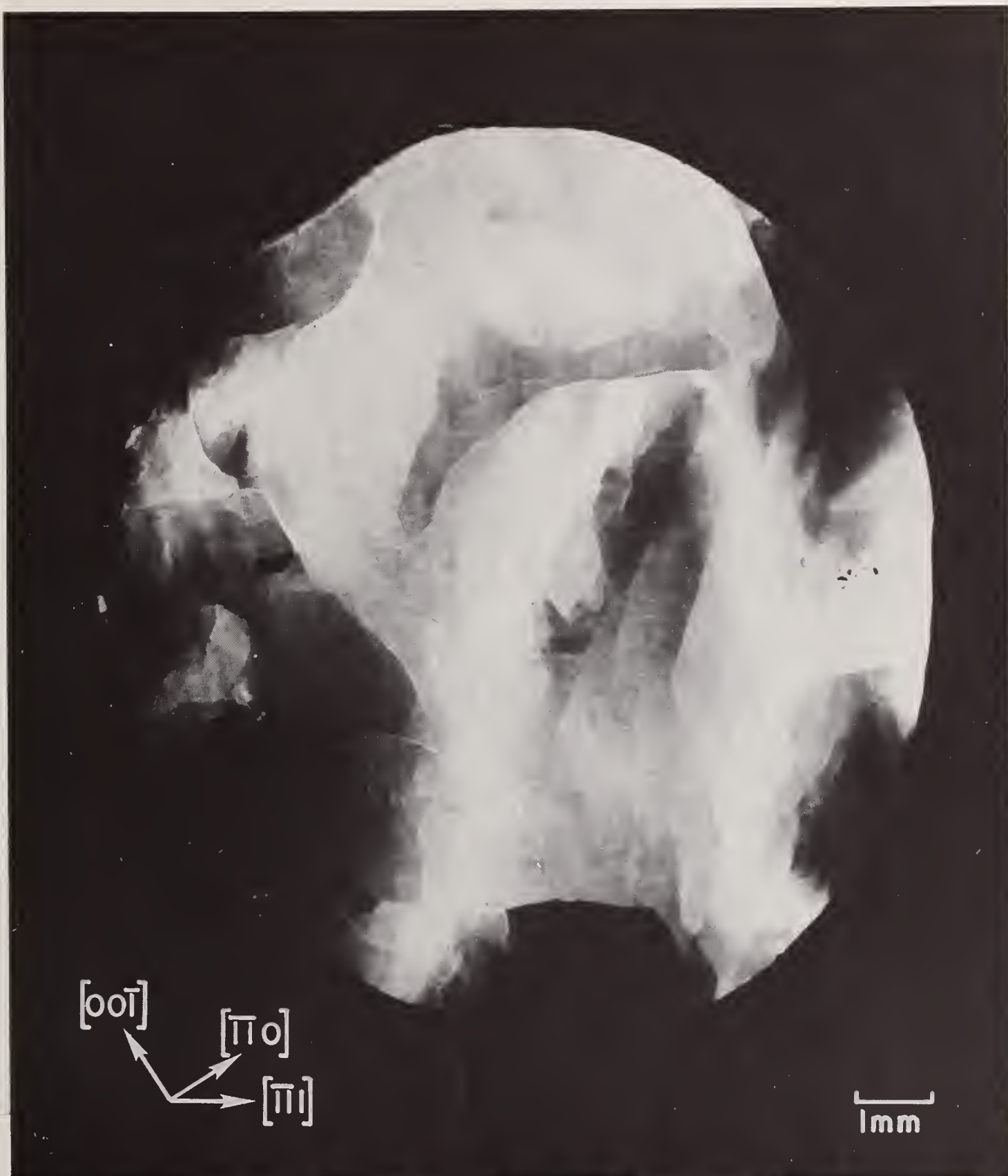
Fig. 5. ACT \bar{2}20 surface reflection topograph of as-grown Ni crystal #140231 grown with a bottleneck and good diameter control. Note that diffraction from the entire area of the crystal indicates that misorientation of sub-grains is less than 30 sec. of arc.
