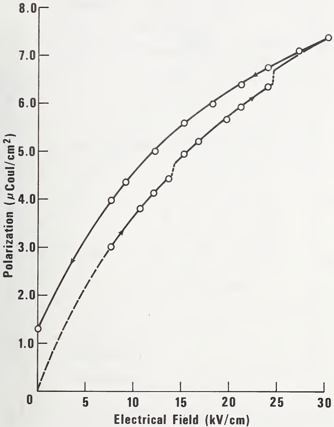
Figure 61. A partial P_t(E) hysteresis loop for \text{SrTiO}_3 ceramic ST2 (1450) over the field range 0 to +30 kV/cm. Discontinuities are due to momentary charge leakage or breakdowns.
