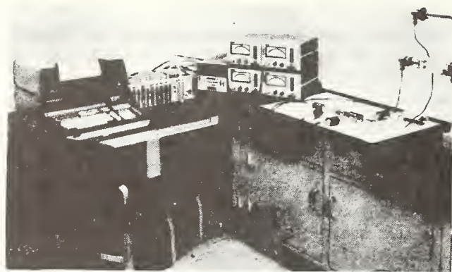
Fig. 8. Experimental six-port X-band vector voltmeter setup. From left to right: programmable calculator, input/output expander, DVM and scanner, four-power meters, six-port junction (on white paper), and two-input signal lines.
