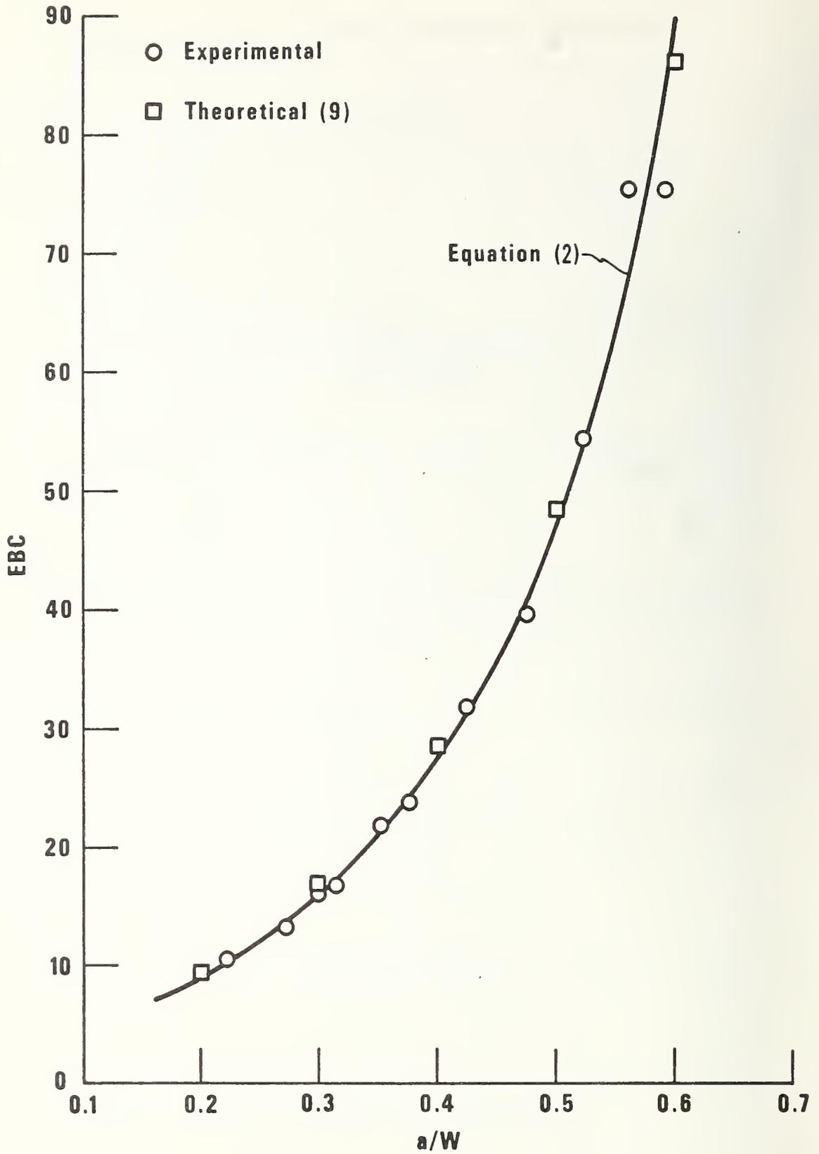
Fig. 5. Compliance calibration of the four point bend specimen.
