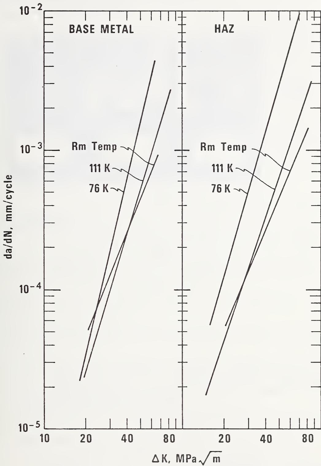
Fig. 12. Effect of temperature on the fatigue crack growth rates in 5% Ni steel weldments.
