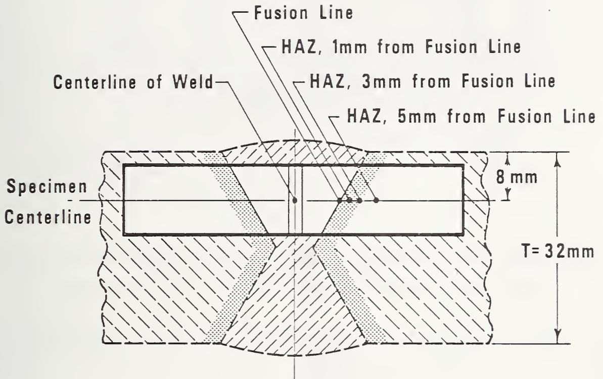
Fig. 2. Notch locations for Charpy impact specimens.
