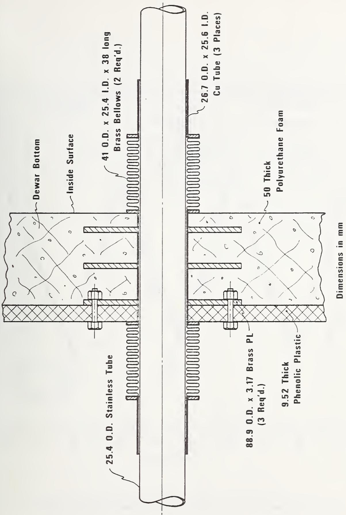
Fig. 8. Mechanical feedthrough for test dewar.
