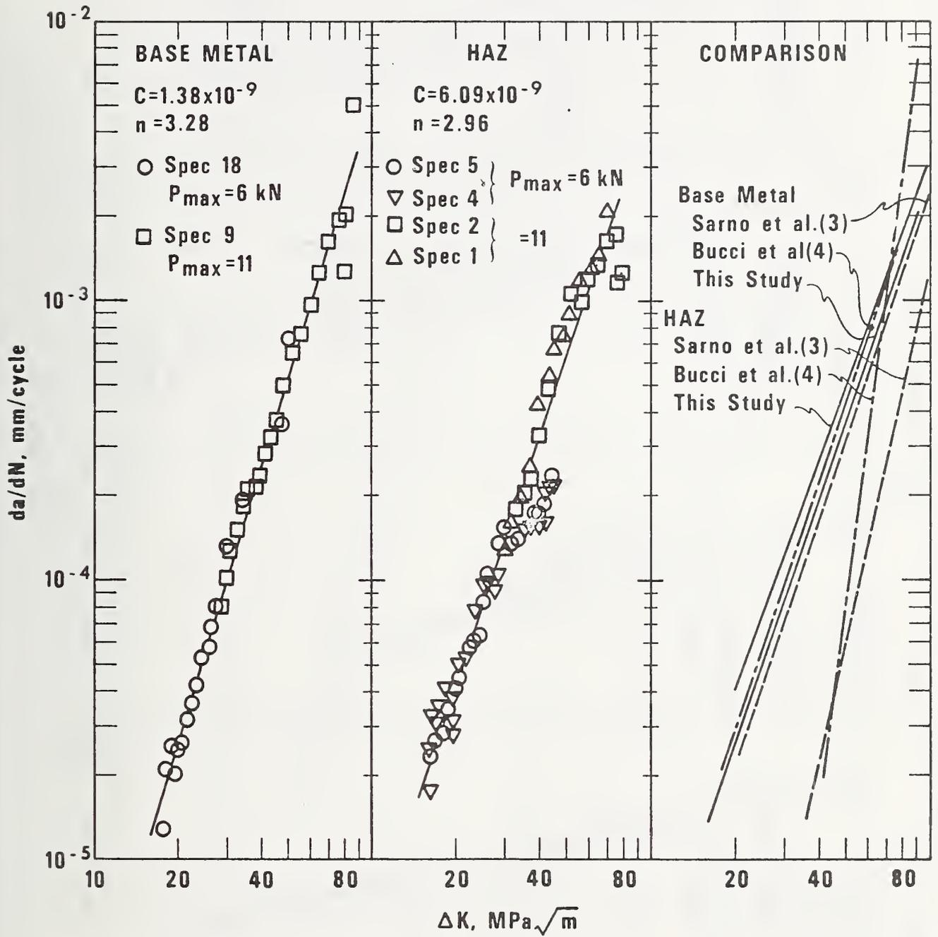
Fig. 10. Fatigue crack growth behavior of 5% Ni steel weldments at 111 K.
