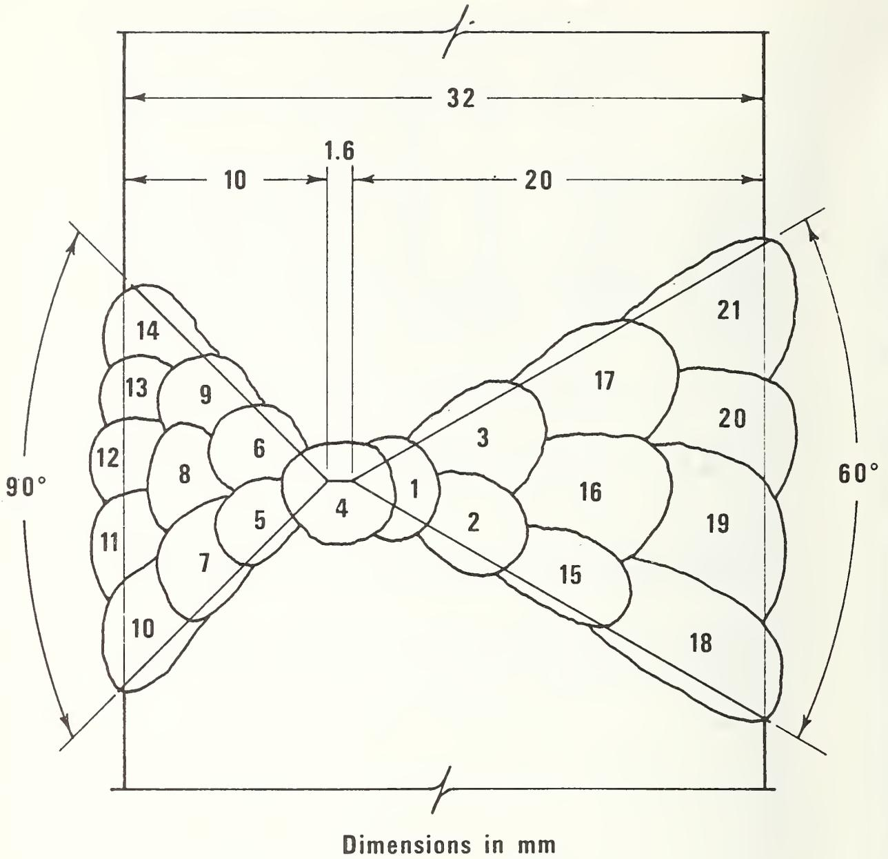
Fig. 1. Weld joint preparation and welding sequence.
