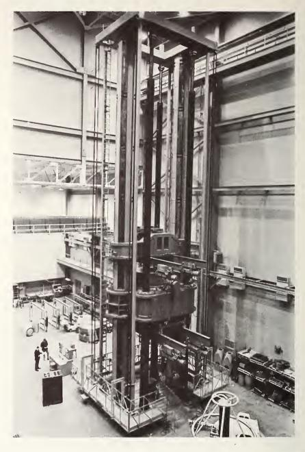
The machine can apply axial force of 12,000,000 lbf (53,400 kN) in compression 6,000,000 lbf (26,700 kN) in tension, and a transverse force of 4,000,000 lbf (17,800 kN) to a flexural member. Working space between the screw columns is 8 feet 4 inches (2.5m), and the working surface of the main platen is 8 feet 4 inches (2.5m) by 15 feet (4.6m). The reinforced concrete foundation includes
