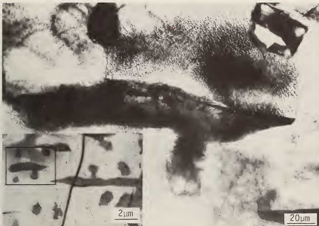
Fig. 5 A transmission electron micrograph of magnetite plates and nodules formed at the surface of a hematite crystal reduced in \text{CO}/\text{CO}_2 = 0.06 at 986^\circ\text{C} for one minute. The magnetite plates contain a high density of dislocations which anneal out rapidly during growth. The outlined area in the inset light micrograph corresponds to the area of the electron micrograph.
