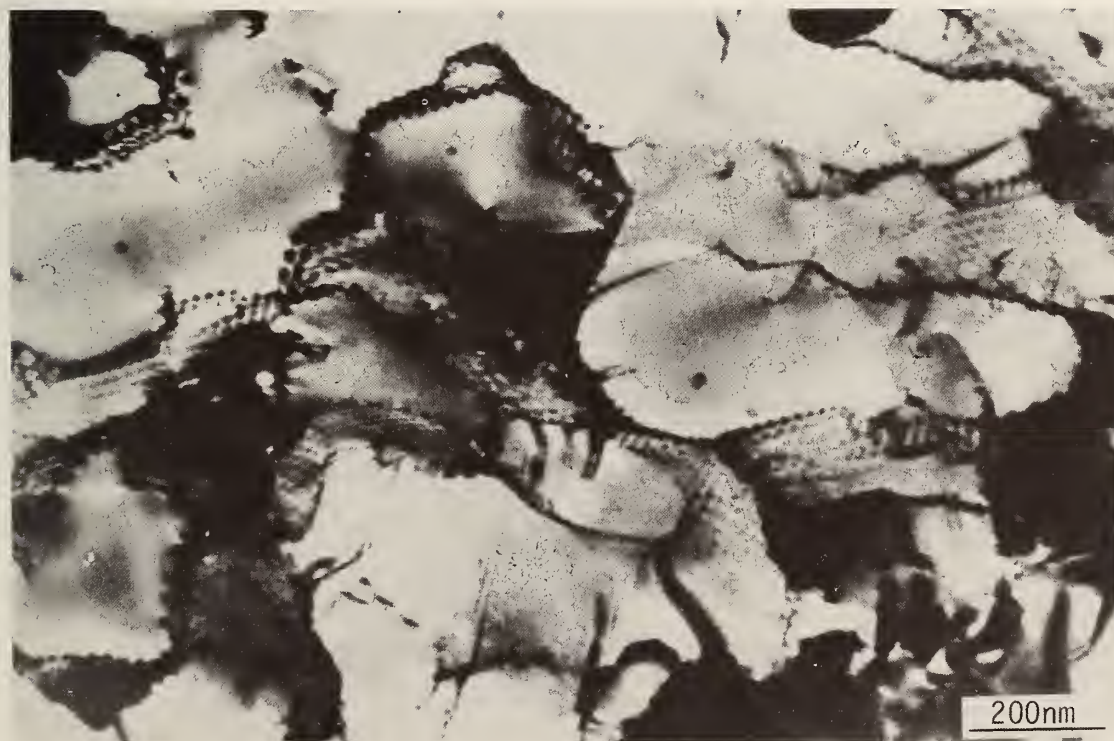
Fig. 10 Network of dislocations within a specimen fully reduced to magnetite at 1000^\circ\text{C} . These networks form by a recovery process at temperatures after the reduction has occurred.
