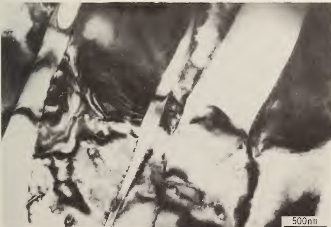
Fig. 4 A typical electron micrograph of the "high" temperature reduction morphology in a hematite crystal partially reduced to magnetite in CO/CO 2 = 0.125 for one minute at 1000°C. The magnetite crystals are in the form of lenticular plates and do not contain the tunnel structure observed at lower temperatures.
