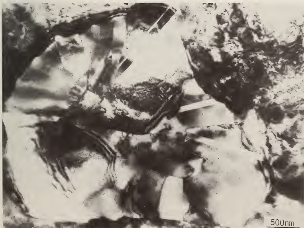
Fig. 6 A high magnification view of a single magnetite nodule showing its twinned internal substructure.
