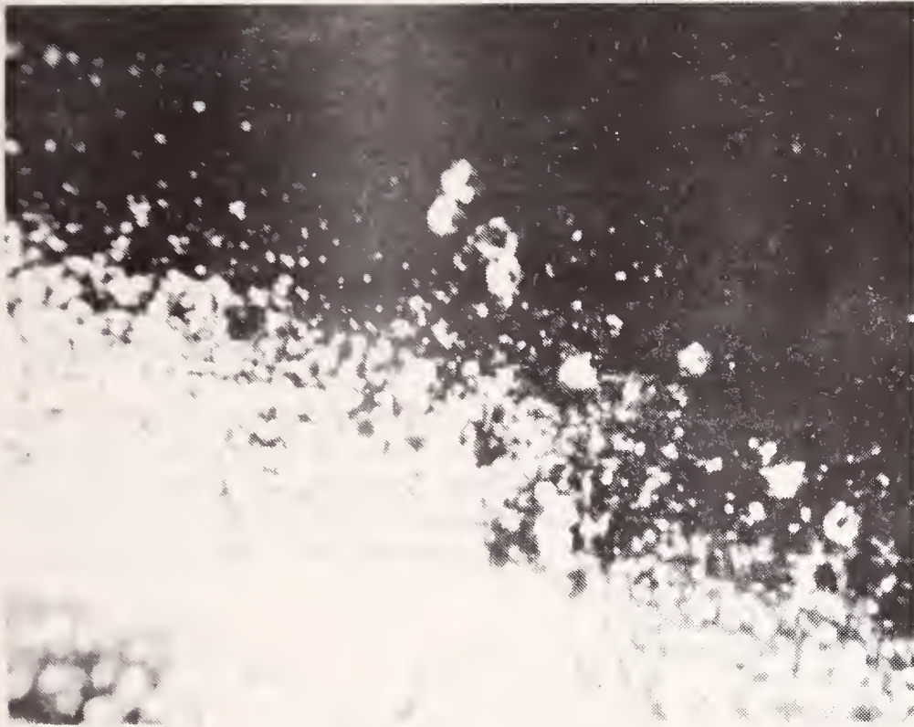
Figure 19. A field of small pits observed on transducer MILES 96R-1 at Griffis Air Force Base. Pit diameters are approximately 0.04 to 0.09 mm ( 1.5 to 3.4 \times 10^{-3} in).
