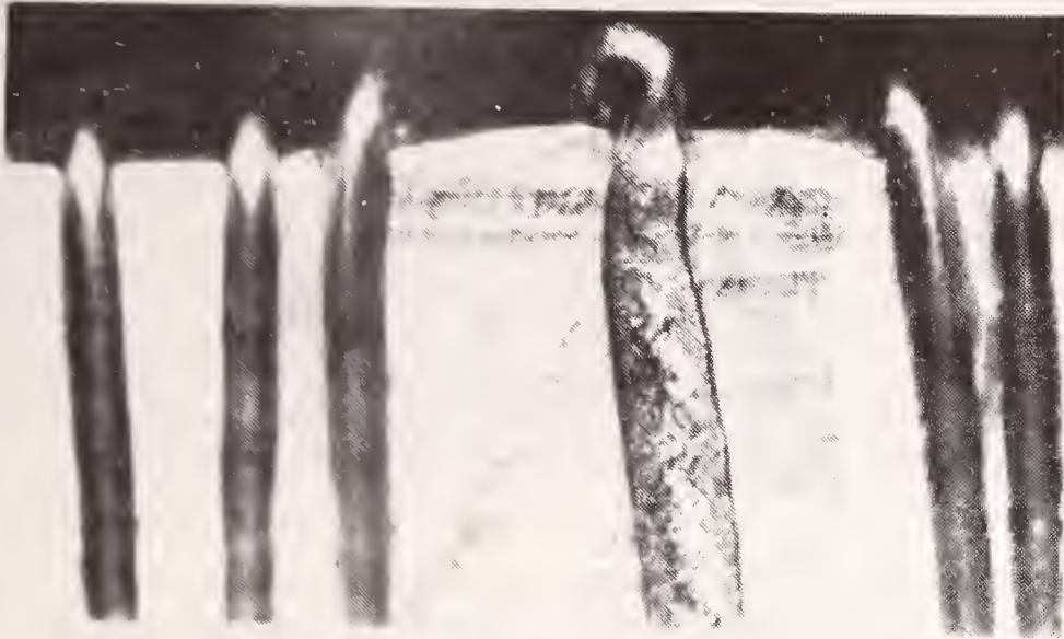
Figure 17. Smashed sense coil for flat transducer specimen No. 71 after an exposure of 100 hours at a 2043-lbf load.
