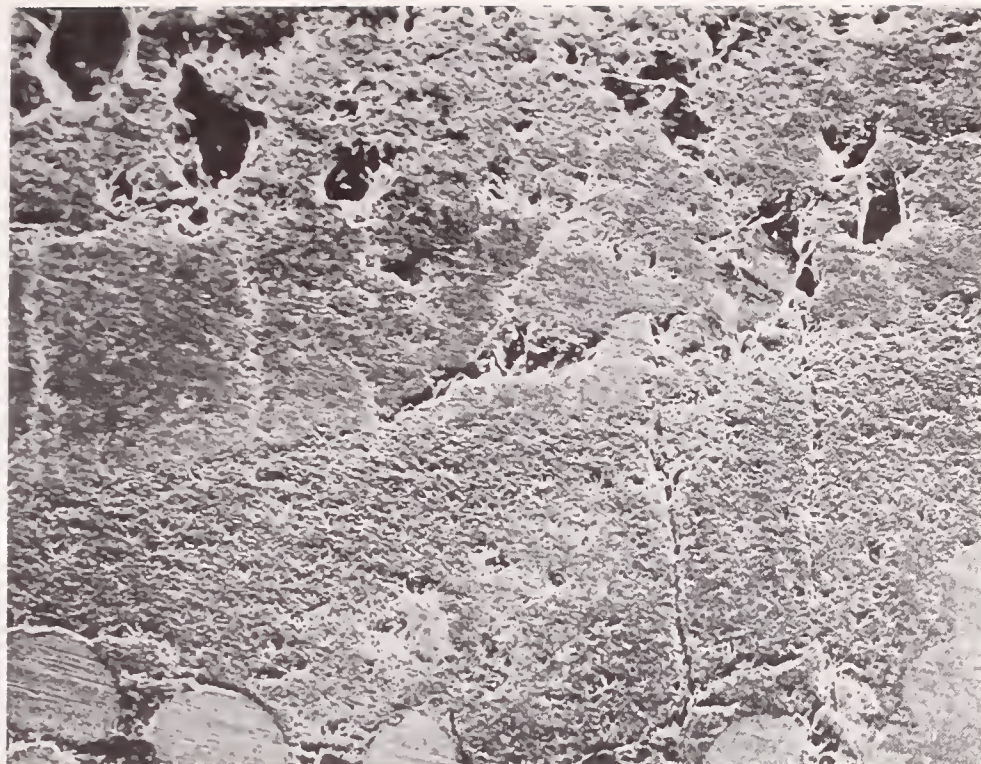
Fig. 20a. Anode (100X) consisting of metal alloy mesh (bottom), the remains of a conducting spinel layer (see text) and slag (top).
