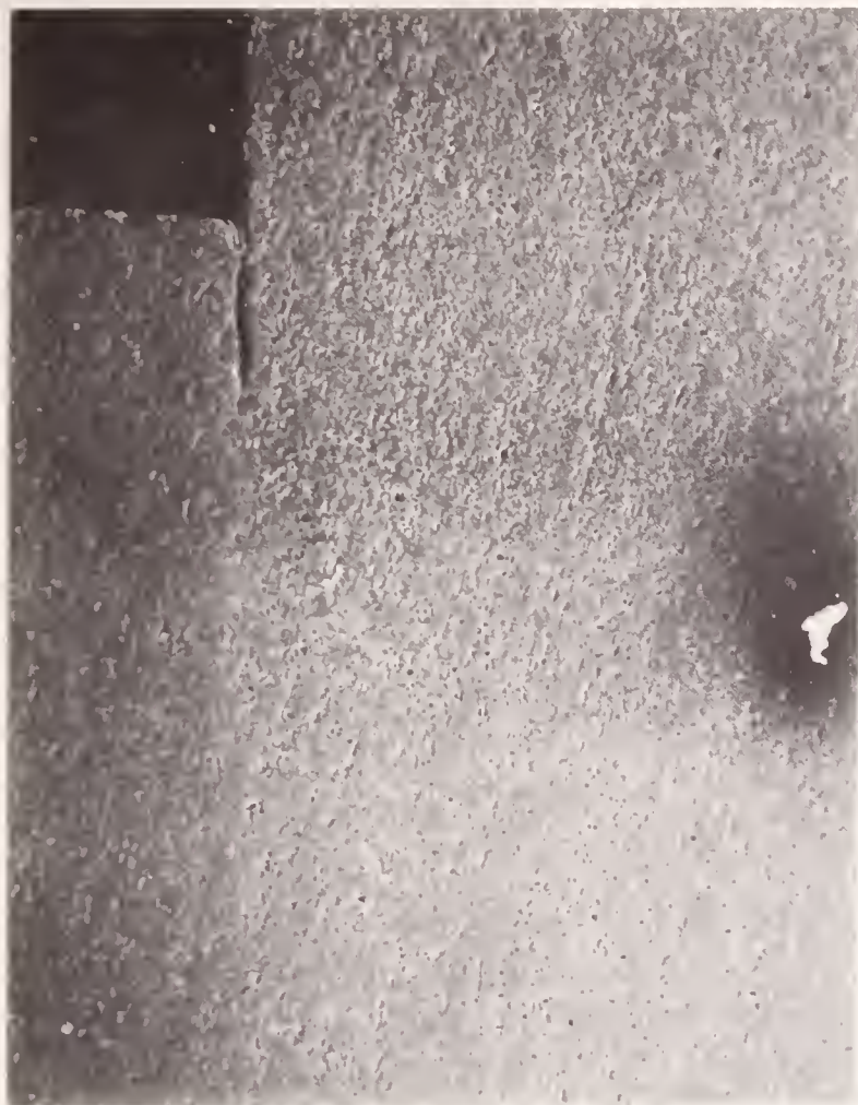
Fig. 14a. 50X secondary electron micrograph showing the \text{MgAl}_2\text{O}_4 insulator on left and iron \text{MgAl}_2\text{O}_4 on the right.
