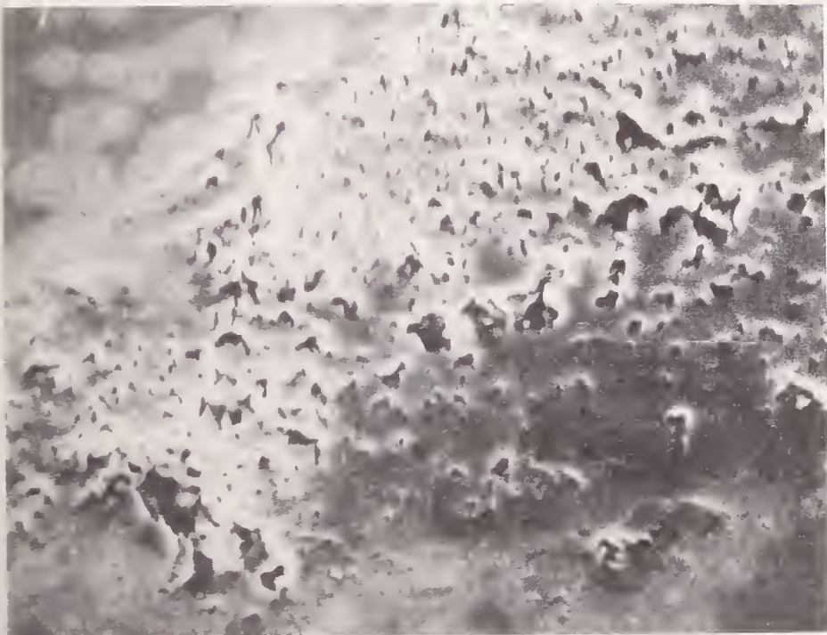
Fig. 25. Typical K/Si-rich domain (1000X) in Fe/Al-spinel prepared by MIT.
