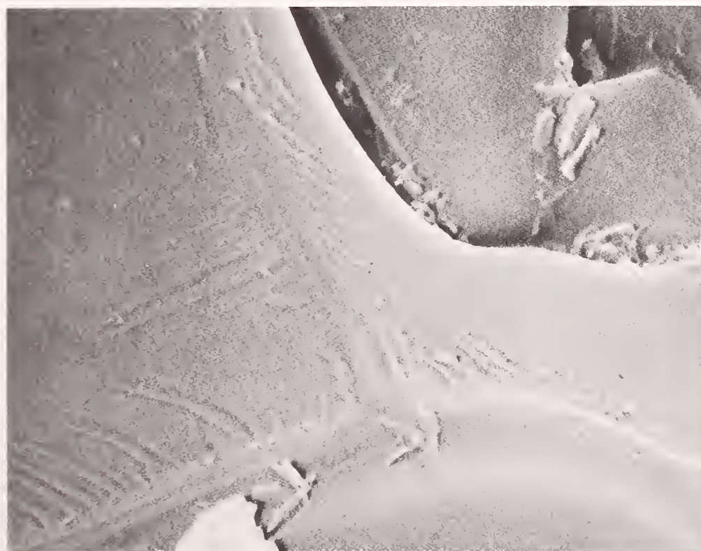
Figure 11b. Enlargement (20,000X, 20KV) of grain boundary in Fig. 11a. showing no evidence for intergranular melt, in contrast to Fig. 10b.
