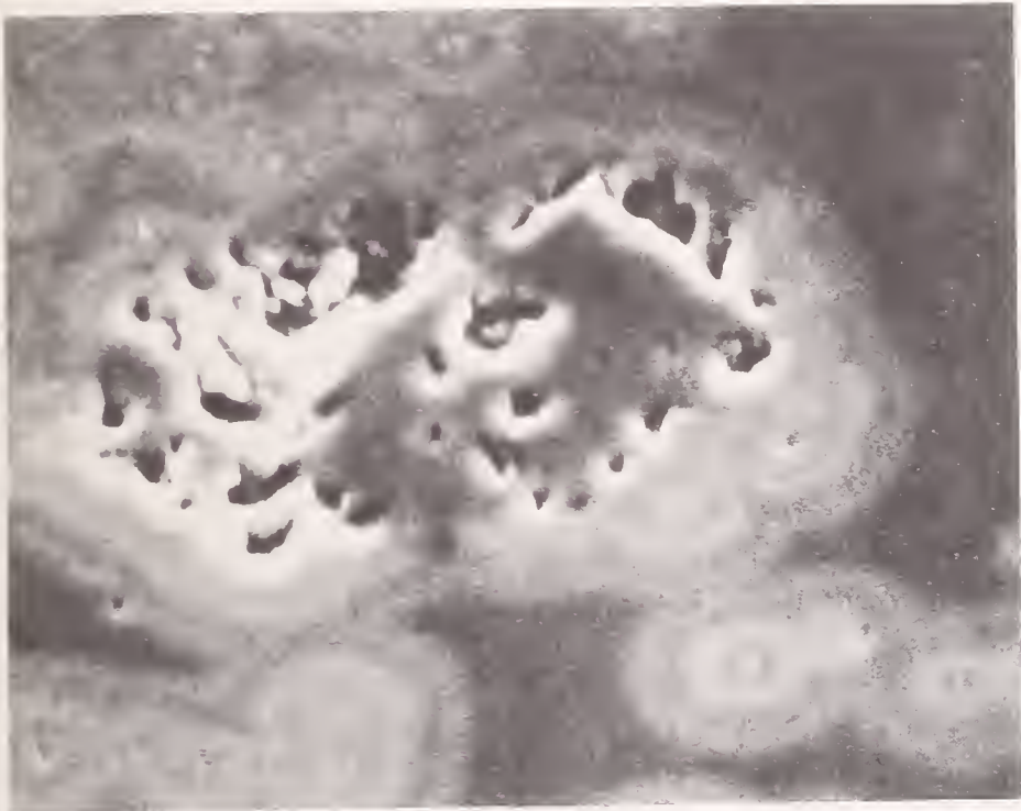
Fig. 24. Typical Mg/Al-rich domain (2000X) in Fe/Al-spinel prepared by MIT.
